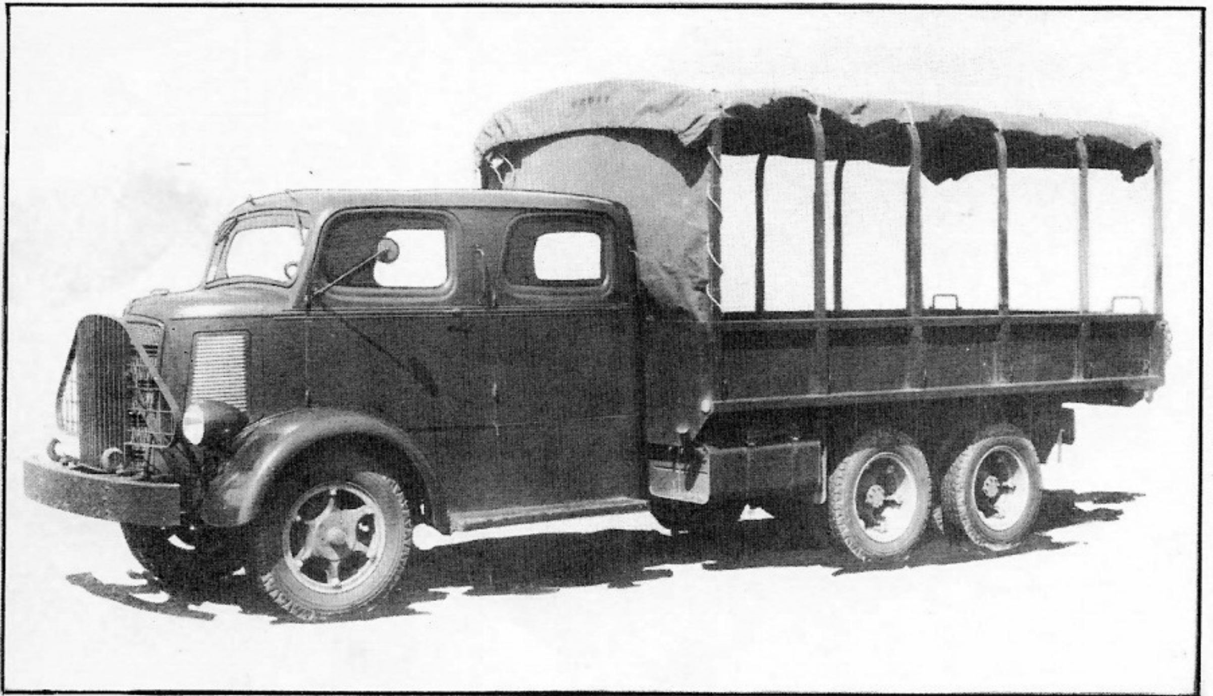
One of the new 2½ ton (6 x 4) cab over engine Mack trucks recently acquired by the Army. The double cab is of particular interest. The front of the cab holds the driver and assistant driver, and the rear of the cab holds a supplementary crew of three.
