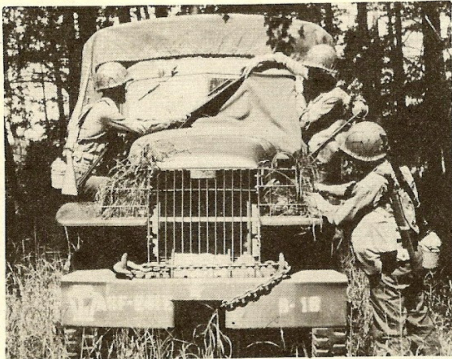
Fig. 5—Dousing windshield shine with canvas and headlight shine with leaves. Mud or grease will do the job, too, but they're messier.
