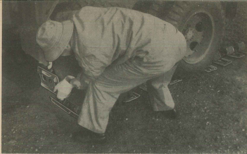
Figure 5. Joe tilts up the first few track shoes and holds them firm against the tire. When he's all set—feet away from the track—he yells, "Gung ho!" and the driver backs up some more . . . slow.
