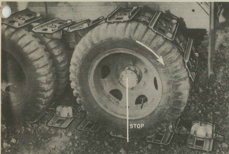
Figure 8. This is what your truck looks like if you've lagged along through the first photos. The truck is stopped right here, so only TWO shoes are left sticking out from under the tire.
