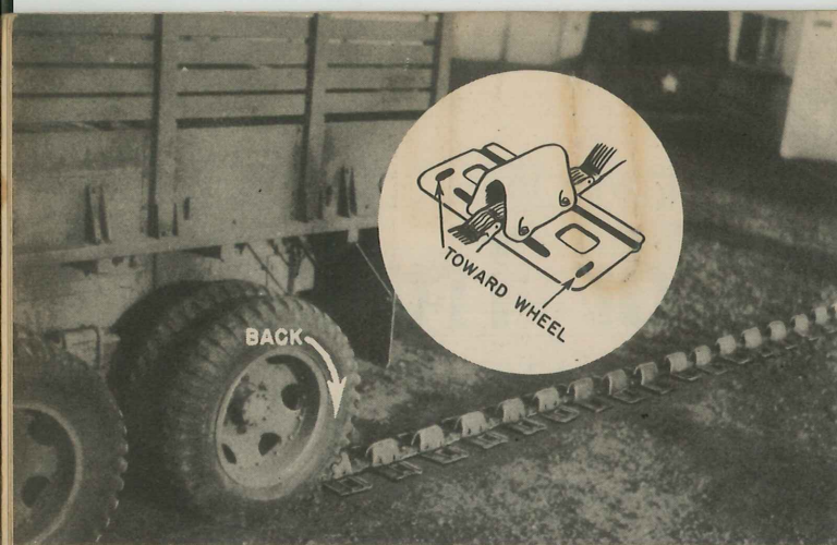
Figure 3. Two bruisers just dragged the track around back of the truck. Place the track so the edge of the shoe with the SHORT CLEATS FACES the tire; the edge with the LONG cleat faces AWAY from the tire.
