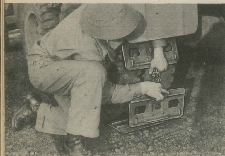
Figure 9. See what happens to the last two shoes . . . they get hitched. Be sure the hook end sits down around the connection bolt, and the yoke end up around the pin. Tighten the connection bolt.
