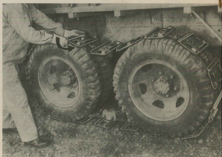
Figure 10. Mark the shoe you start on, and go around the track giving each adjusting screw 10 or 15 turns. Keep it up till the slack's taken out of the track. Three adjusting wrenches come with each set.
