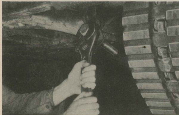
Fig. 6. Adjust the idler shackle stop bolt to a clearance of 1 3/4 inches to 2 inches between the end of the bolt and idler shackle.
