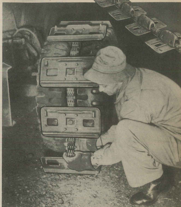
Figure 12 (upper photo) Nothing's special about slipping the track on the front tires. First put on the spare wheel. That's easy . . . just drive the front wheel up on a board. That's to get clearance enough to put on the spare wheel. Stretch the tracks out in front, and hop to it. (Lower photo) The same system used in Figure 5, but with the truck moving FORWARD, brought the track around to here. Now Joe's joining up the last shoe on the ground. Next he'll tighten each shoe (as in Figure 10), till the track's snug.
