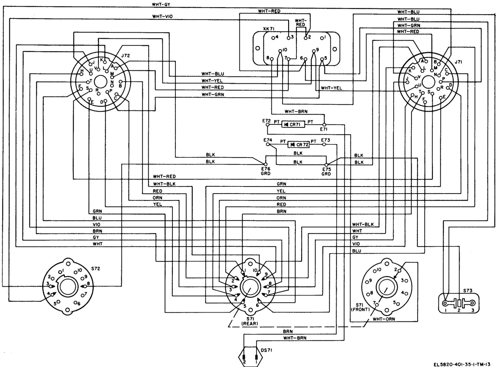
Figure 2-3. Control, Frequency Selector C-2742/VRC, wiring diagram.
