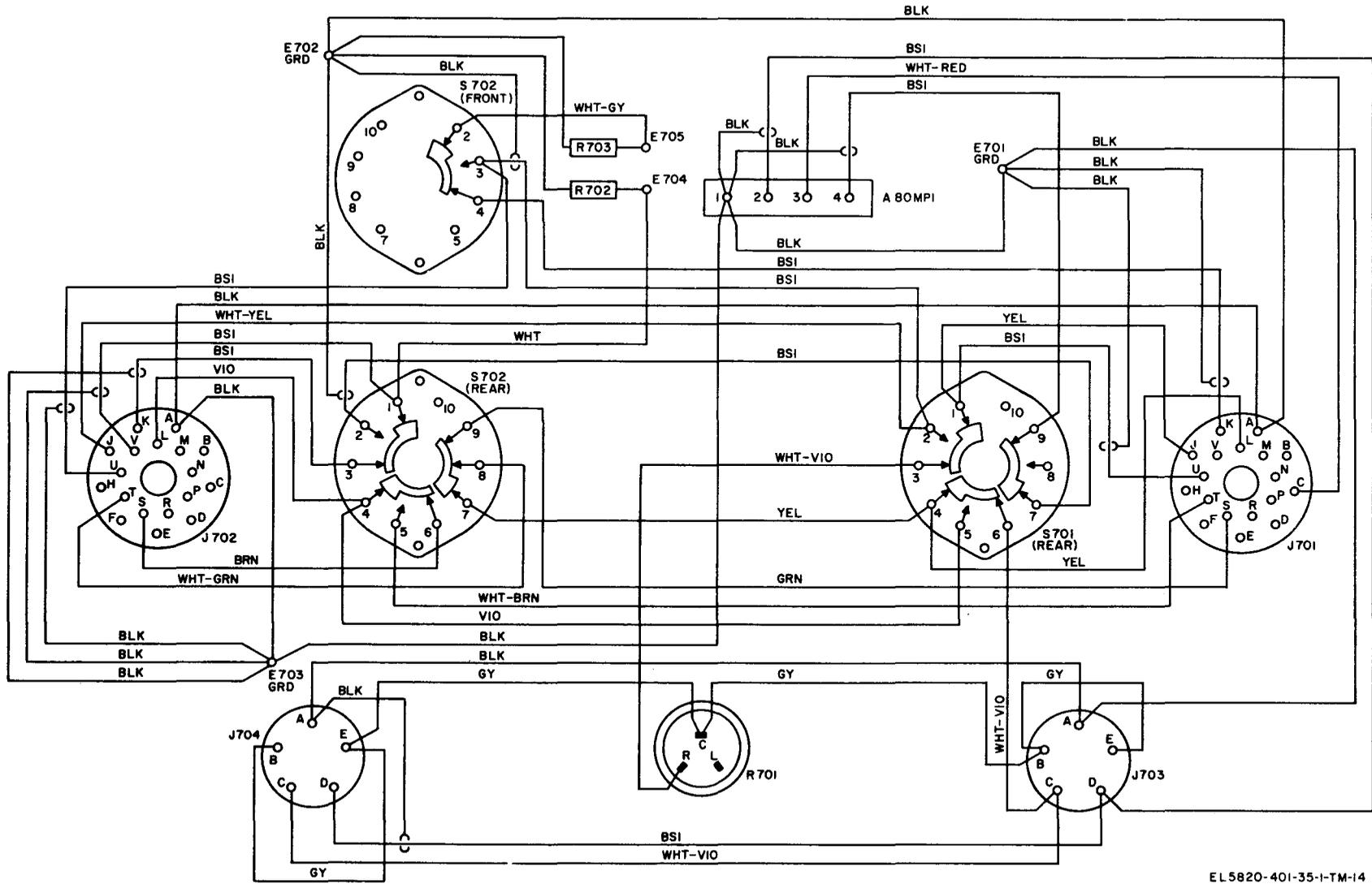
Figure 3-3. Control, Radio Set C-2299/VRC, wiring diagram.
