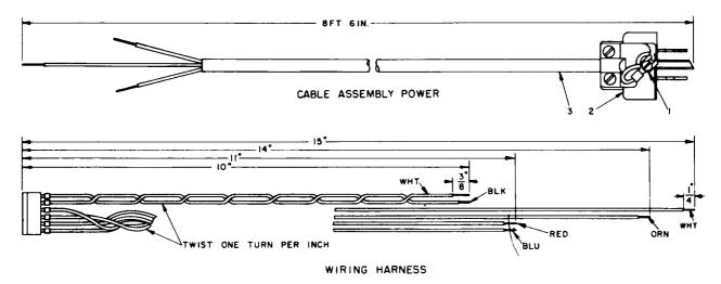
If repair is not practicable, replace power cable assembly and wiring harness.
