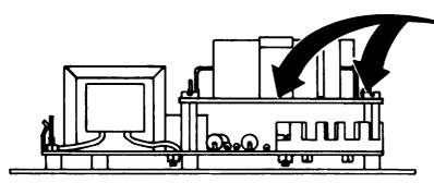
Disconnect pins A through D of power supply board from nylon connector of amplifier circuit board assembly.
