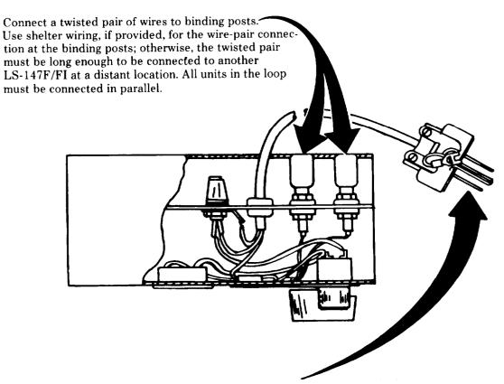
Connect the plug of the power cable assembly to a 115-volt, 60-Hertz (Hz) power source.
