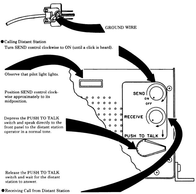
Adjust the RECEIVE control to obtain desired volume level.
