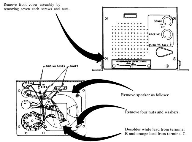
Replace defective speaker with one that is serviceable as follows:
