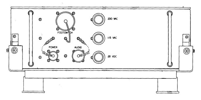
FIGURE 3-2 CONNECTORS - REAR VIEW
