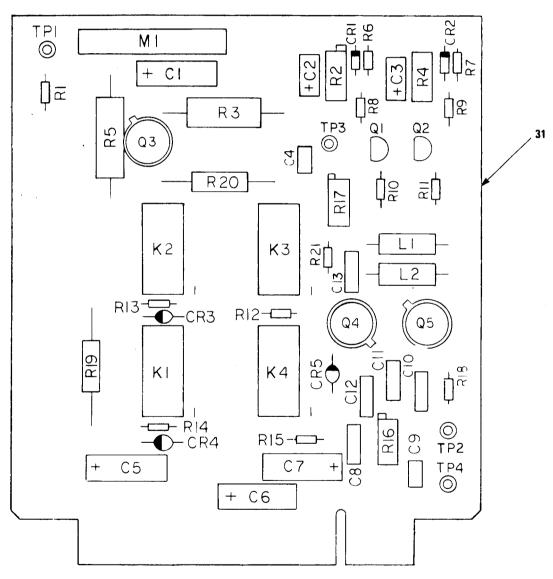
Figure C-13. Bias Oscillator and Meter Drivers Assembly
