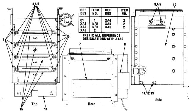
Figure C-18. Circuit Card Housing Assembly
