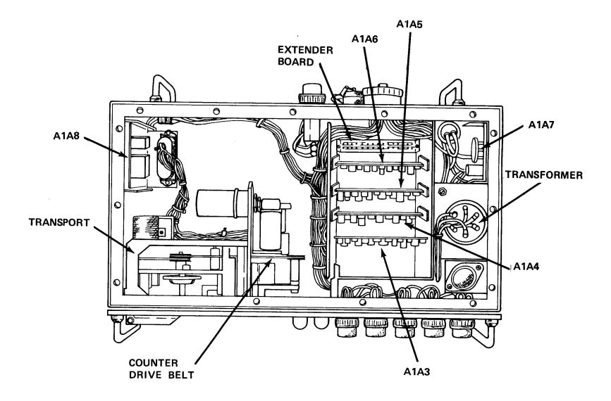
**FIGURE 7-1**AN/UNH-17A - TOP VIEW
