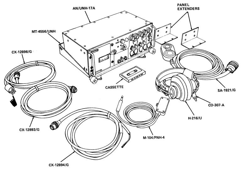
Figure 1-1. Sound Recorder-Reproducer Set AN/UNH-17A
