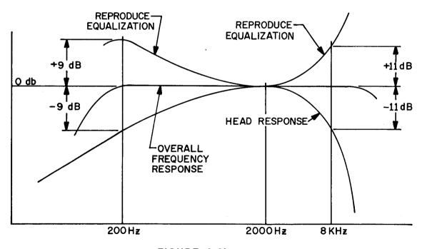
FIGURE 6-2b EQUALIZATION CURVE AT 1 7/8 IPS
