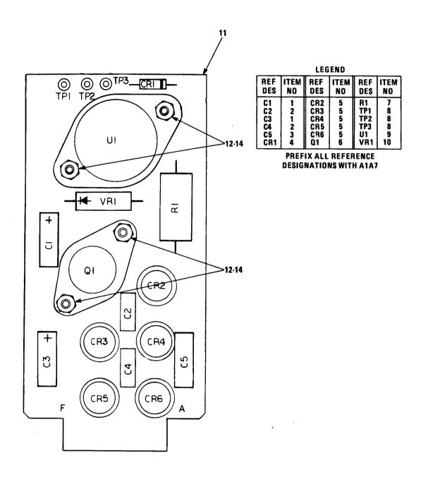
Figure C-16. Power Supply Assembly
