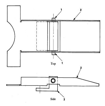
Figure C-4. Brake Subassembly
