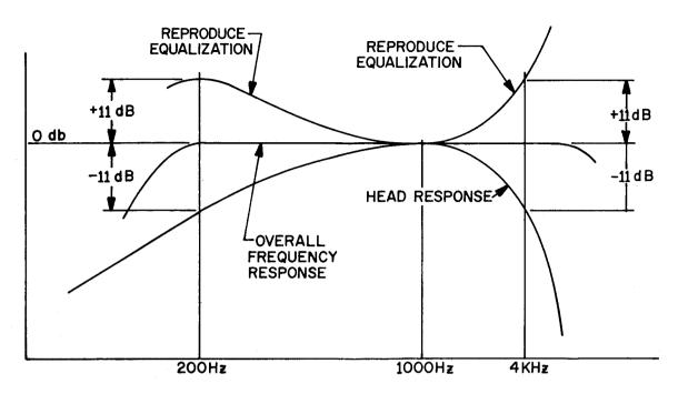
FIGURE 6-2a EQUALIZATION CURVE AT 15/16 IPS
