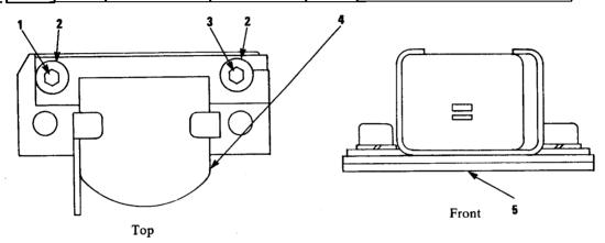
Figure C-7. Head Mounting Assembly
