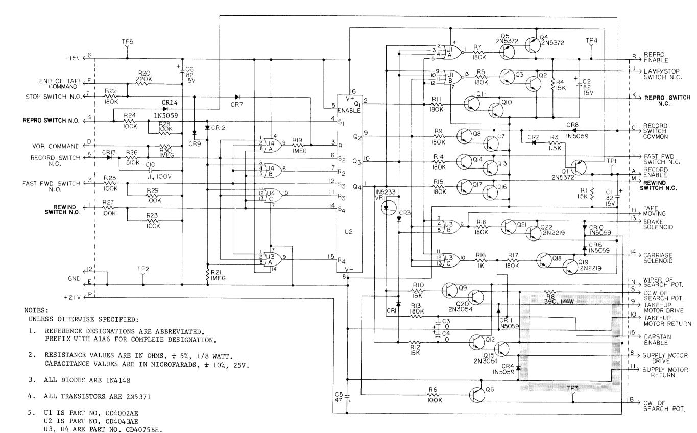
FIGURE 8-10 SCHEMATIC DIAGRAM LOGIC CONTROL ASSEMBLY
