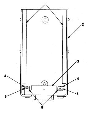
Figure C-19. Card Guide Bracket Assembly
