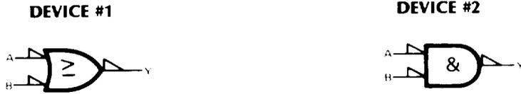
8-69. **MIXED LOGIC.** The use of the polarity indicator symbol (  $\blacktriangleleft$  ) automatically invokes a mixed-logic convention. That is, positive logic is used at the inputs and outputs that do not have polarity indicators, negative logic is used at the inputs and outputs that have polarity indicators.
