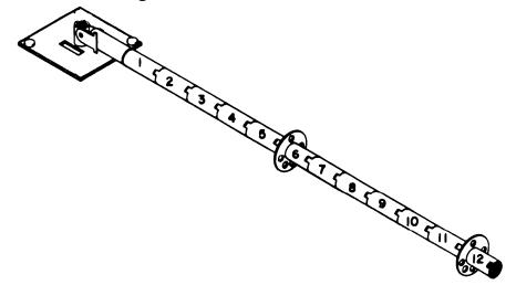
STEP (13) Turn both the UPPER and LOWER GUY PLATES so that one hole is uppermost:
