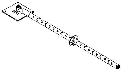
STEP Slide the UPPER GUY PLATE (color code RED) onto the male end of the UPPER ADAPTER ASSEMBLY.
