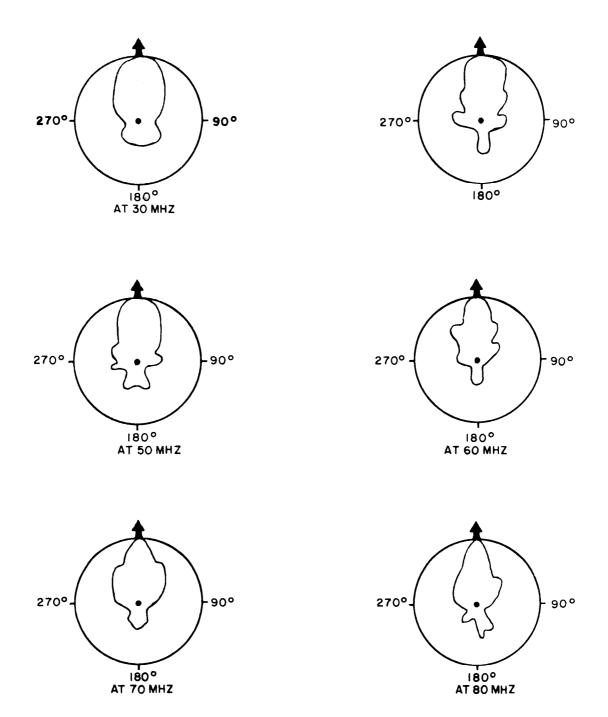
The LOW ANGLE VERTICAL RADIATION CHARACTERISTICS and the UNIDIRECTIONAL HORIZONTAL RADIATION CHARACTERISTICS make this an excellent antenna for field use.
