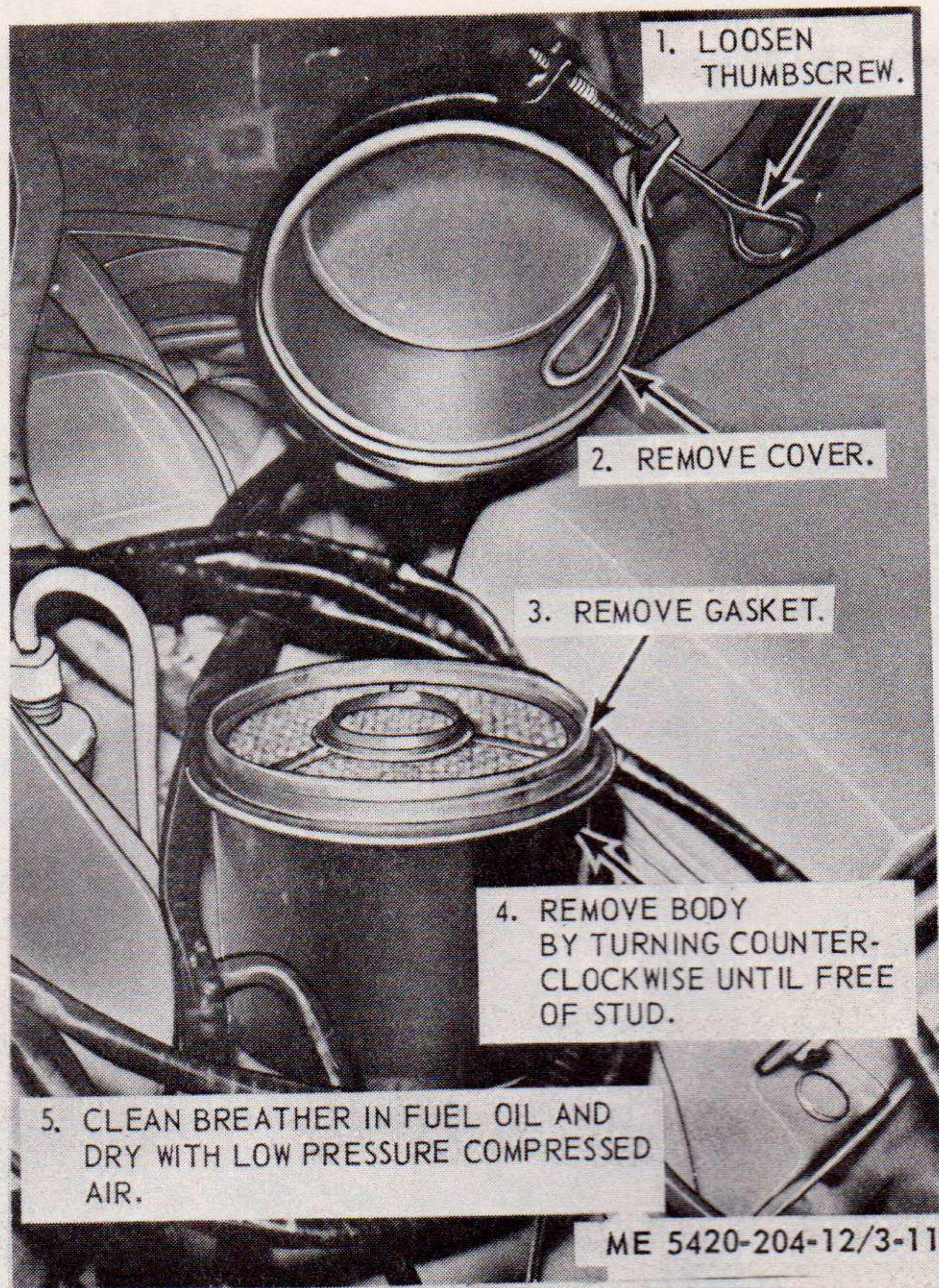
Figure 3-11. Engine crankcase breather service.
