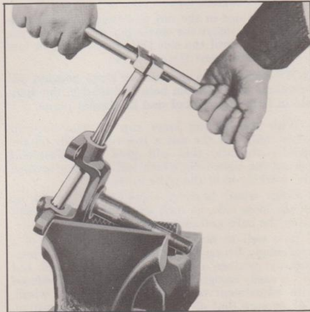
Fig. 11—Reaming Steering Knuckle Bushings
