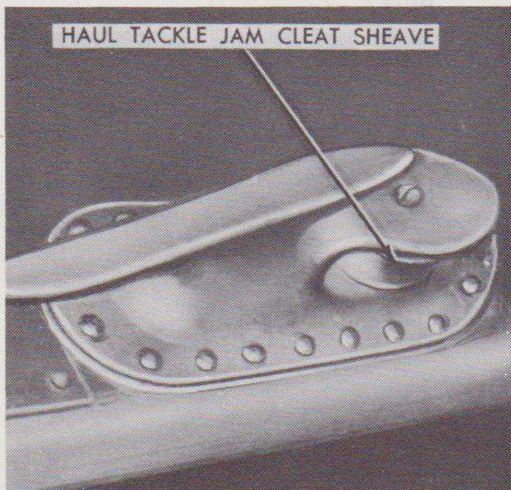
3 Haul tackle jam cleat sheave. (Clean sheave and lubricate sparingly)
