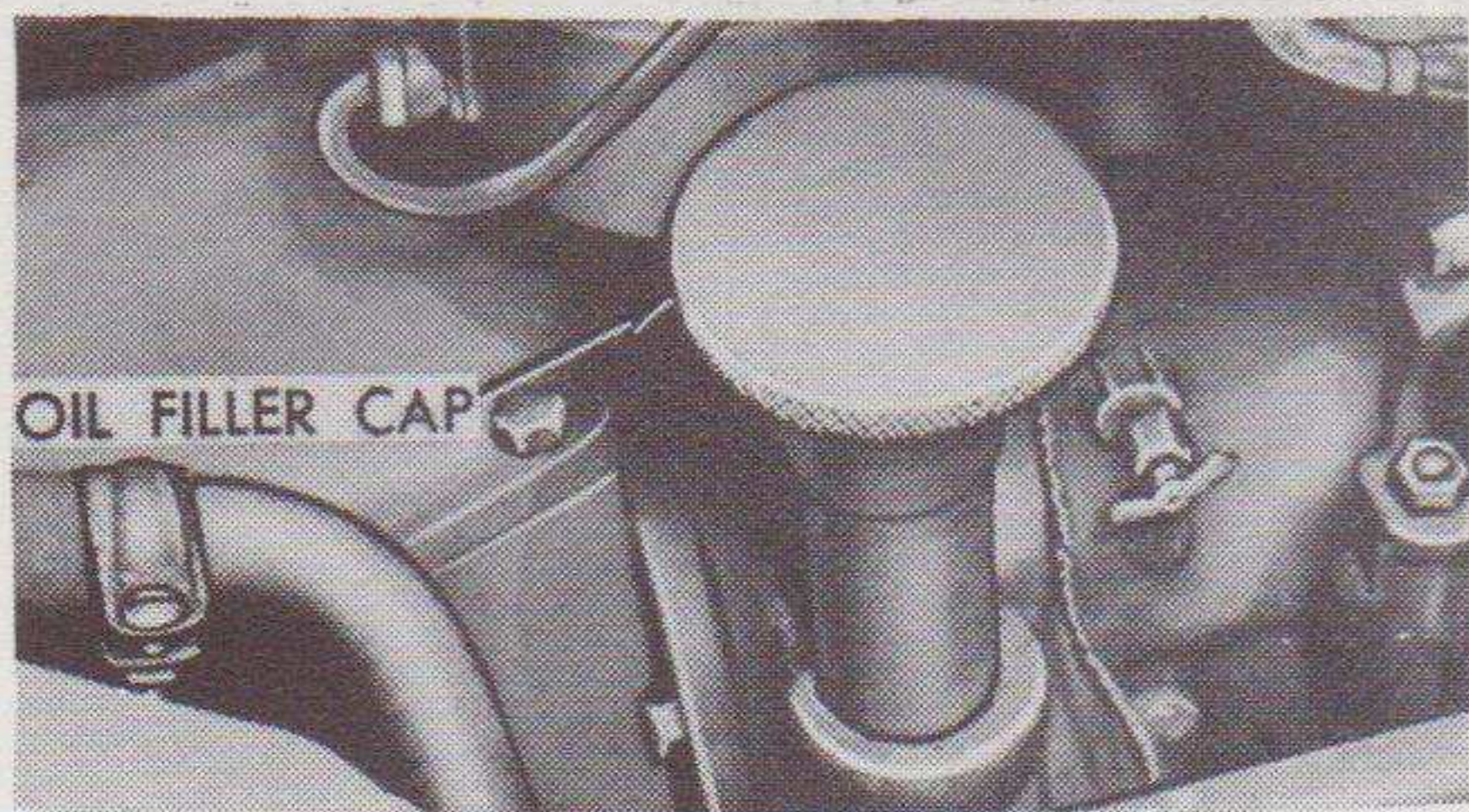
17 Oil filler. (Add oil only when boat is unloaded and in water)
