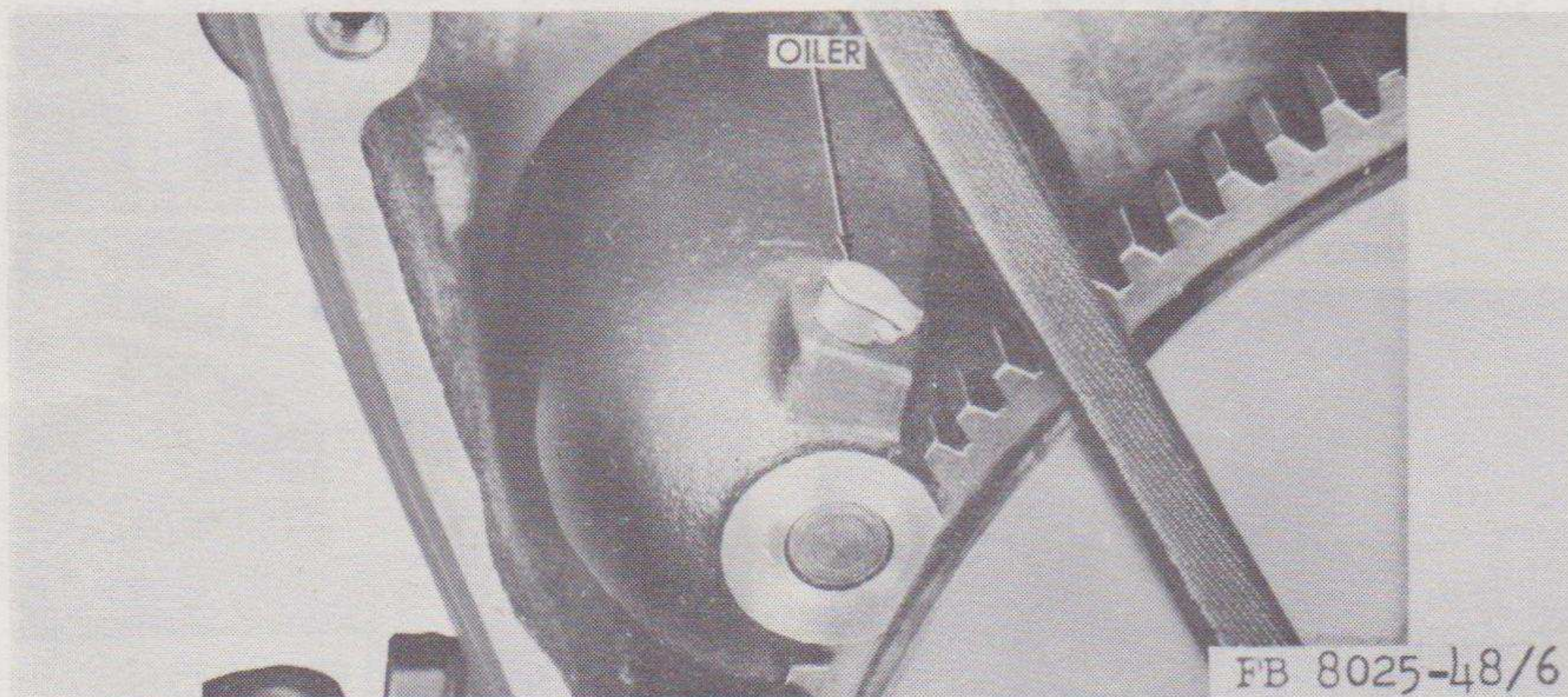
23 Starter drive housing bushing. (Clean fitting and lubricate sparingly)
