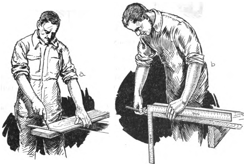
FIG. 1.—Using steel square.
