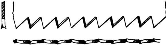
FIG. 3.—Teeth of crosscut saw.
