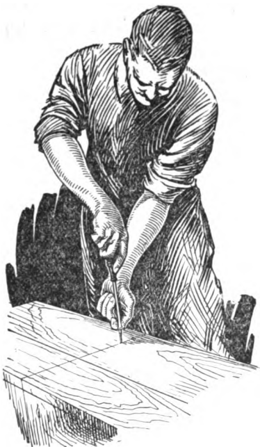
FIG. 13.—Fastening with screws.
