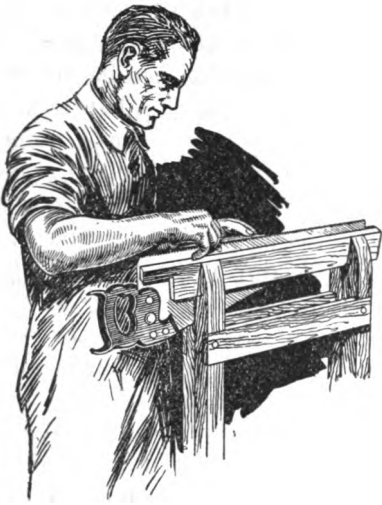
FIG. 62.—Jointing a saw.
