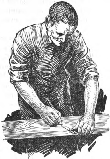
FIG. 69.—Using sliding T-bevel.
