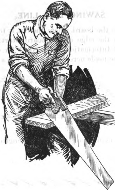
FIG. 5.—Sawing to a line.
