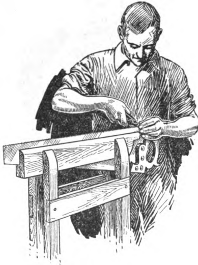
FIG. 63.—Setting a saw.
