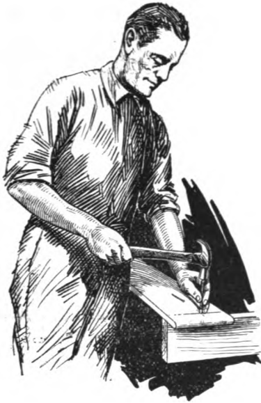
FIG. 10.—Using nail set.
