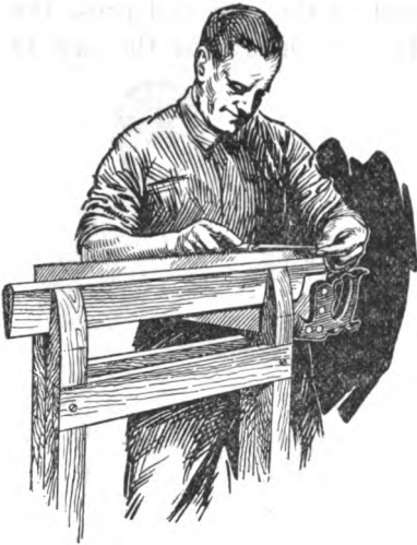
FIG. 64.—Sharpening a saw.
