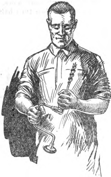
FIG. 8.—Tightening bit in brace.
