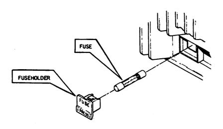
Figure 2-3 Internal Power and AC Line Fuse Replacement (FM/AM-1100S)
