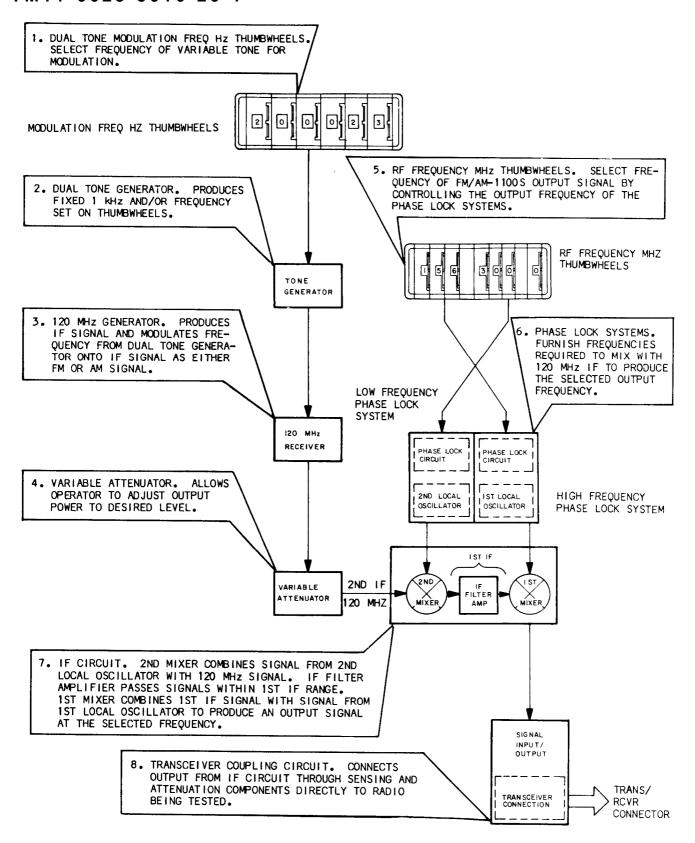
Figure 1-2 Signal Generator Operation (FM/AM-1100S)
