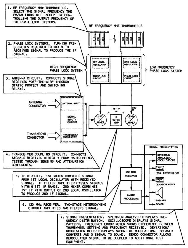
Figure 1-1 Receiver Operation (FM/AM-1100S)
