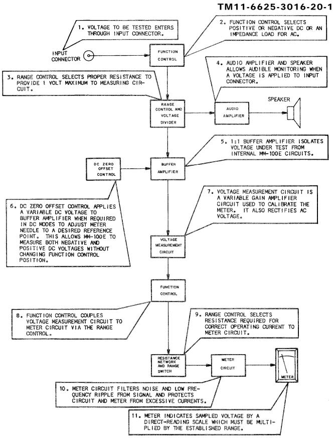
Figure 1-5 AC/DC Voltmeter Operation (MM-100E)
