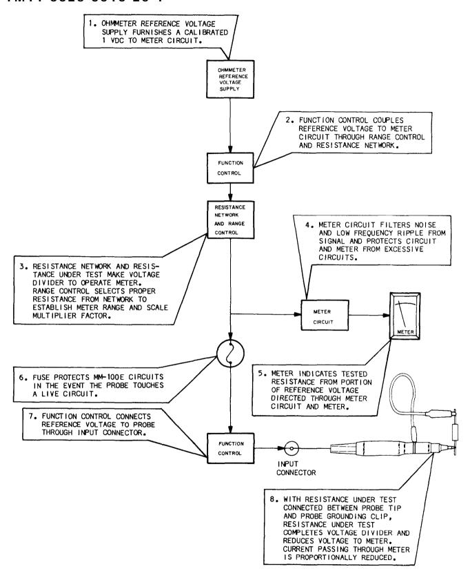
Figure 1-6 Ohmmeter Operation (MM-100E)
