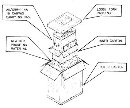
Figure 2-6. Packing the AN/GRM-114A.
