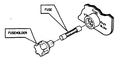
Figure 2-5 Fuse Replacement (MM-100E)
