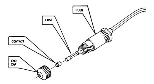
Figure 2-4 DC Power Cord Fuse Replacement (FM/AM-1100S)
