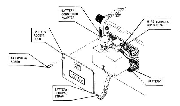
Figure 2-1 Battery Removal and Installation
