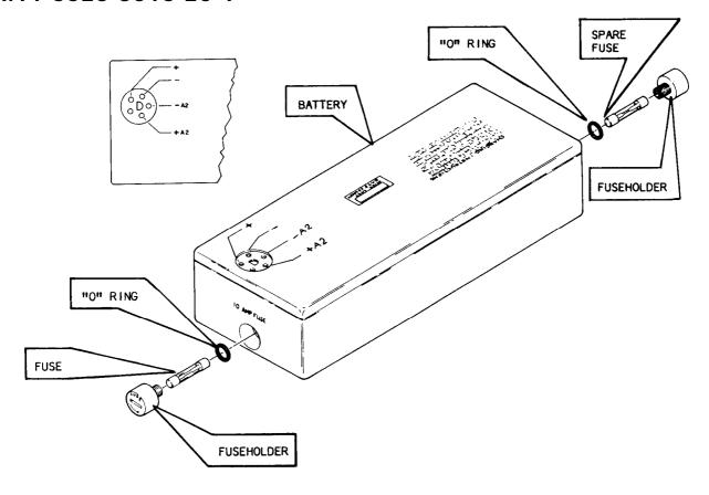
Figure 2-2 Battery Fuse Replacement (FM/AM-1100S)
