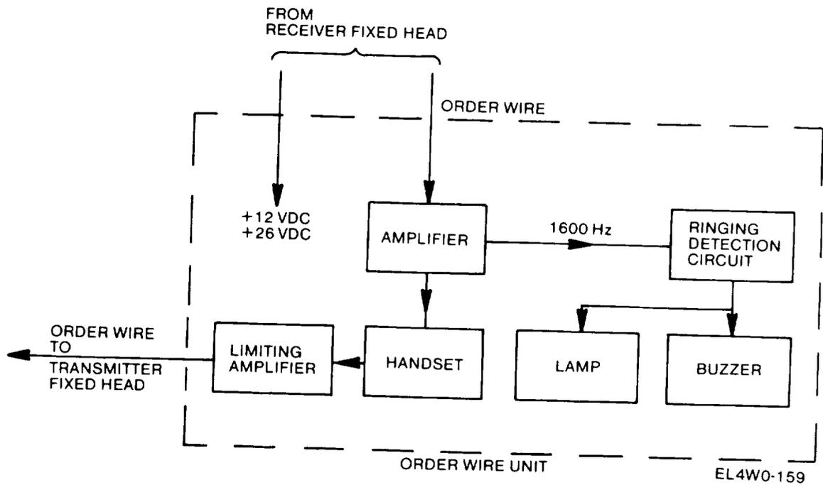
The order wire unit amplifier circuits provide the proper audio levels to the handset and from the handset to the transmitter fixed head. A 1,600 Hz signaling tone is generated for operation of the call buzzer.
