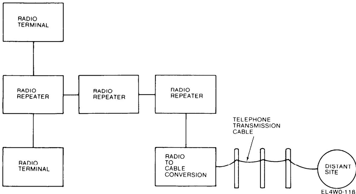
Information is conveyed throughout the communication system in the form of pulses, which are regenerated at each terminal or repeater site.
