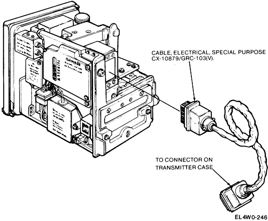
B Connect the transmitter rf head to the connector on the transmitter case by Cable, Electrical, Special Purpose CX-10879/GRC-103(V).
