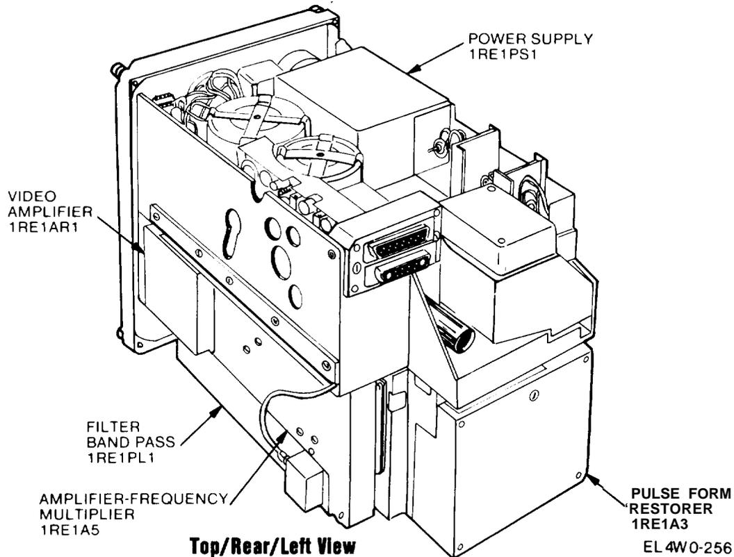
**4-15. REPLACEMENT OF MODULES IN RADIO RECEIVER (1 RE1) R-1329(P)/GRC-103(V), R-1329A(P)/GRC-103(V), R-1329 B(P)/GRC-103(V) Oii R-1329C(P)/GRC-103(V) - Continued**
