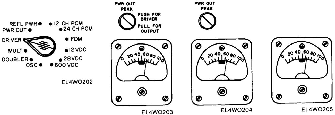
**H** Set transmitter meter switch to PWR OUT and then for:
