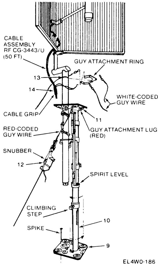
**Extending Launcher and Attaching Guy Wires**
