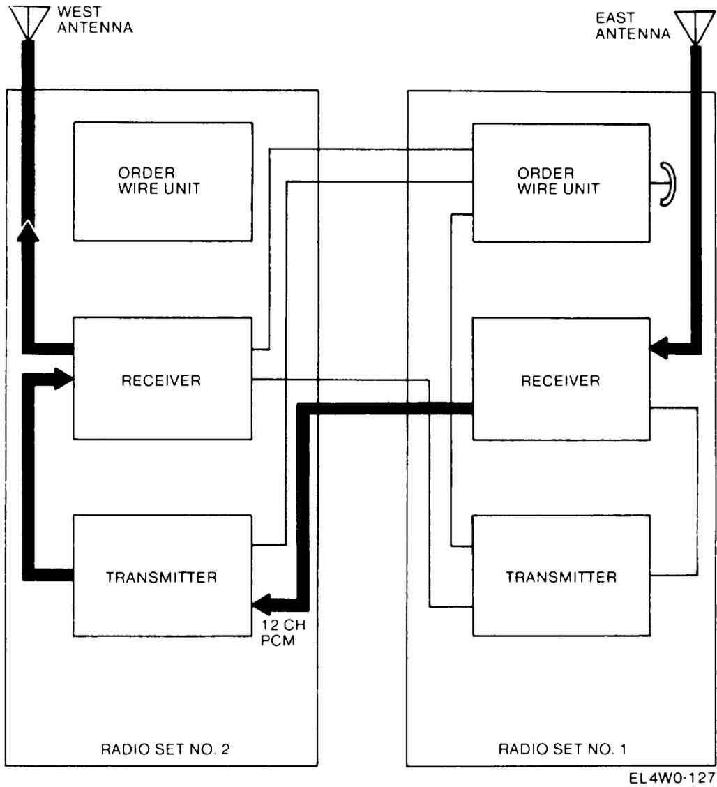
The 12-channel radio repeater uses two radio sets, without any additional multiplex equipment, for the bidirectional reception and transmission of pcm signals. Signals received at the east antenna are regenerated in receiver 1 and fed to transmitter 2 for transmission at the west antenna.
