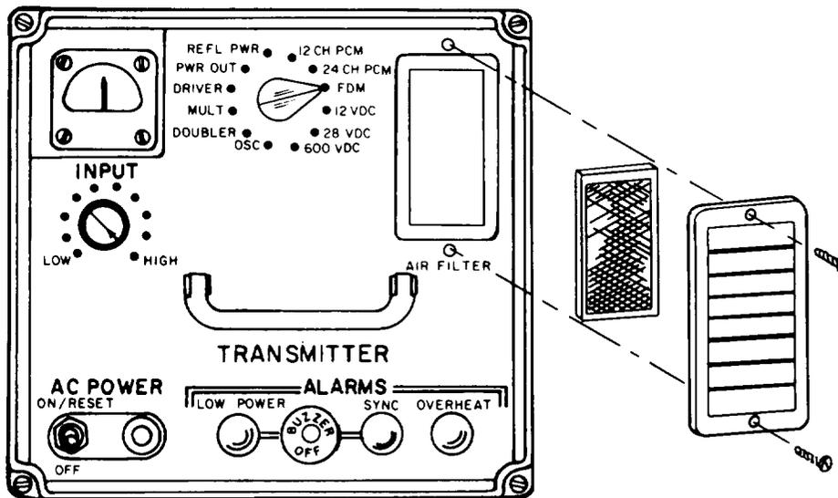
B Remove the dirty filter and replace it with a clean one.
