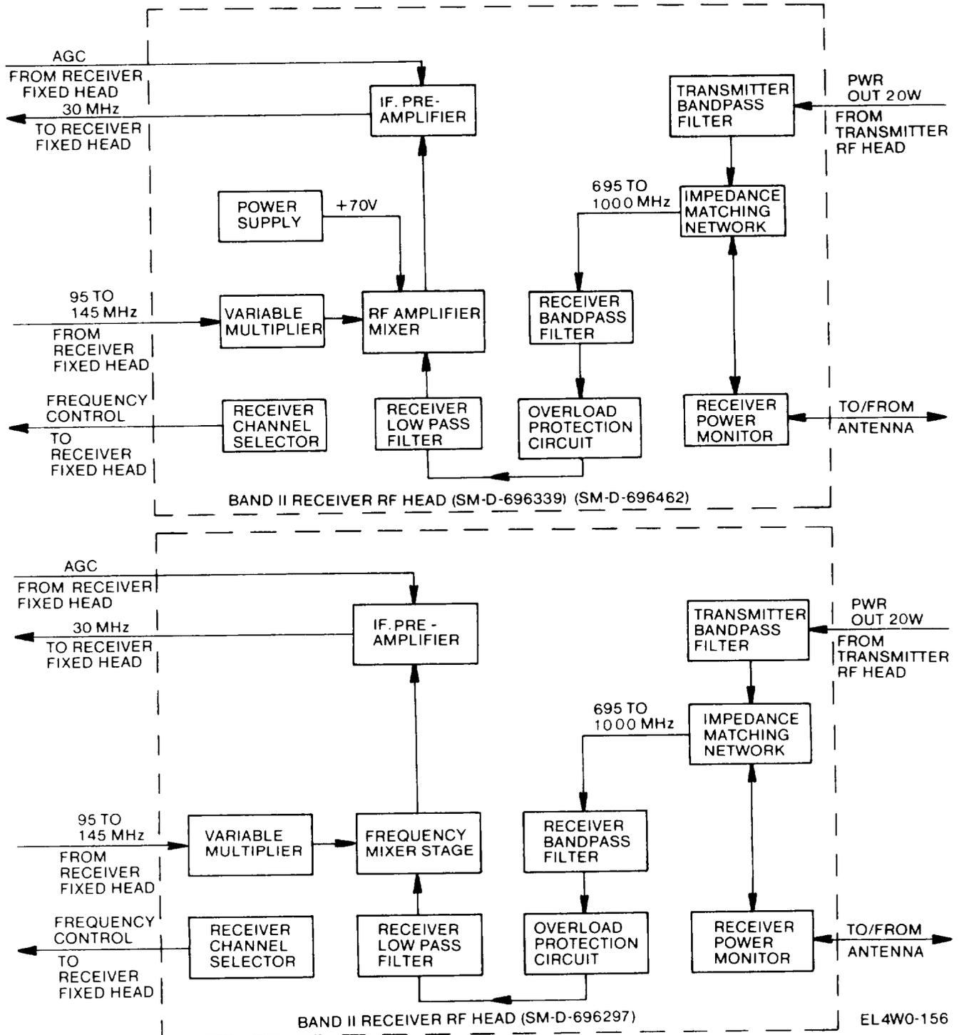
The Band III rf head functions in the same manner as that for Band I except for the frequency mixing stage. The earlier versions of the Band III rf head, SM-D-696339 and SM-D-696462, employ an rf amplifier mixer and power supply. The later version, SM-D-696297, employs a frequency mixer stage.
