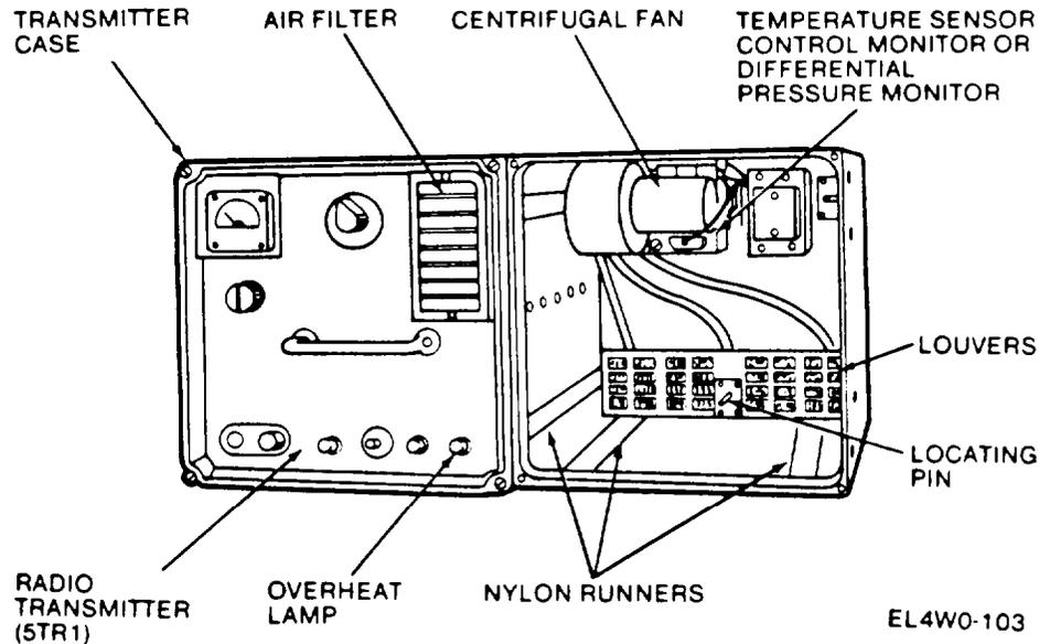
The radio transmitter consists of a case and radio transmitter 5TRI which plugs into the case. The case houses two plug-in units, radio transmitter 5TRI and an amplifier-frequency multiplier. Nylon runners guide these plug-in units into position and locate them by means of pins. A centrifugal fan is mounted on the case partition. Air is drawn in through an air filter on the front panel of radio transmitter 5TRI and passed out through louvers at the rear of the transmitter case,
