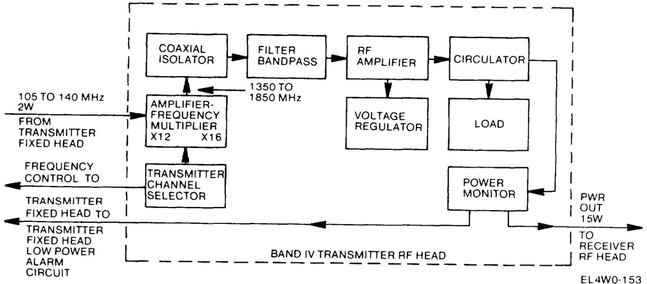
The Band IV transmitter rf head functions in the same manner as that for Band I except that it does not contain a control monitor; frequency multiplication is by 12 or 16; and, a coaxial isolator and band-pass filter, as well as a circulator and dummy load, are employed.
