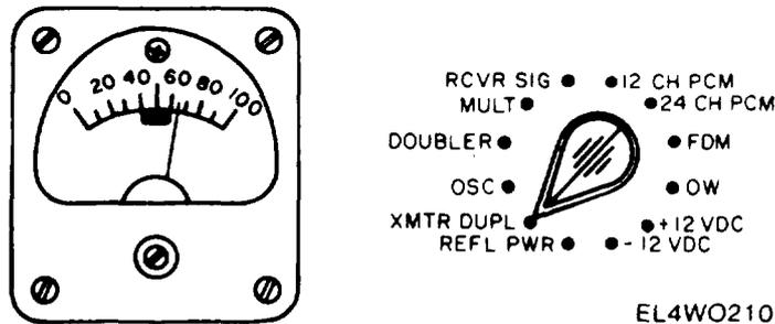
Q Set receiver meter switch to REFL PWR. The meter reads less than 20% of full scale.
