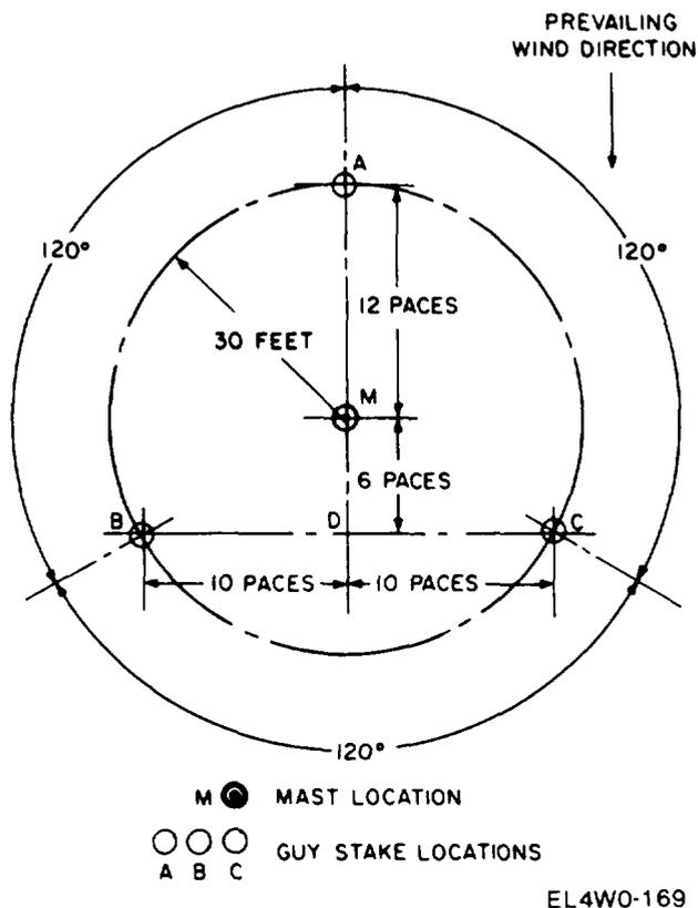
Unload the antenna system in the central clear area, open the accessories kit, as shown, and proceed as follows:
