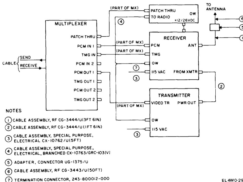
PCM Terminal, 24 Channels, Radio-to-Cable Conversion for Receiver, Radio R-1329C(P)/GRC-103(V)
