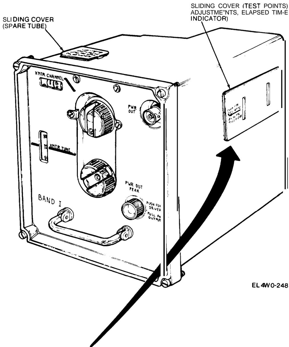
E Remove the cover plate over the test points on the transmitter rf head.
