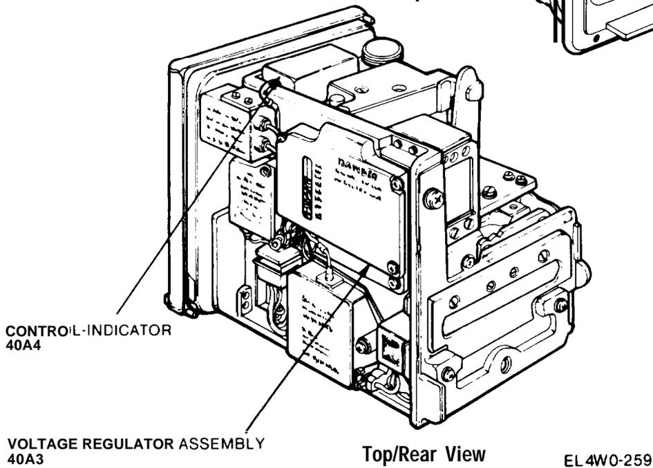
**4-13. REPLACEMENT OF MODULES IN AMPLIFIER/FREQUENCY MULTIPLIERS AM-4321 /GRC-103(V), AM-4321 B/GRC-103(V), AM-4322/GRC-103 (V), AM-4322A/GRC-103(V) OR AM-4323/GRC-103(V) - Continued**
