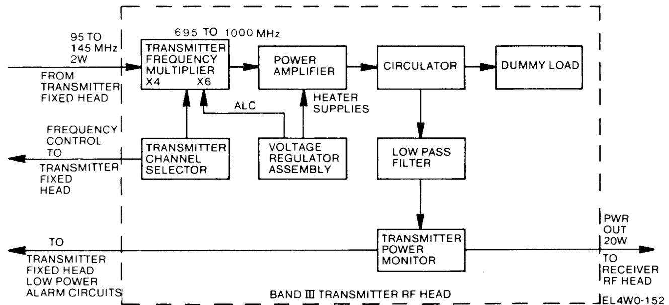
The Band III transmitter rf head functions in the same manner as that for Band I except that it does not contain a control monitor: frequency multiplication is by 6 or 8, and, a voltage regulator, a circulator, and a dummy load are used.
