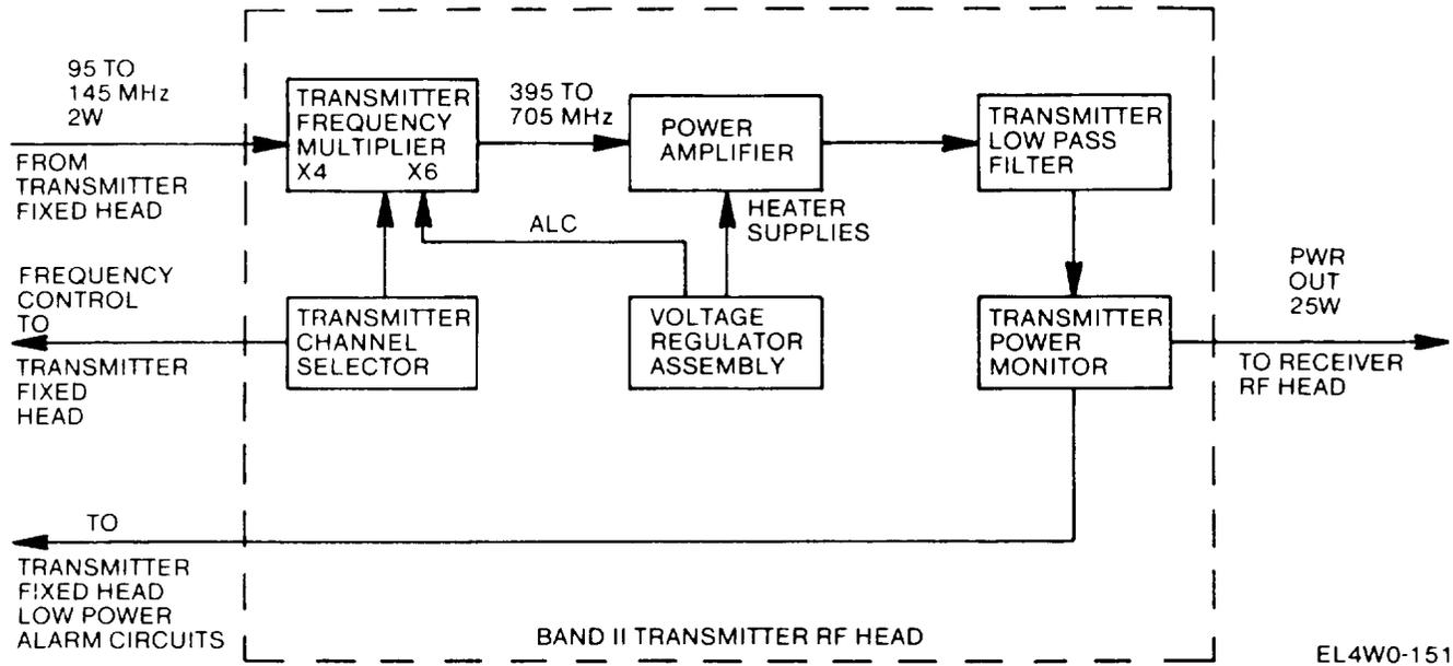
The Band II transmitter rf head functions in the same manner as that for Band I except that it does not contain a control monitor, frequency multiplication is by 4 or 6; and, a voltage regulator is used.
