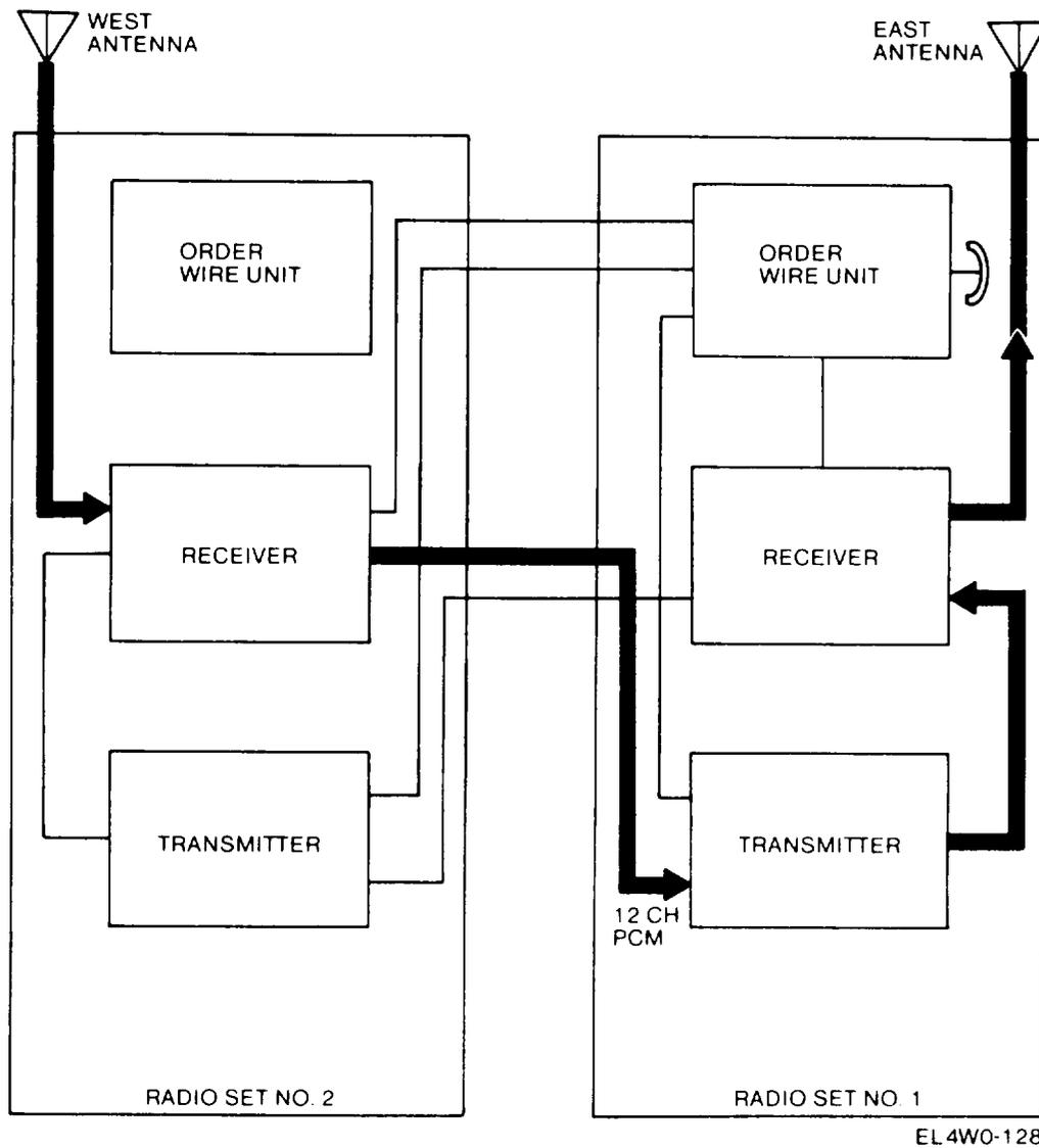
Signals received at the west antenna are regenerated in receiver 2 and fed to transmitter 1 for re-transmission at the east antenna.
