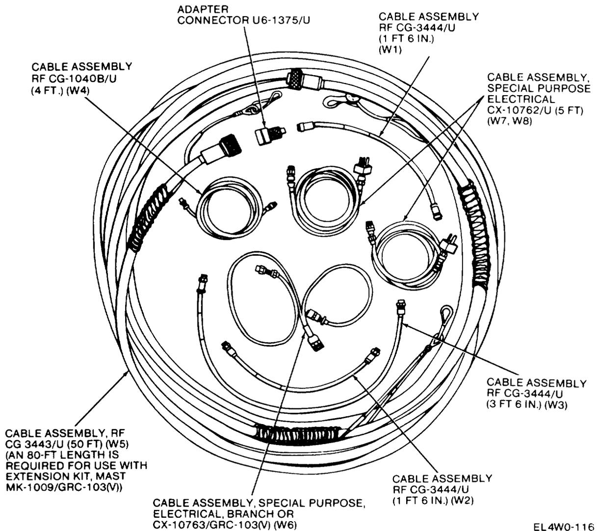
The radio set includes a group of rf, video and power cables used to Interconnect the various components,
