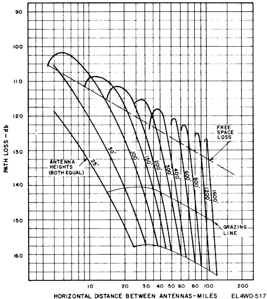
Figure E-17. Pathless Between Half-Wave Dipoles Over Smooth Curved Earth at 1,000 MHz
