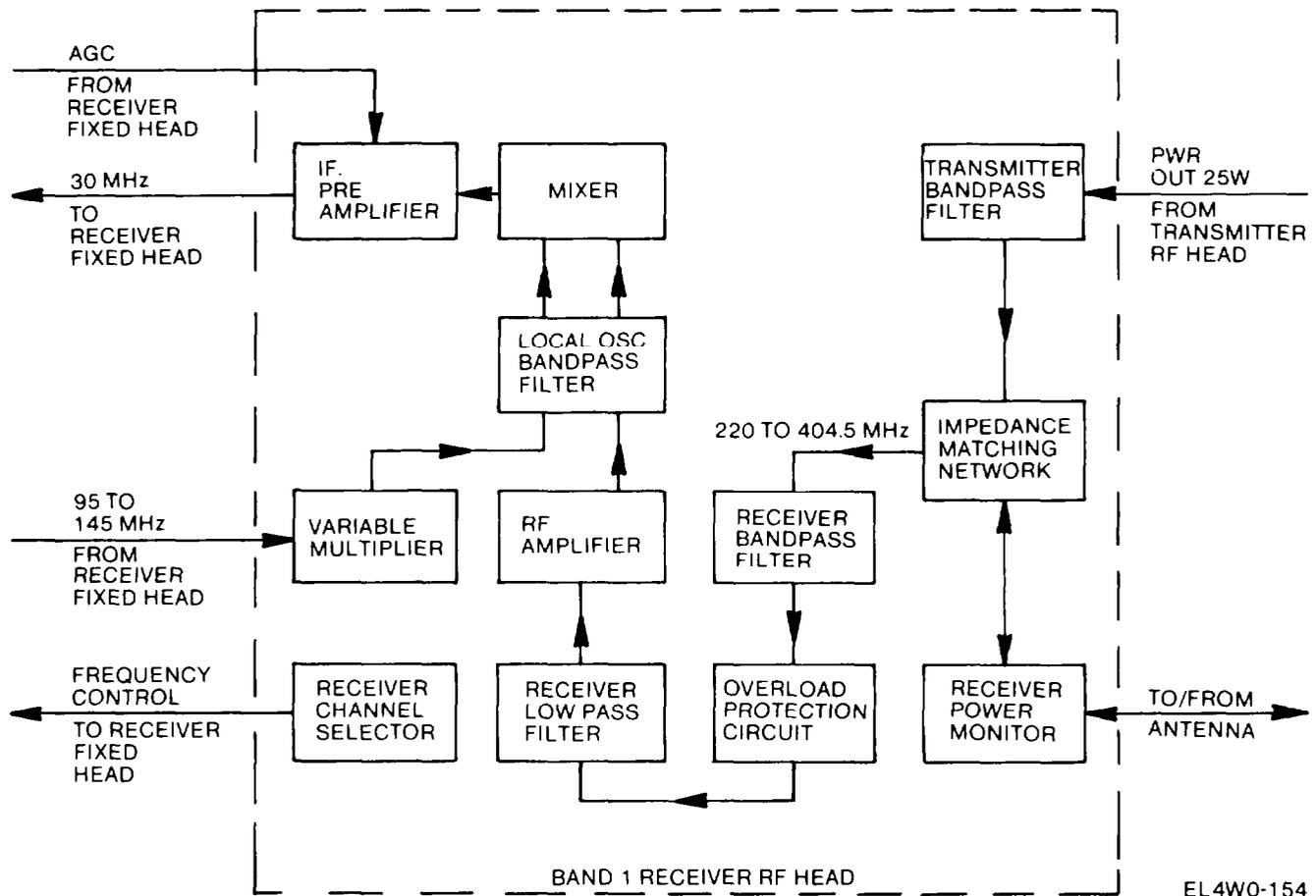
The Band I receiver rf head contains the antenna duplexing network and the circuits necessary to convert the incoming signal to an intermediate frequency (if.) of 30 MHz for application to the receiver fixed head.
