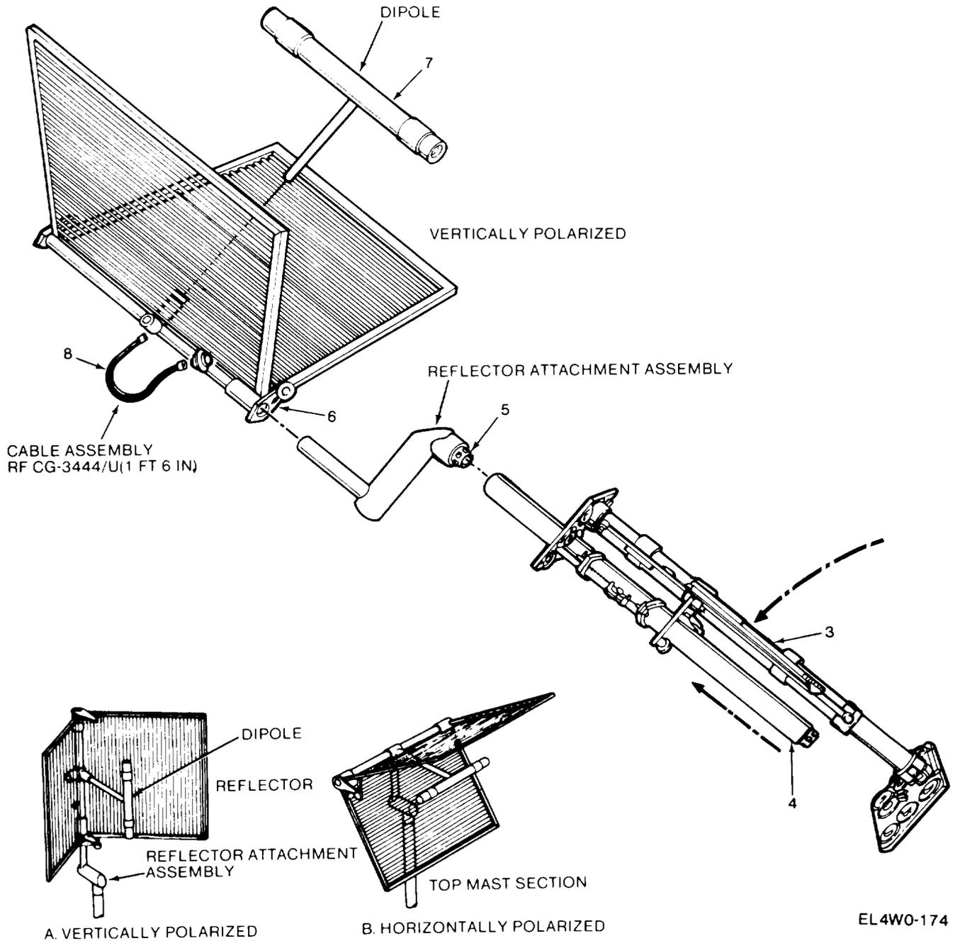
**Polarization and Mounting Antenna on Mast**
