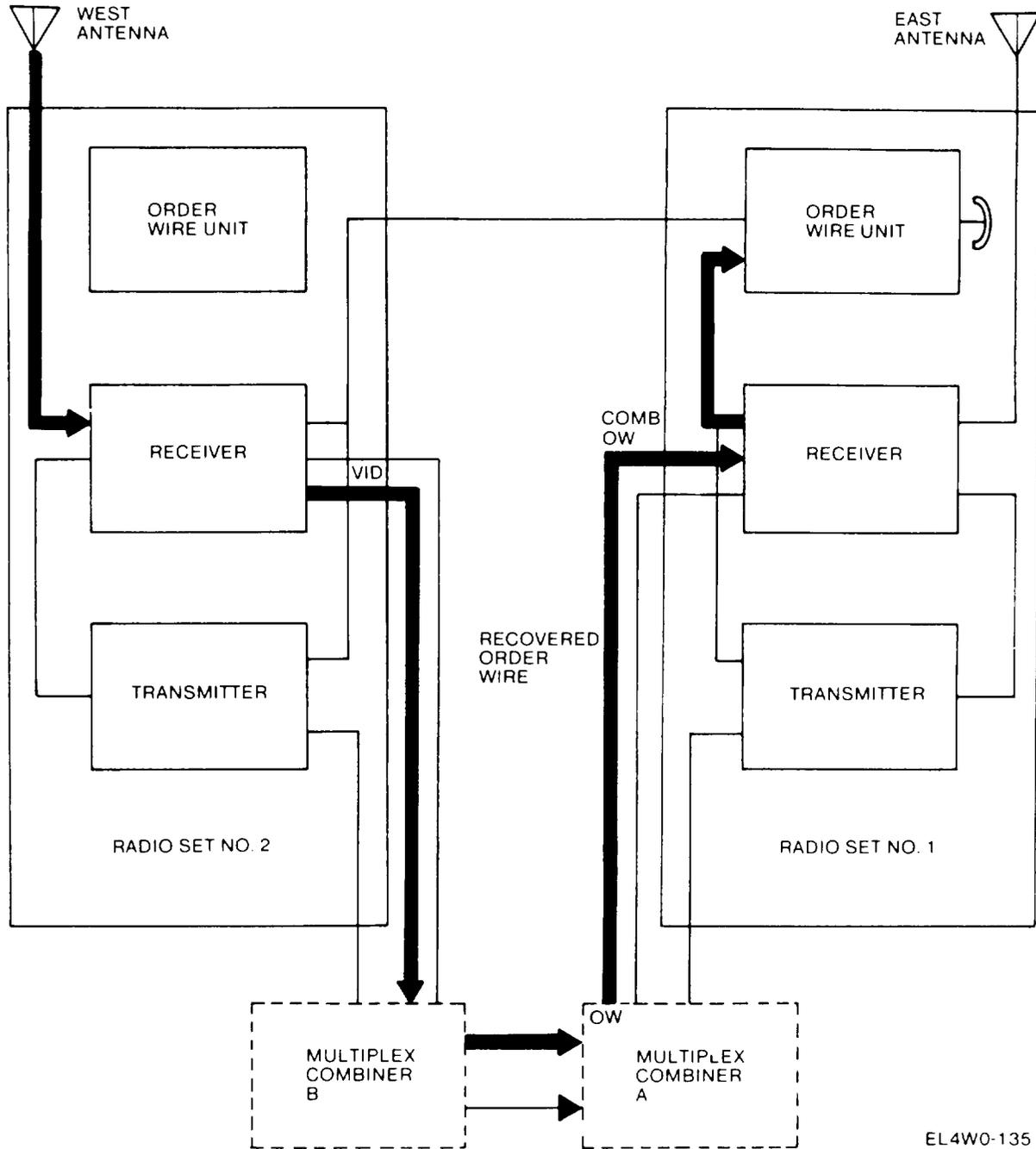
Order wire signals from the west antenna are passed through receiver 2 to combiner B where they are regenerated and fed through combiner A and receiver 2 to the order wire unit.
