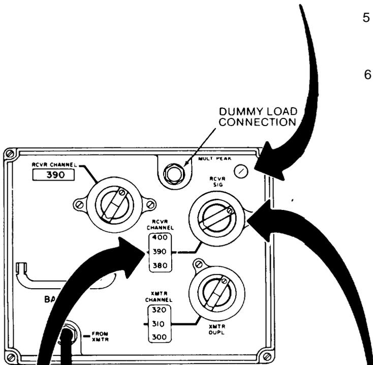
7 Set the receiver meter switch to RCVR SIG.
