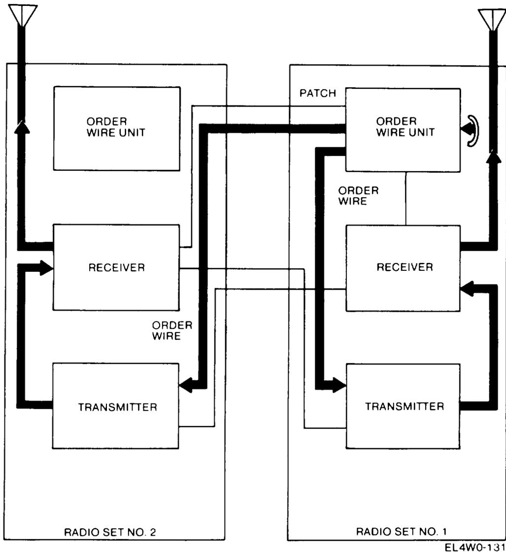
Only one order wire unit is required for the two radio sets at a radio repeater site. Local order wire signals are applied directly to both transmitters and passed through the receivers to the antennas.
