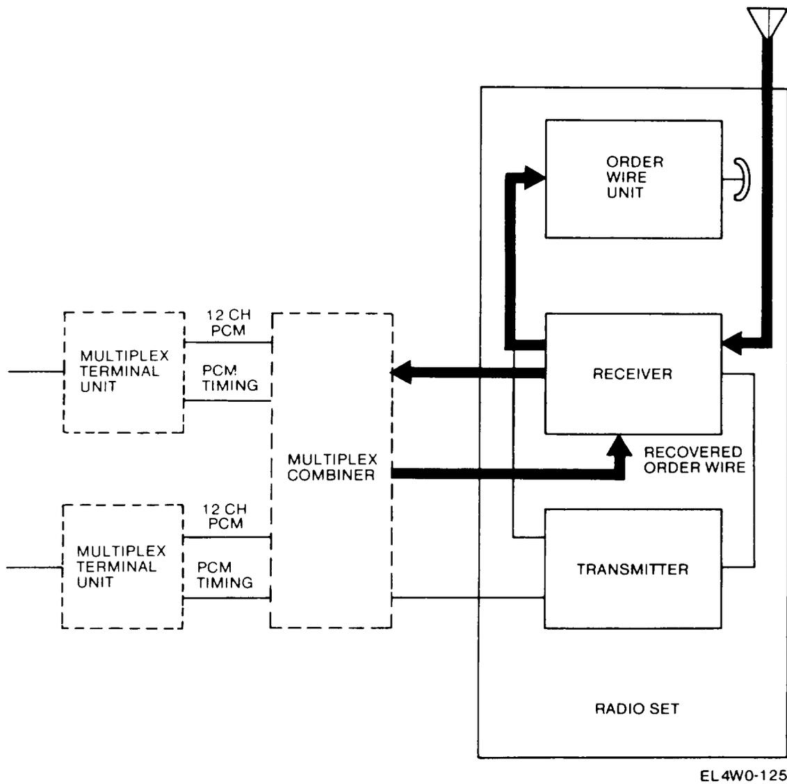
The multiplex combiner also recovers any order wire information from the received signals and feeds it back to the receiver as a recovered order wire signal. From the receiver, it is supplied to the order wire unit.
