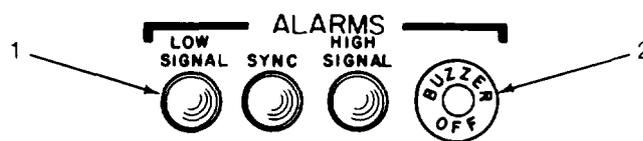
**X** Wait until LOW SIGNAL lamp goes out. Loud rushing noise in order wire unit handset disappears.
