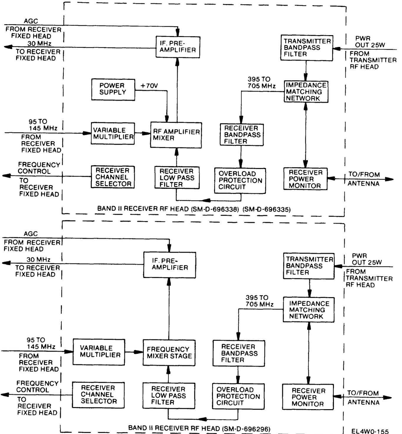
The Band II rf head functions in the same manner as that for Band I except for the frequency mixing stage. The earlier versions of the Band II rf head, SM-D-696339 and SM-D-696335, employ an rf amplifier mixer and power supply. The later version, SM-D-696296, employs a frequency mixer stage.
