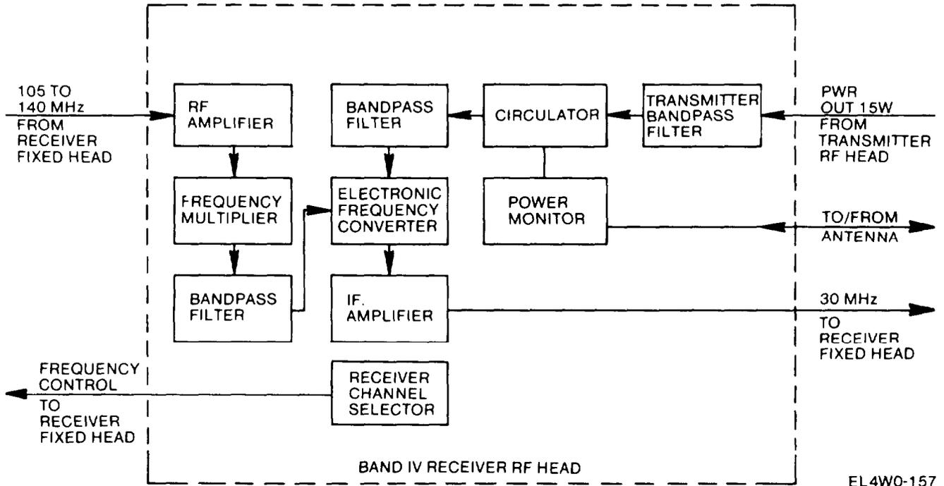
The Band IV rf head functions in the same manner as that for Band I except that it employs a circulator instead of an impedance matching network, the frequency mixing circuitry consists of an rf amplifier, frequency multiplier, bandpass filter and electronic frequency converter, and it has no overload protection circuit.
