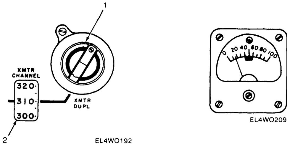
P Set receiver meter switch to XMTR DUPL. The meter reads between 25% and 90% of full scale.
