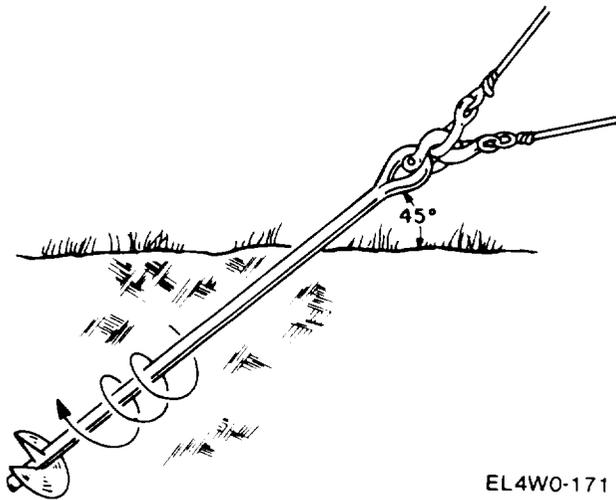
**D** Use hammer handle to screw anchor into ground.
