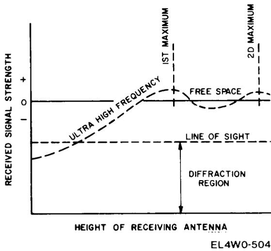
**Figure E-4. Results of Wave Propagation Phenomena**
