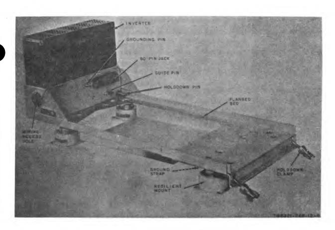
Figure 4. Power-Inverter, Mounting PP-3702/ARC-108.
