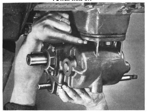
Figure 180 — Installing Power Take-off
