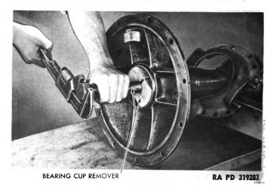
Figure 93 - Removing Differential Bearing Cups
