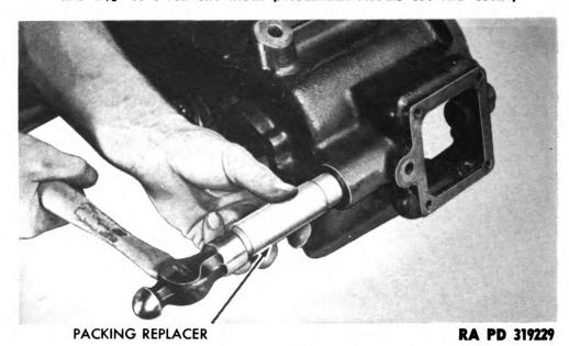
Figure 61 — Installing Shift Shaft Oil Seal
