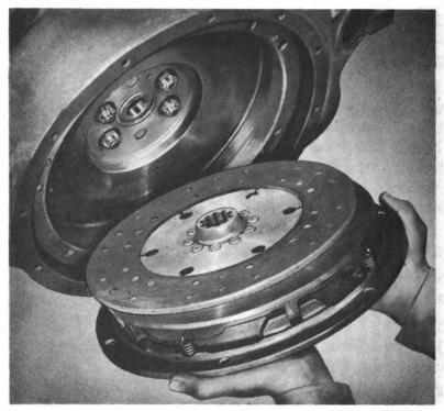
RA PD 319372 Figure 10 — Removing Clutch Assembly
