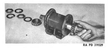
Figure 74 - Removing Pillow Block Shaft
