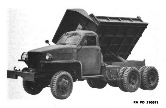
Figure 7 — 148-inch Wheelbase Side Dump Model Truck US6 (6x6) — Body Raised
