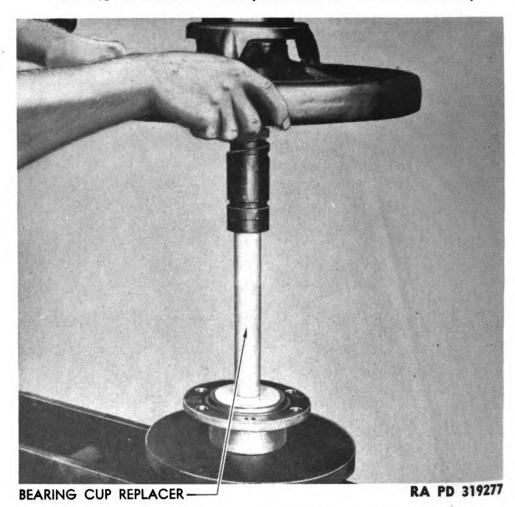
Figure 96 — Installing Drive Pinion Bearing Cups
