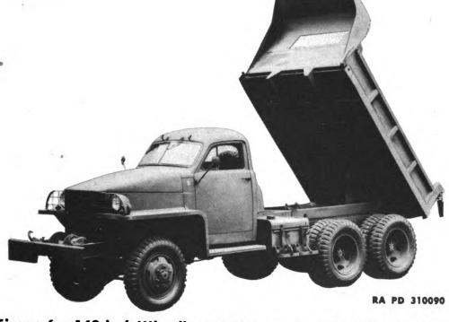
Figure 6 — 148-inch Wheelbase End Dump Model Truck US6 (6x6)
