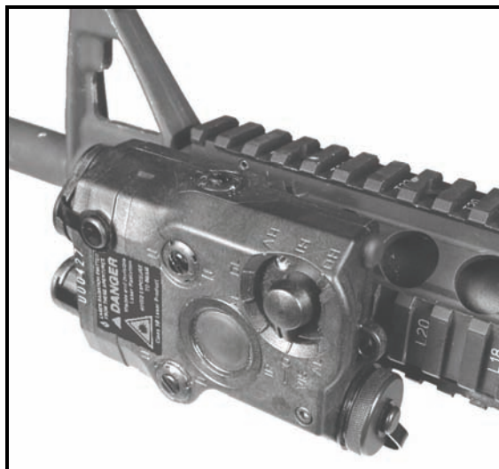
Figure 2-34. AN/PEQ-15 mounted on M4 carbine.
