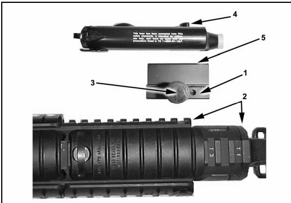
Figure 2-27. Mounting the AN/PAQ-4B/C on the M4 MWS top or left.
