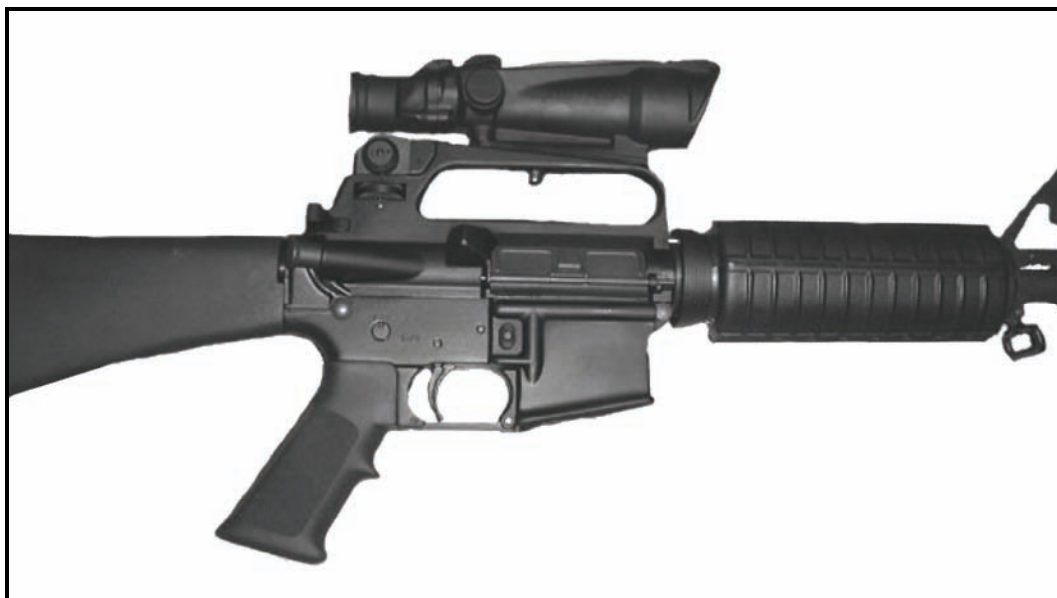
Figure 2-45. Mounting the ACOG on an M16A1/A2/A3 rifle.
