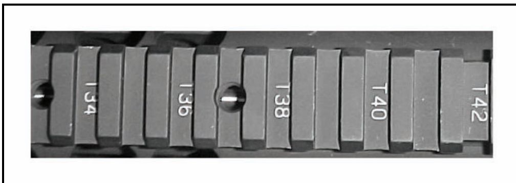
Figure 2-17. Address markings on the adapter rail system.
