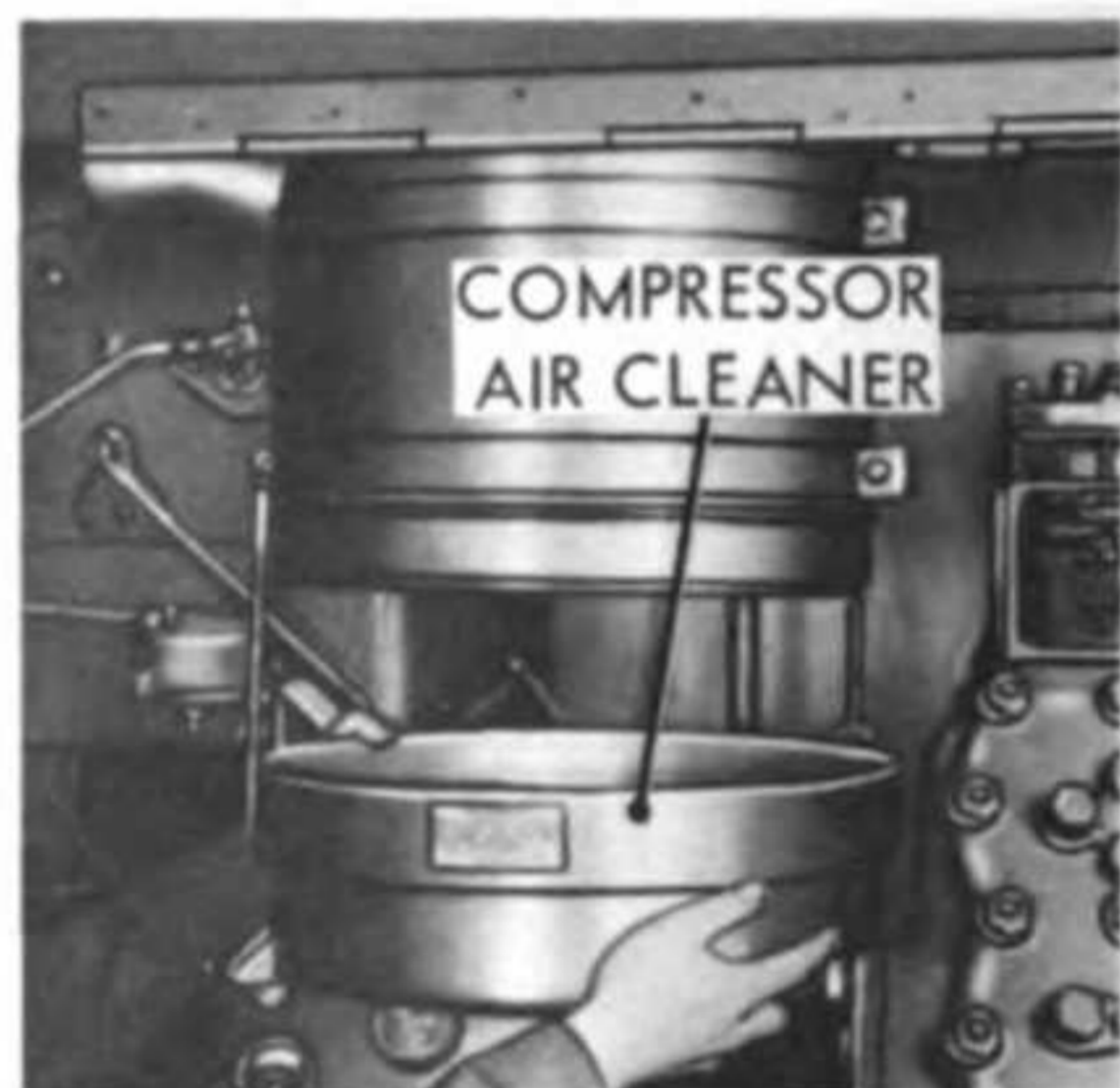
REFERENCE 10: Clean cup and re-fill to level mark.
