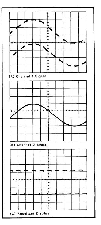
Fig. 1-8. Using the ADD mode for common mode rejection.
