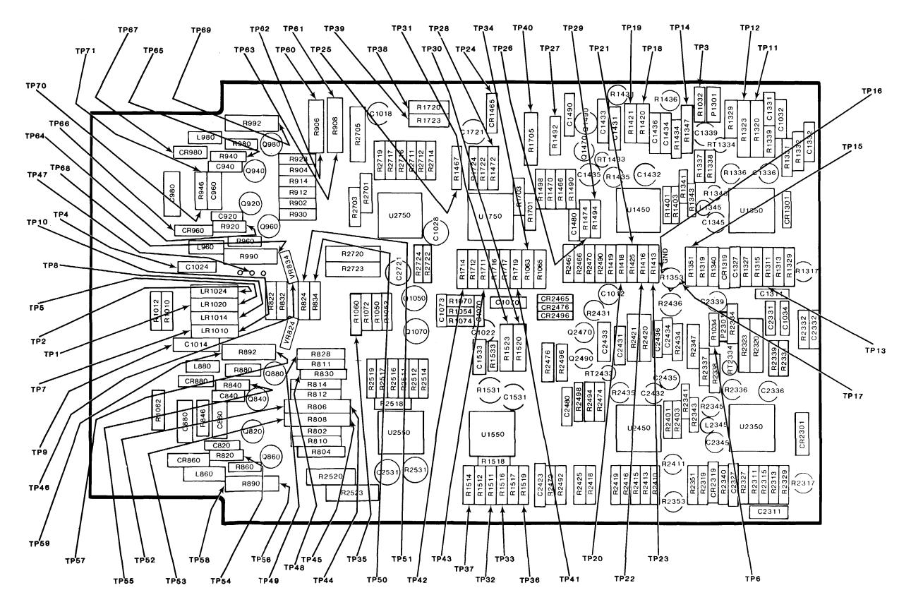
A2 Amplifier Board Test Point Layout Figure FO-4
