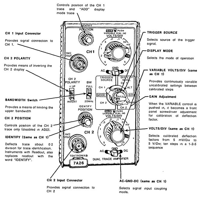
Fig. 1-3. AM-6785/U front-panel controls and connectors.
