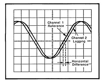
Fig. 1-6. Measuring phase difference between two signals.
