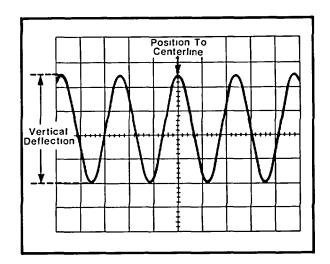
Fig. 1-4. Measuring the peak-to-peak voltage of a waveform.
