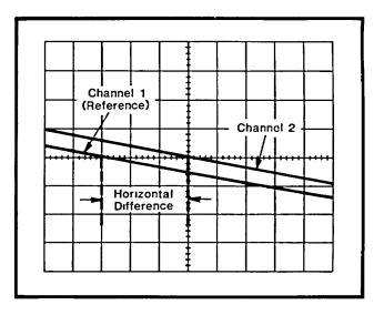
Fig. 1-7. High resolution phase measurement using time-base magnifier.
