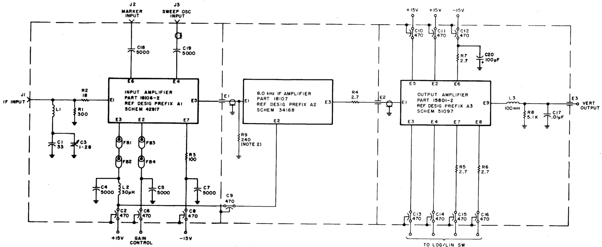
Figure 6-1. Type 724005-1, IF Amplifier Assembly, (A2A1) Schematic Diagram 470156
