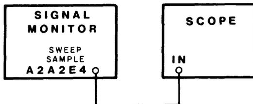
Figure 4-4. Test Setup, Sweep Rate Calibrate
