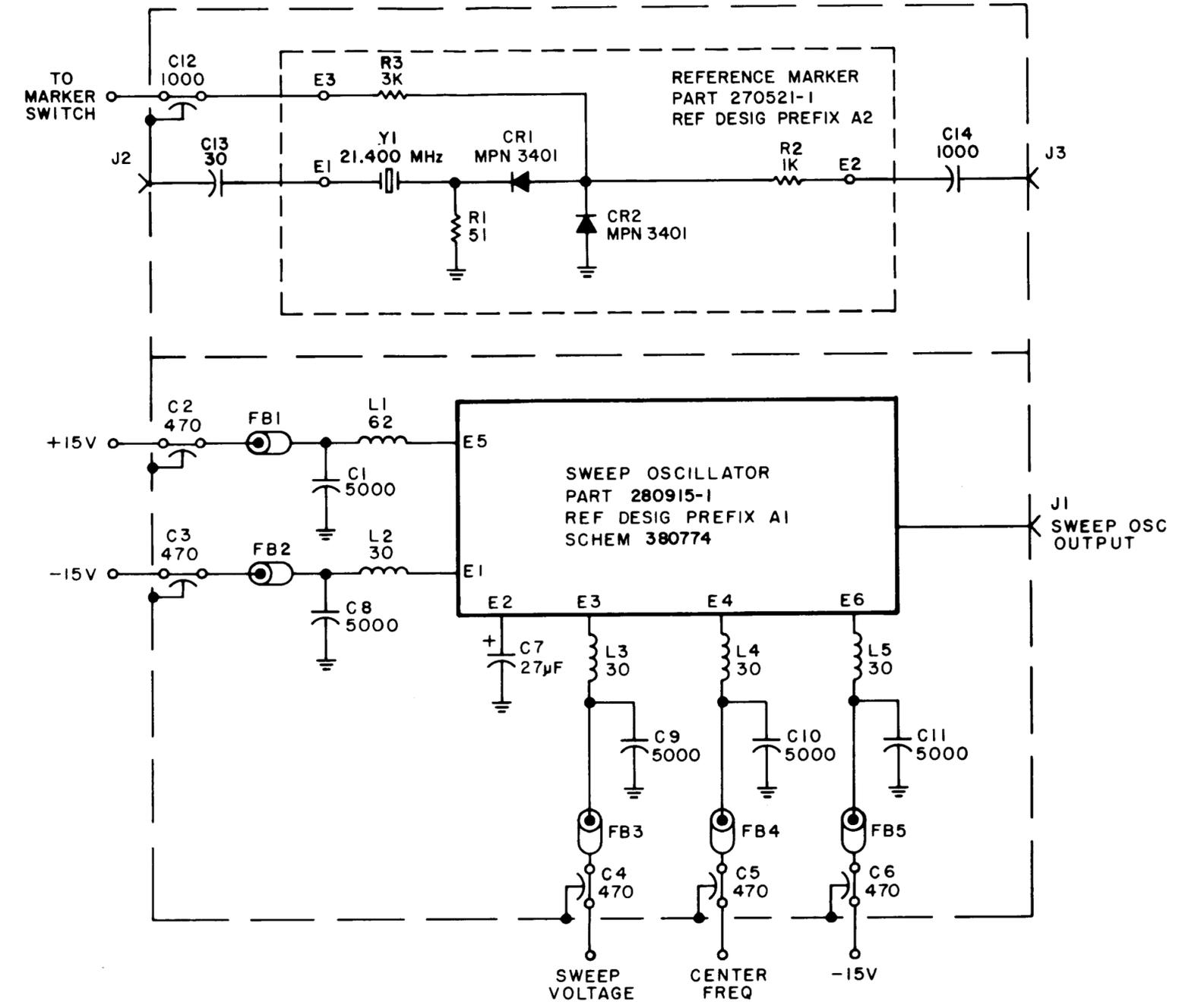
Figure 6-6. Type 774007-1, Oscillator, (A2A3) Schematic Diagram 370315
