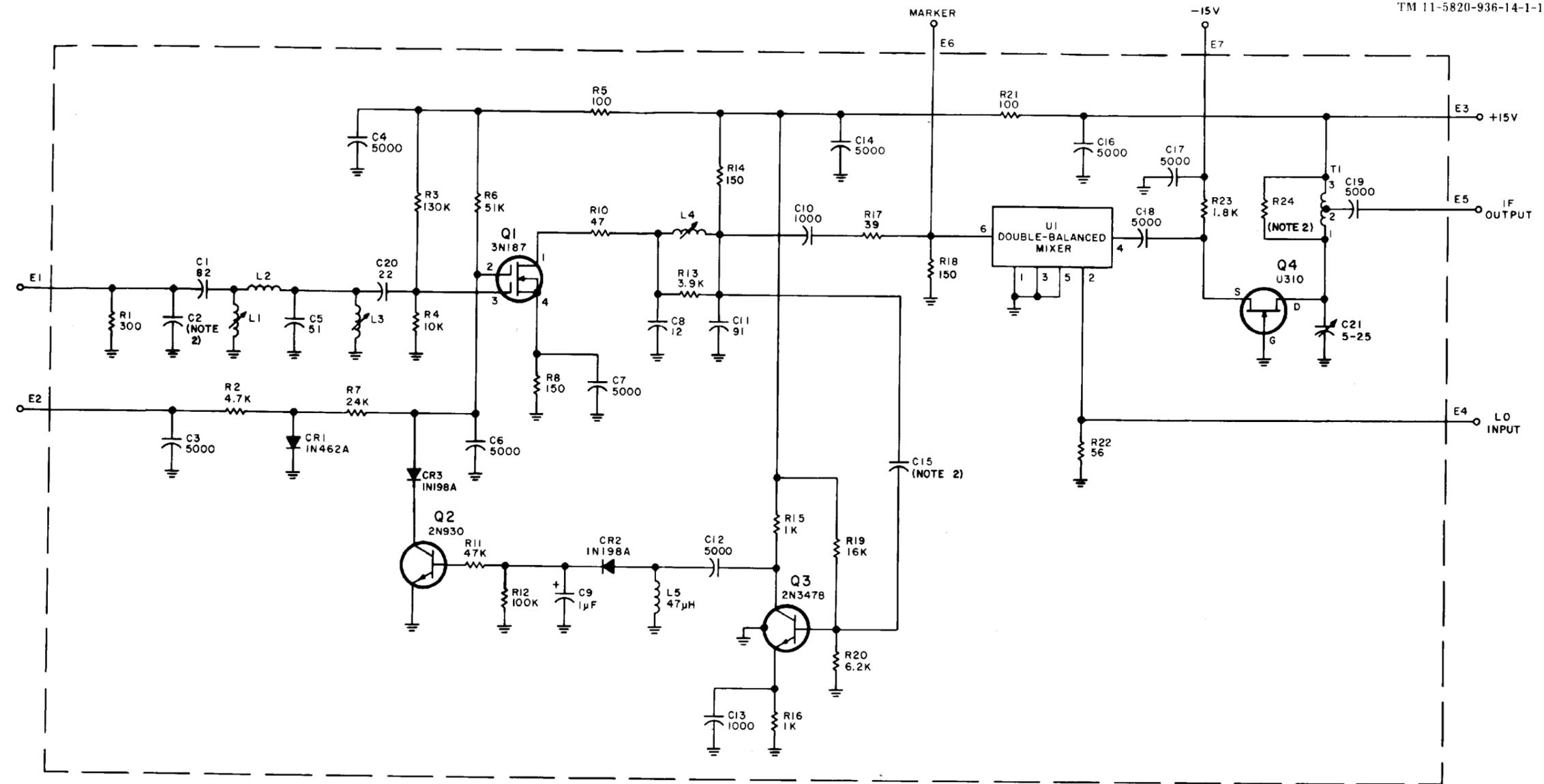
Figure 6-2. Part 18106-2, Input Amplifier, (A2A1A1) Schematic Diagram 42917
