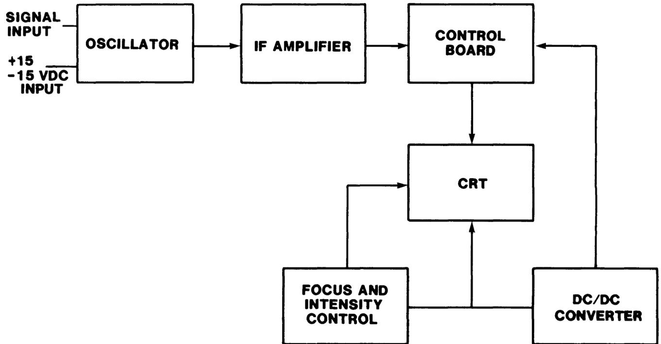
Figure 3-1. Signal Monitor Functional Block Diagram
