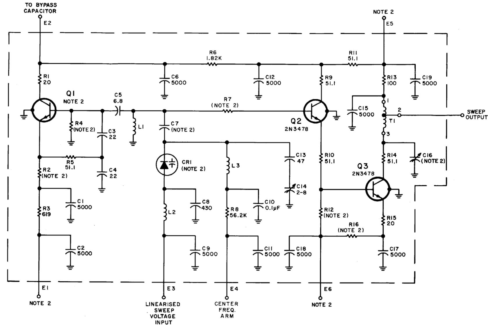
Figure 6-7. Part 15799-3 Sweep Oscillator Assembly, (A2A3A1) Schematic Diagram 32369
