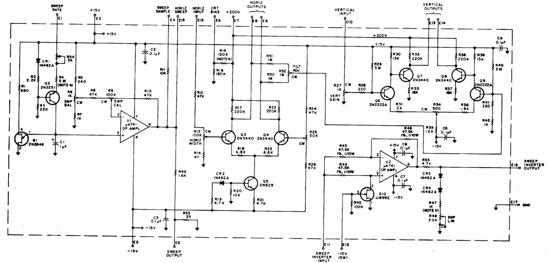
Figure 6-5. Type 824002-1, Control Board, (A2A2) Schematic Diagram 470227
