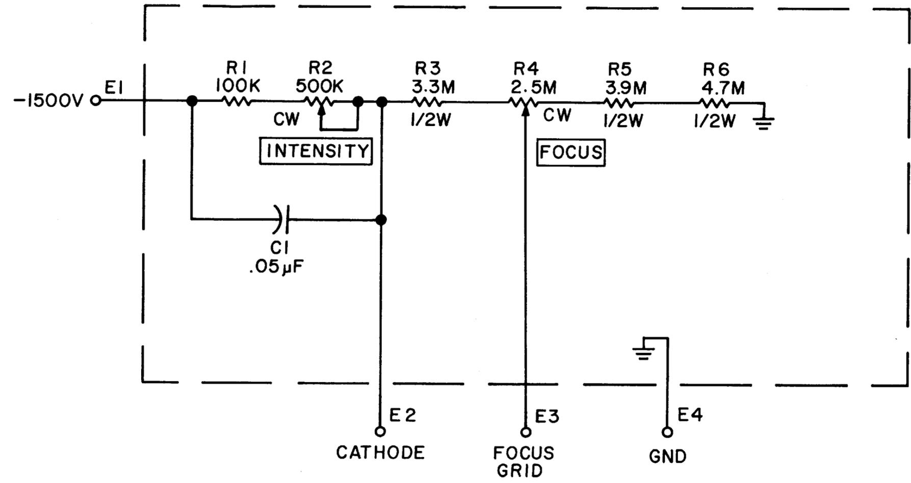
Figure 6-8. Type 794099-1, Focus and Intensity Control, (A2A4) Schematic Diagram 270343
