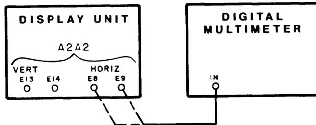
**Figure 4-3. Test Setup, Signal Monitor Deflection Amplifier Initial Alignment**
