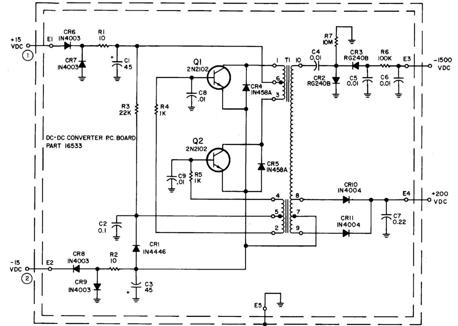
Figure 6-9. Type 764006-1, DC-DC Converter, (A2A5) Schematic Diagram 32874
