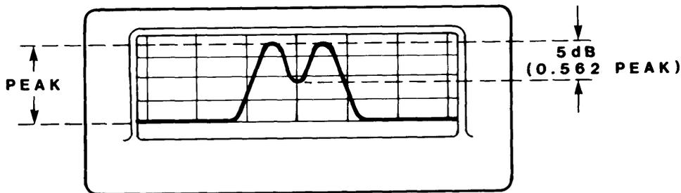
Figure 4-2. Typical Response, Signal Monitor Resolution Test
