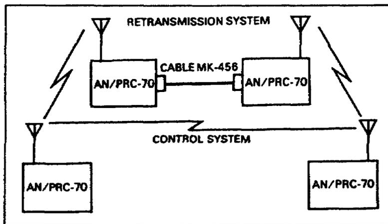
Figure 2-1. AN/PRC-70 retransmission configuration
