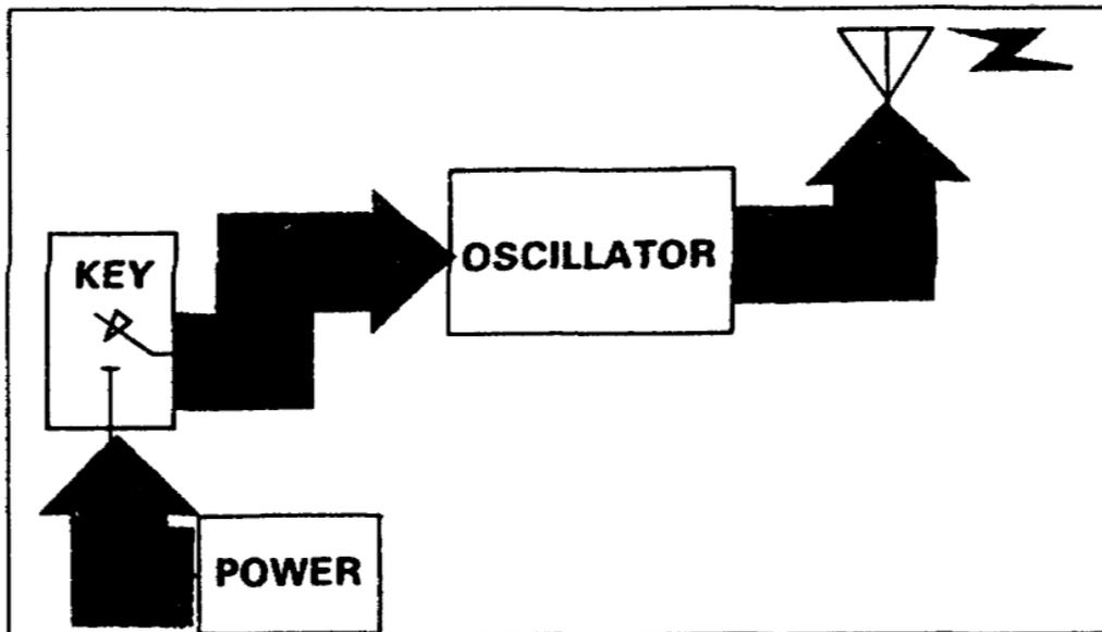
Figure 1-8. Block diagram of a simple radio transmitter
