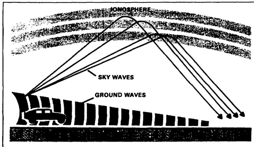
Figure 1-3. Radio wave transmission paths
