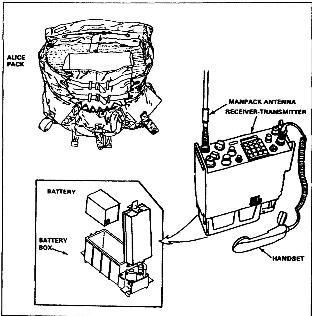
Figure 5-3. Manpack radio AN/PRC-119
