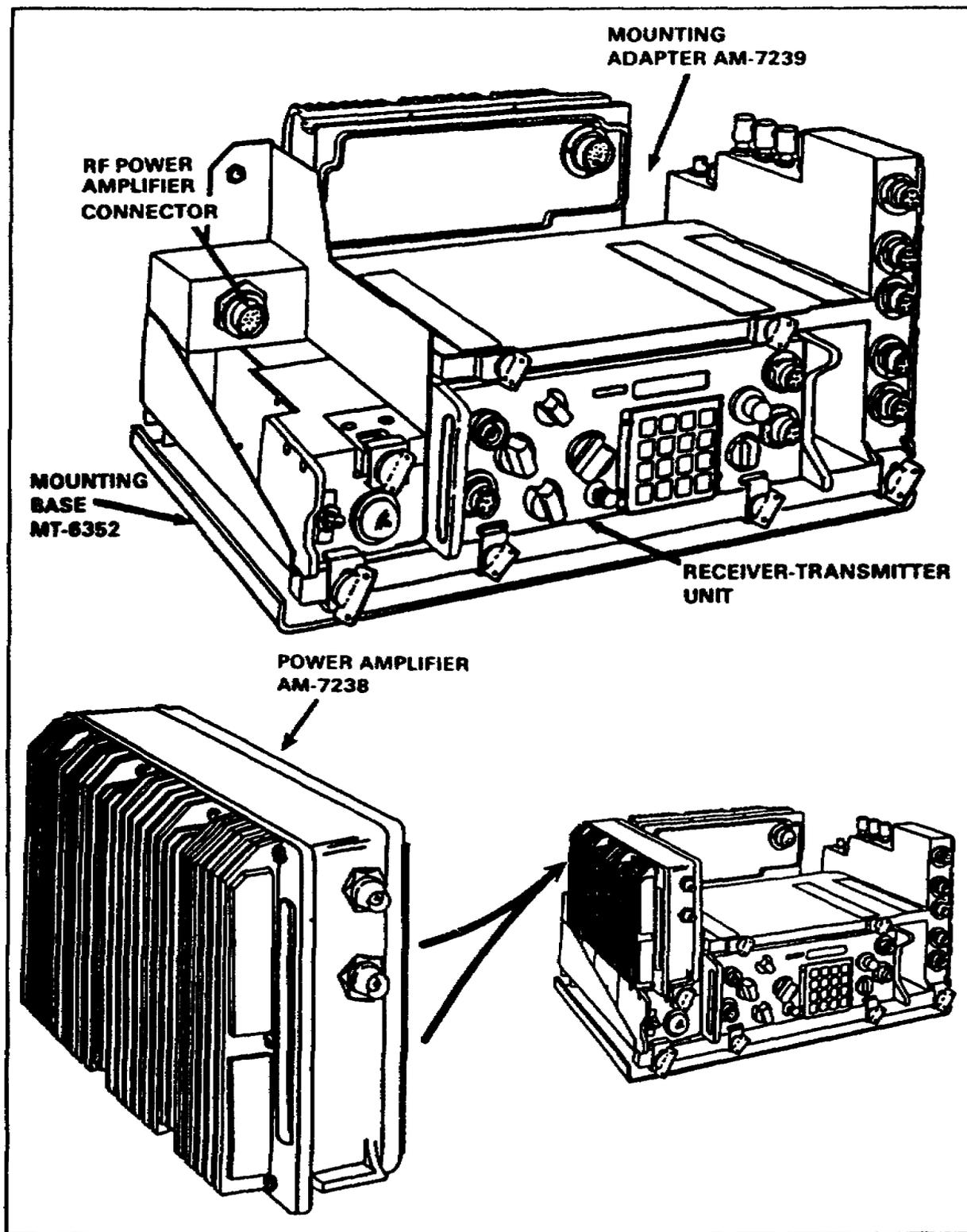
Figure 5-2. Radio set components
