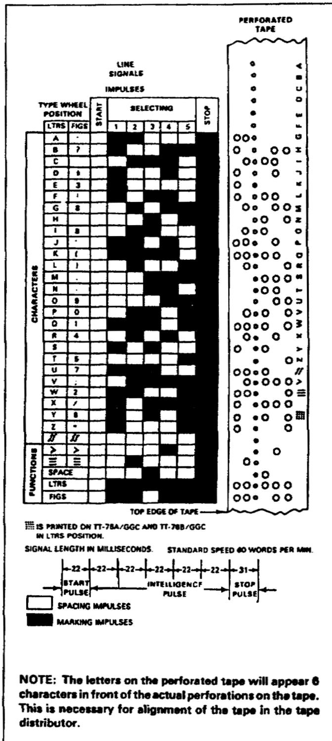
Figure 4-1. Teletypewriter code character set and standard start-stop, five-unit code chart
