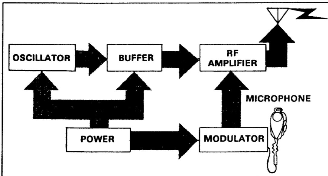
Figure 1-9. Block diagram of a radiotelephone transmitter
