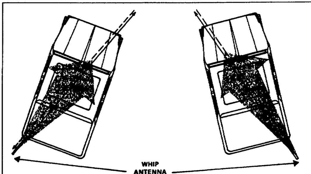
Figure 1-14. Directivity of a vehicle-mounted whip antenna
