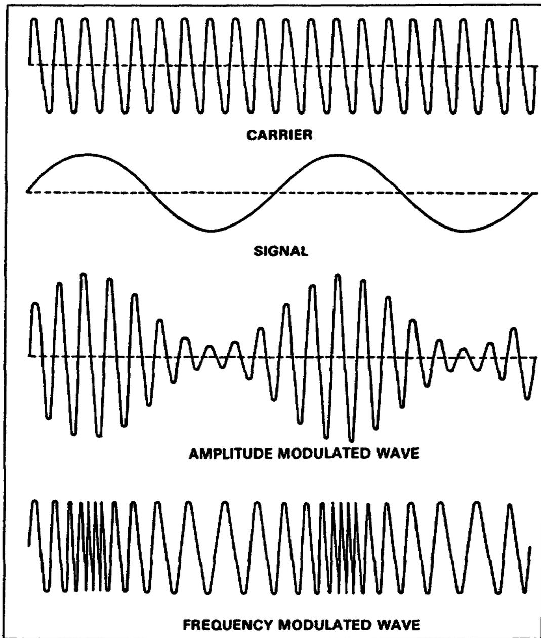
Figure 1-6. AM and FM wave shapes
