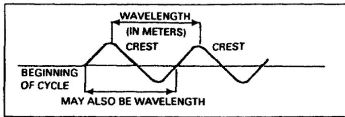
Figure 1-1. Wavelength of a radio wave
