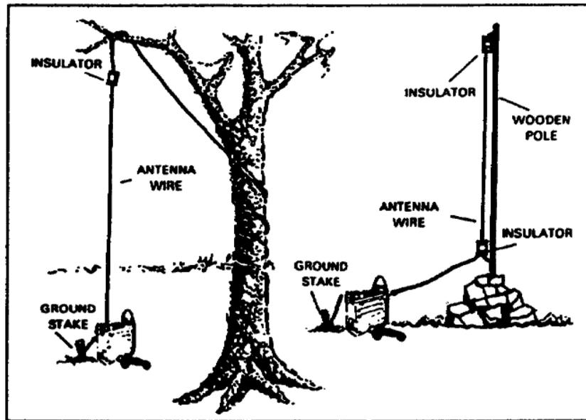
Figure 1-16. Field substitutes for antenna supports
