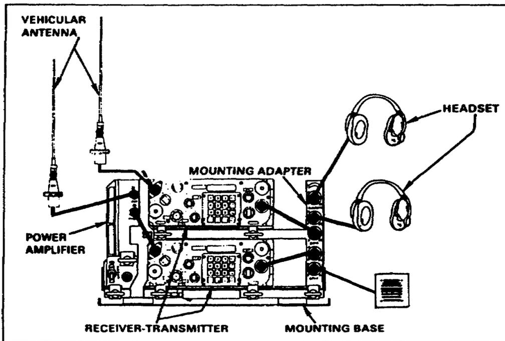
Figure 5-4. Vehicular long-range/short-range radio AN/VRC-89
