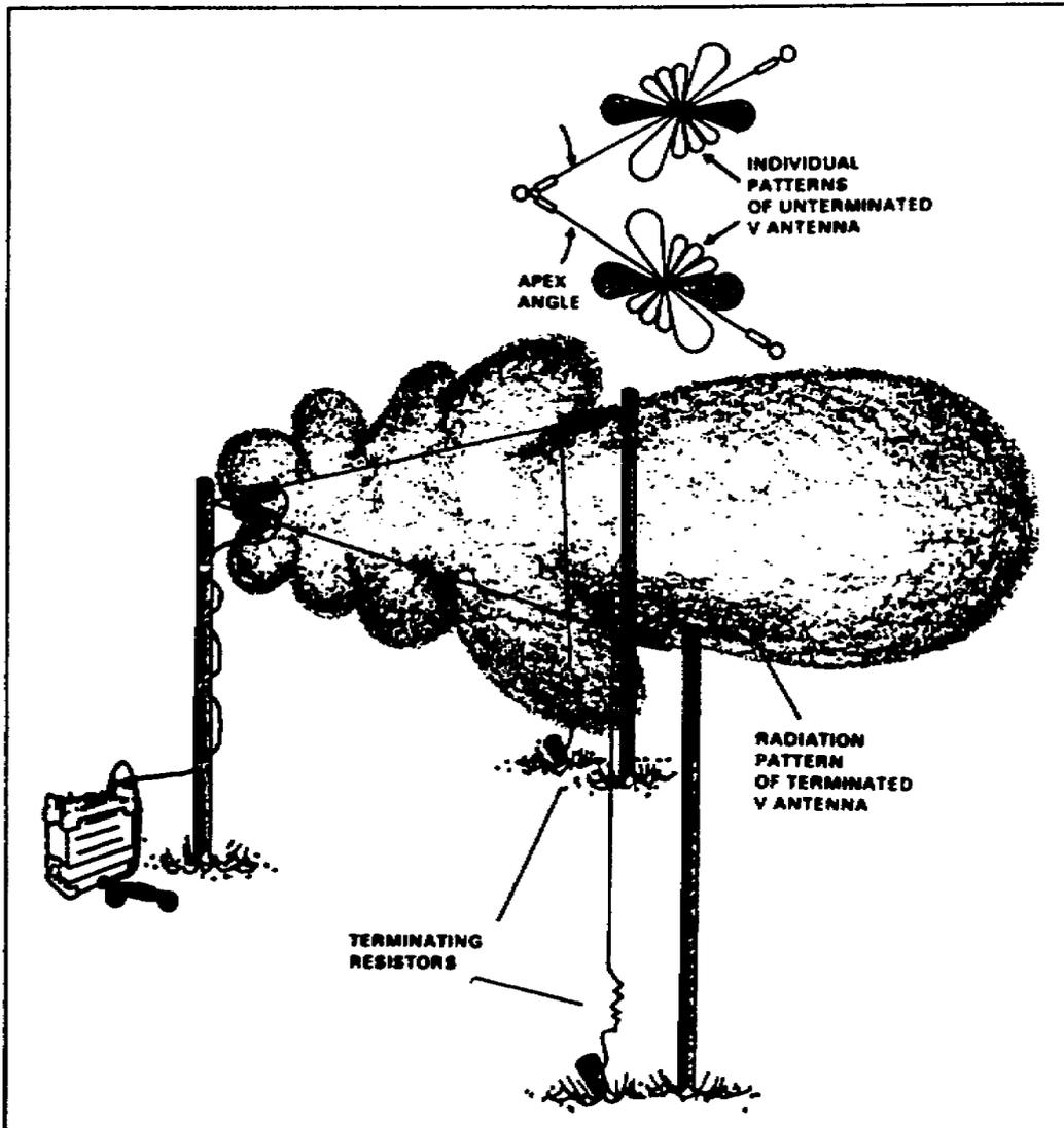
Figure 1-15. Radiation pattern of a V antenna
