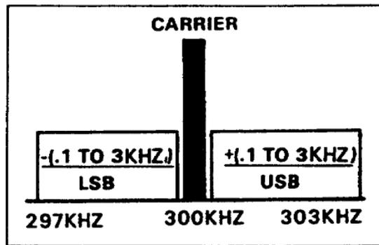
Figure 1-7. AM carrier with sidebands
