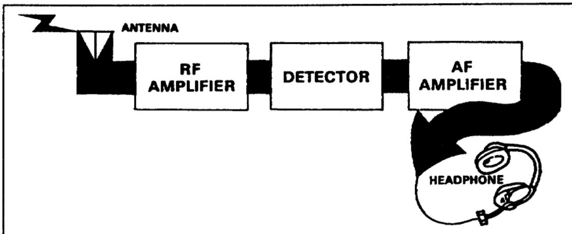
Figure 1-10. Block diagram of a radio receiver
