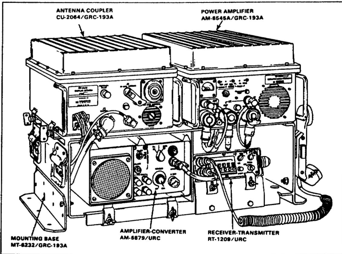
Figure 5-6. Radio set AN/GRC-193A
