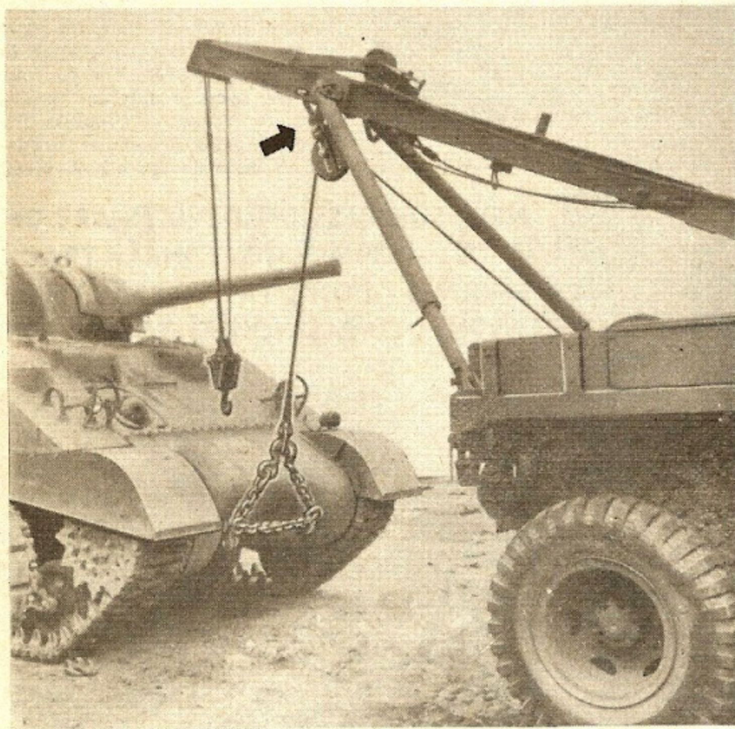
Fig. 3—Here's how the M1 wrecker is set up for the job. First, hang a single snatch block (wrecker equipment) on the boom (arrow). Remove two of the clevises that are part of the heavy snatch blocks (on the wrecker) and install them on the final drive towing lugs. (If they don't fit the lugs, you'll have to dig up clevises big enough to take the chain on the end of the rear winch cable.) Run the chain and hook from the rear winch through the single snatch block you've installed on the boom and through these clevises as shown. The hook on the boom dangles from above waiting for the eye to be installed.
