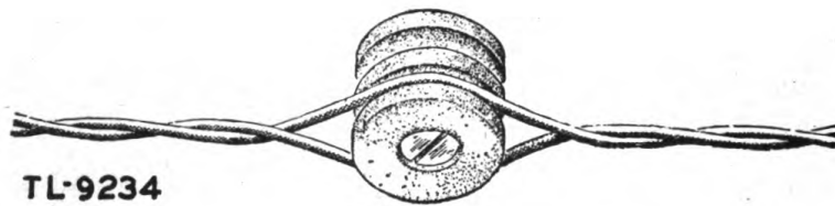
Figure 39. Slipover tie (twisted-pair drop wire).
