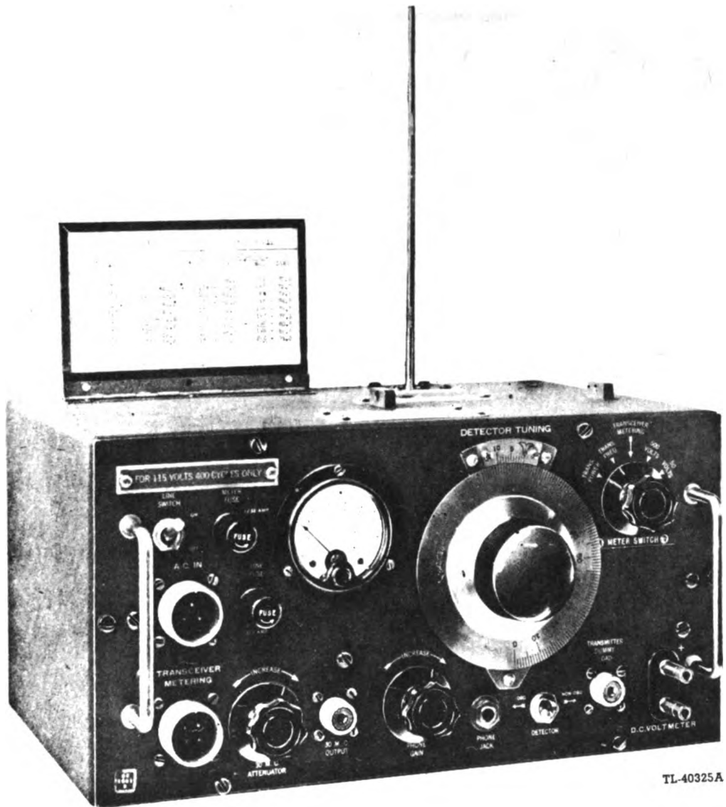
Figure 12. Test Set TS-159/TPX, antenna and tuning chart in operating position.
