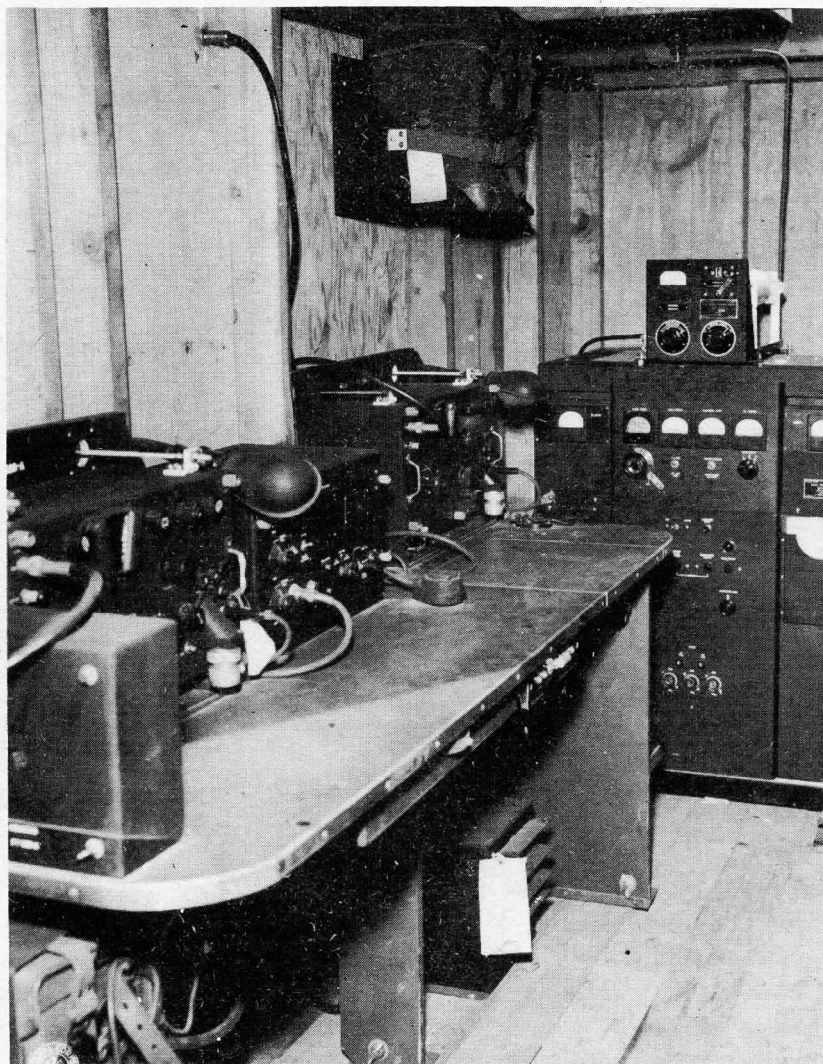
OPERATING POSITION OF THE SCR-299 INSTALLED IN AMPHIBIAN DUKW
