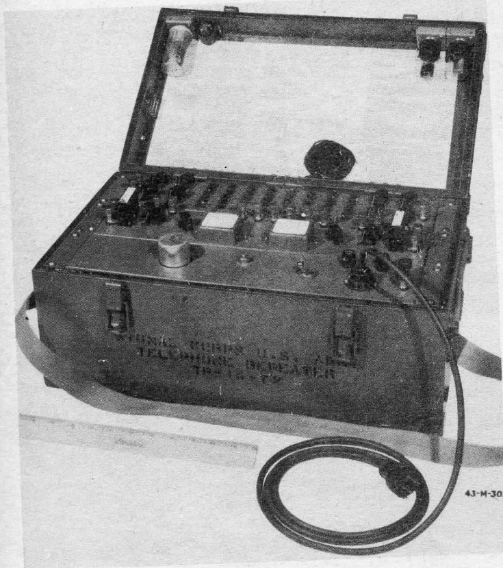
FIG.2- TELEPHONE REPEATER TP-14-T2
