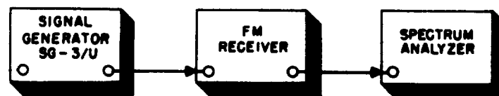
Figure 40. Rf distortion test setup.
