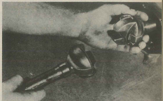
12. There's the complete Tracta joint—unmasked. The outer axle shaft he's holding has the slotted end of the joint still on it. The inner axle and the spigoted half of the Tracta are about to be pulled out of the knuckle.
