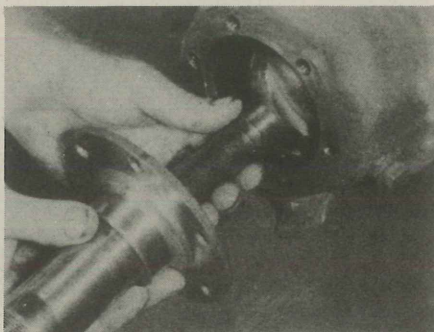
11. Ah-ha, he changed hands. The idea is to reach in and grab the outer axle shaft. If you don't hold on to the axle, it may come tumbling out with half of the Tracta, right into the sand. Now remove the spindle.
