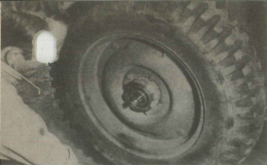
7. Jiggle the wheel lightly to bring the wheel bearing out. Watch it—don't drop the bearing on the ground. Dirt and bits of junk don't mix well with bearings. Now take the wheel off.
