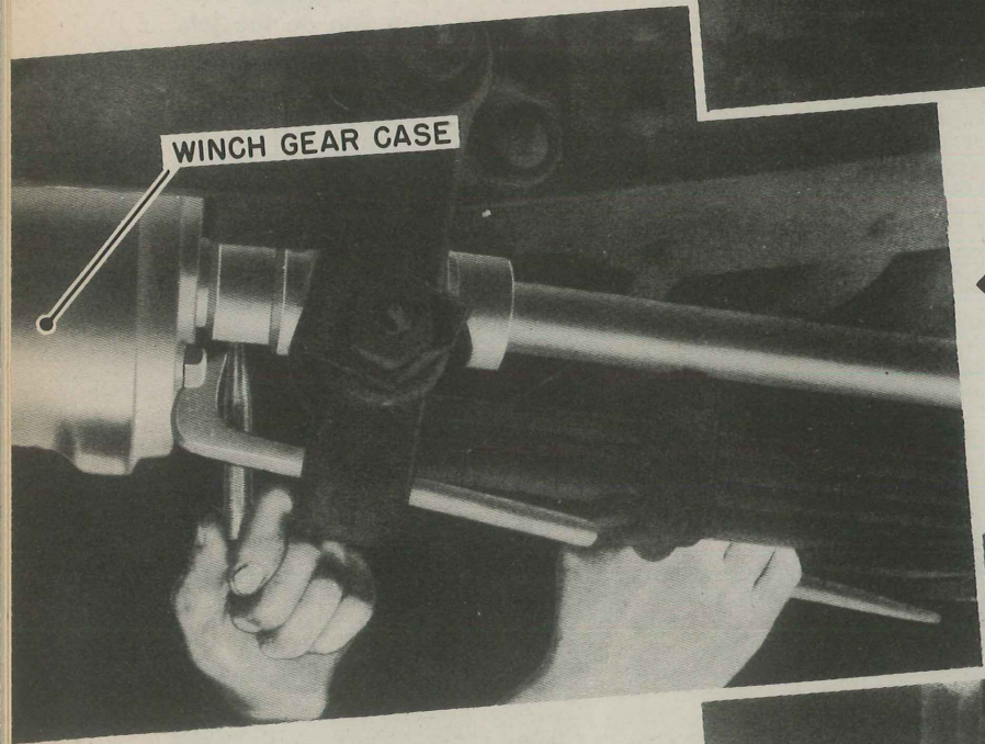
Fig. 9—... pry directly on the shoulder of the universal-joint itself. Then remove the joint from the worm shaft. After cleaning the outside surface of the worm shaft and the inside surface of the universal-joint, smear some Grease General Purpose No. 2 (WB-2) on both before re-installing.
