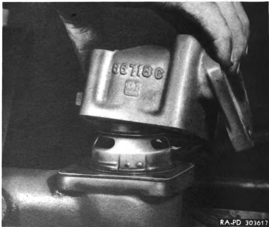
Figure 75—Removing Thermostat Housing
