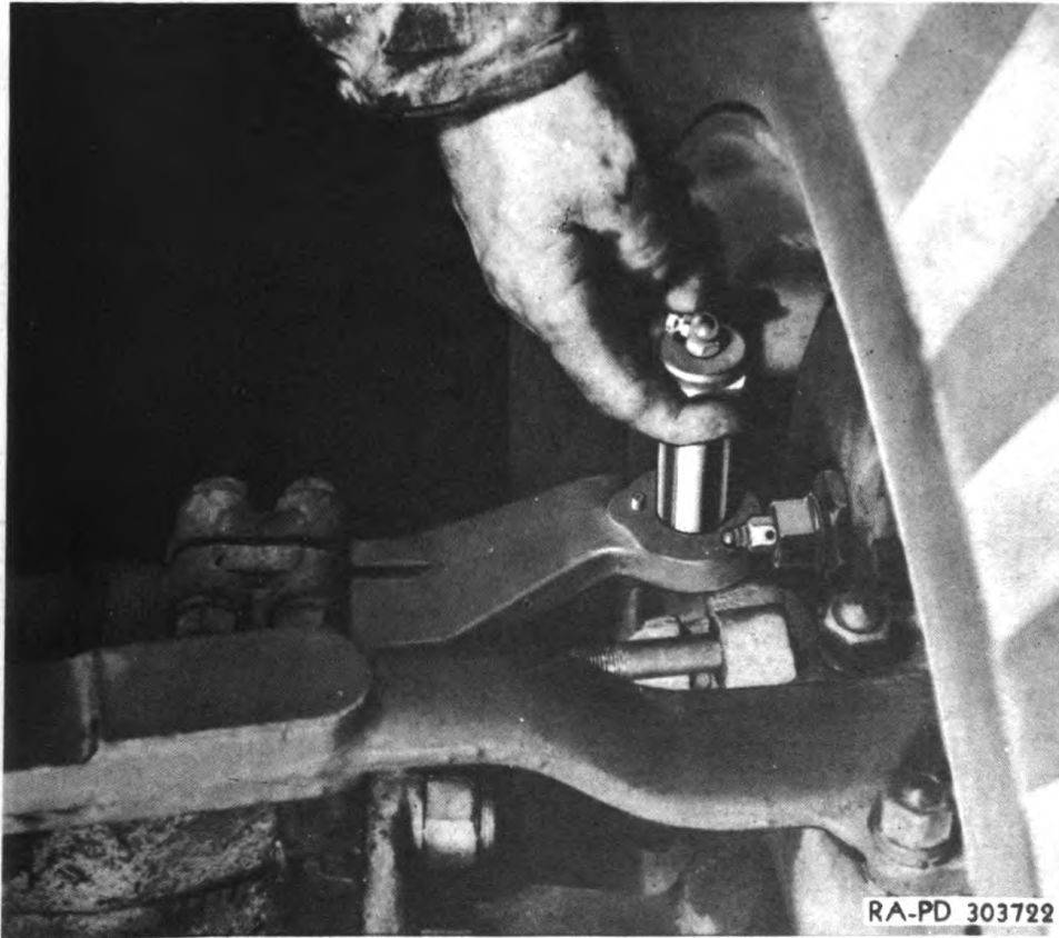
Figure 109—Removing Tie Rod End Pin
