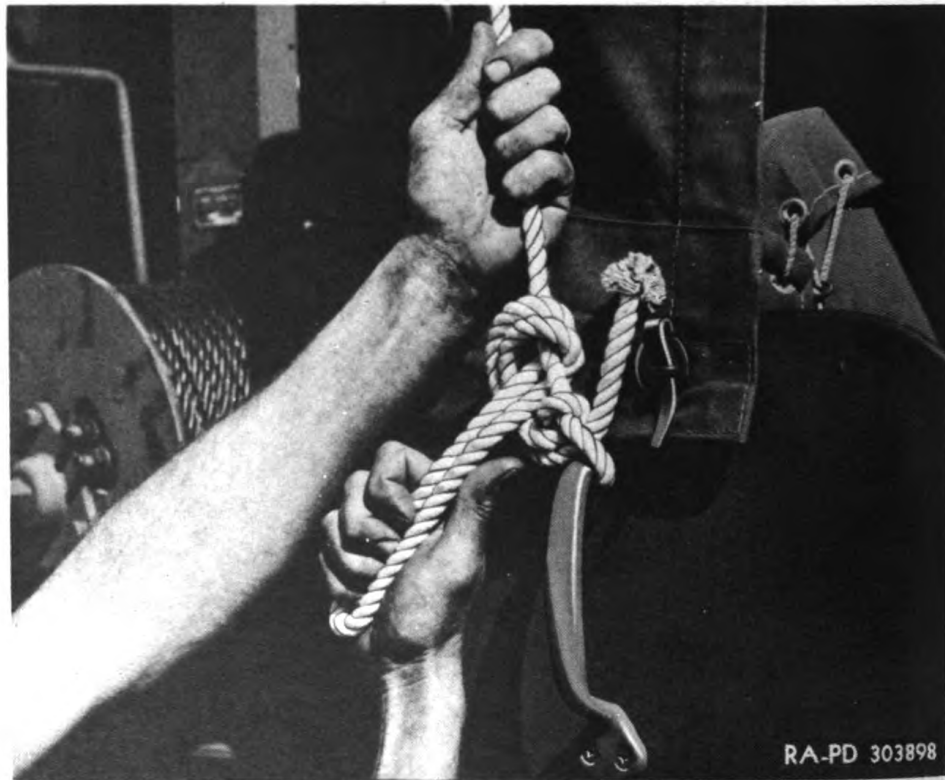
Figure 203—Tying Top Tarpaulin Ropes to Grab Handles
