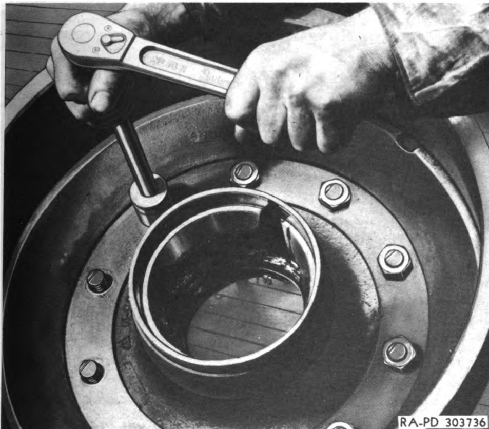
Figure 144—Removing Drum Stud Nuts
