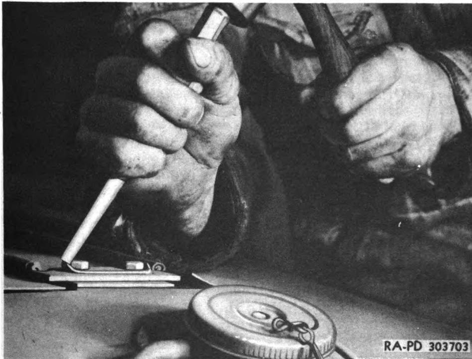
Figure 207—Folding Lock Plate Away From the Hood Center Panel Cap Screws
