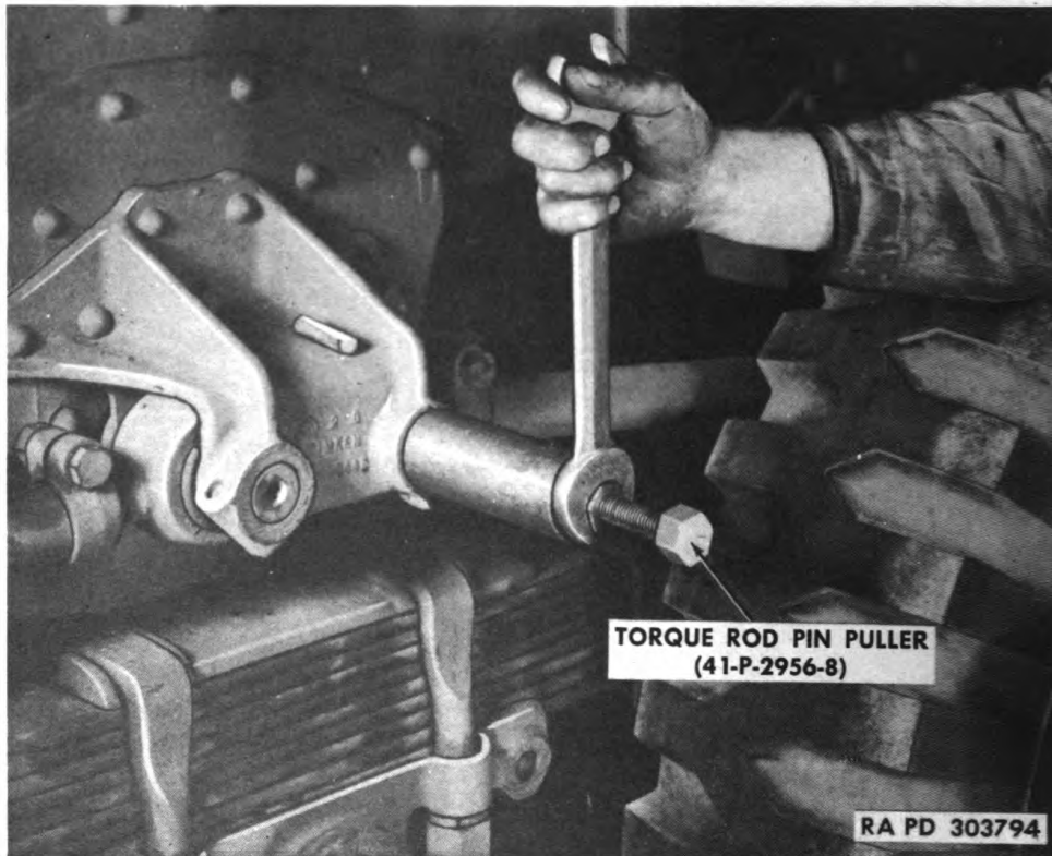
Figure 156—Pulling Upper Torque Rod Center Pin
