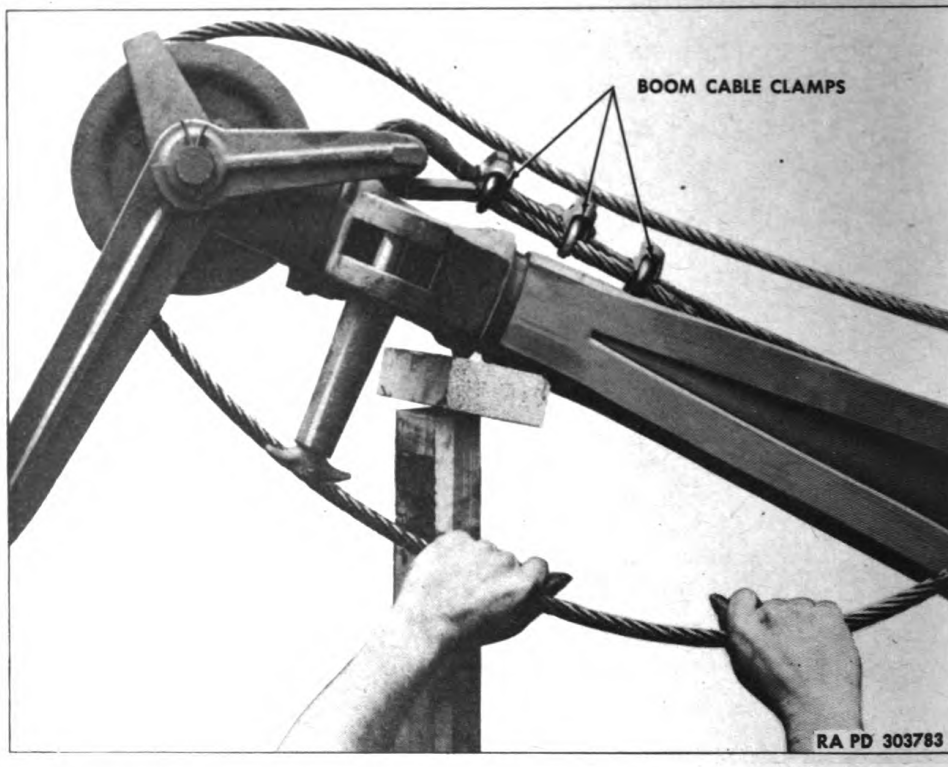
Figure 182—Installing Boom Cable Over Boom Sheave
