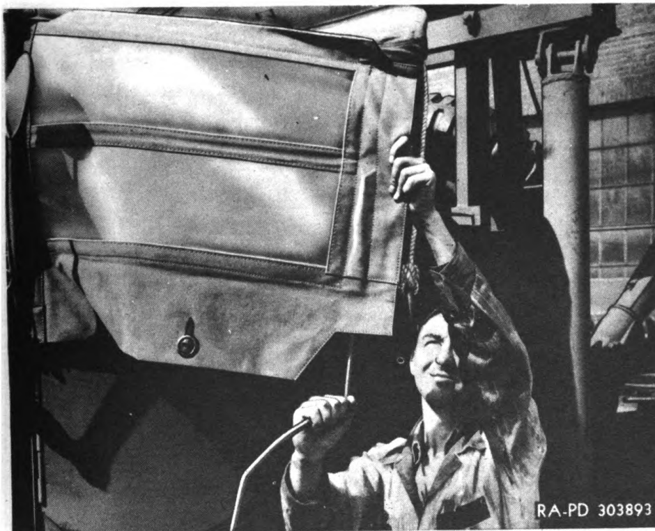
Figure 204—Installing Side Curtain Support Rod
