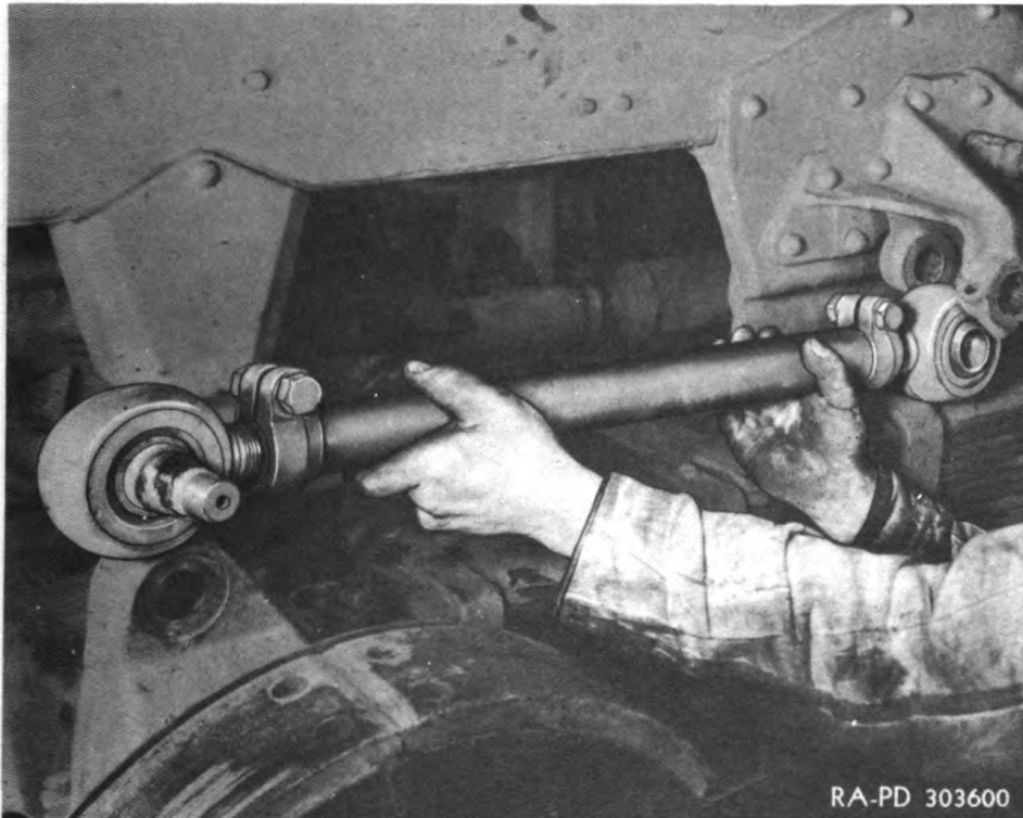
Figure 157—Removing Upper Torque Rod
