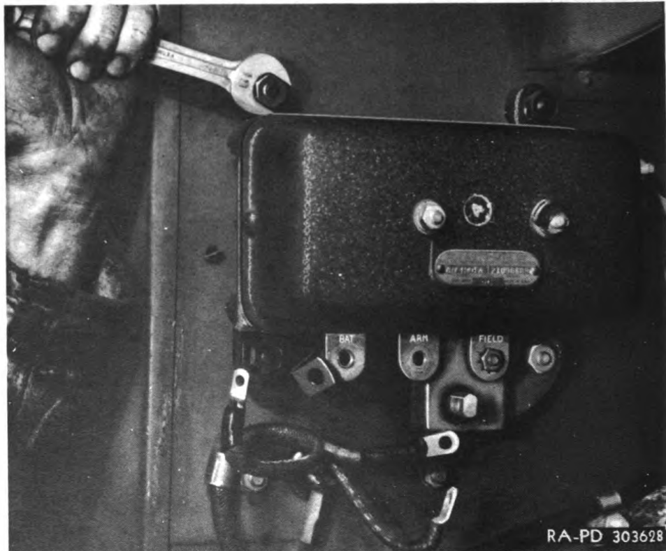
Figure 81—Removing Regulator Mounting Nuts
