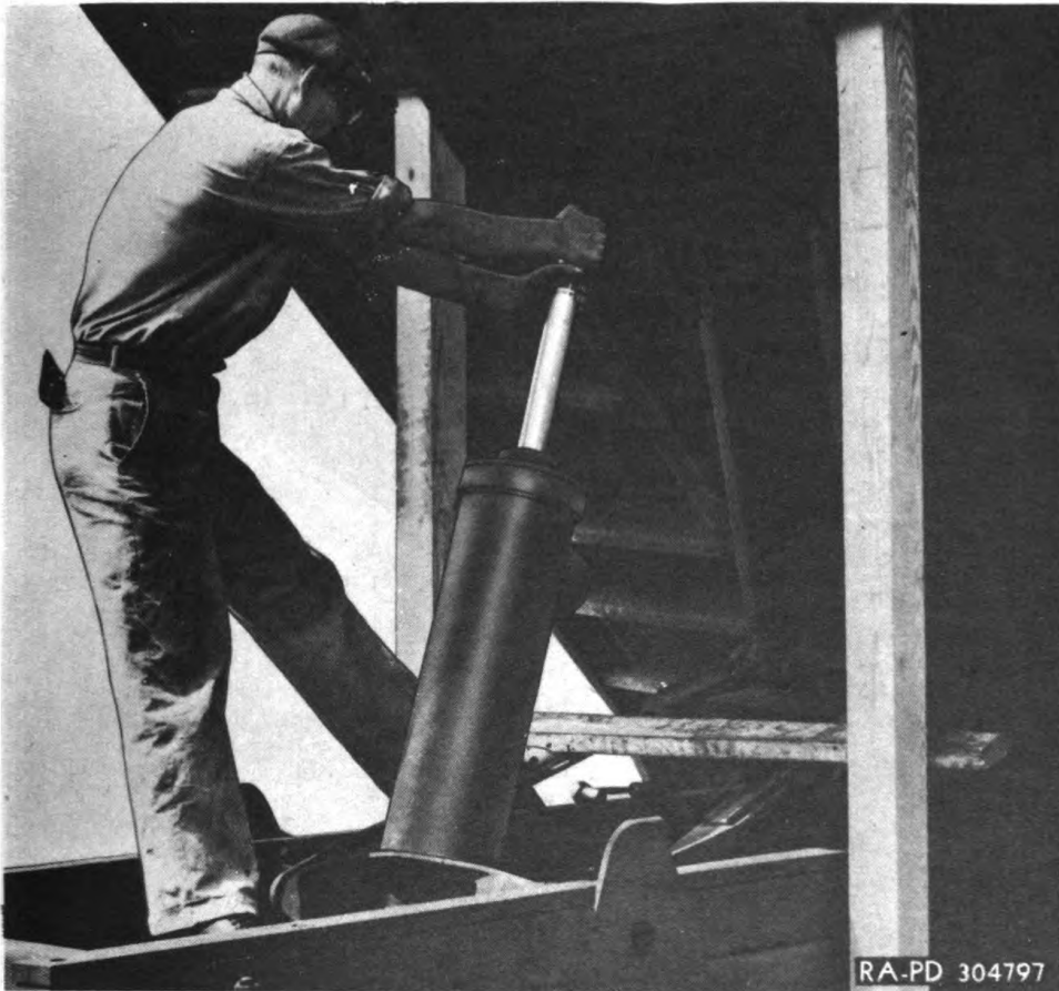
Figure 198—Tipping Hoist Cylinder Back
