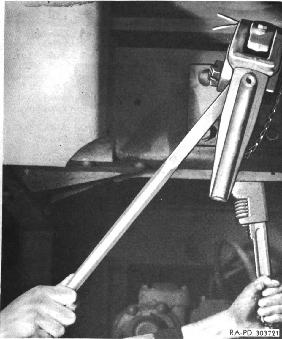
Figure 163—Removing Pintle Hook
