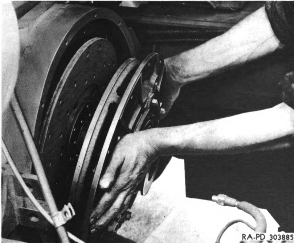
Figure 62—Removing Clutch and Driven Disk
