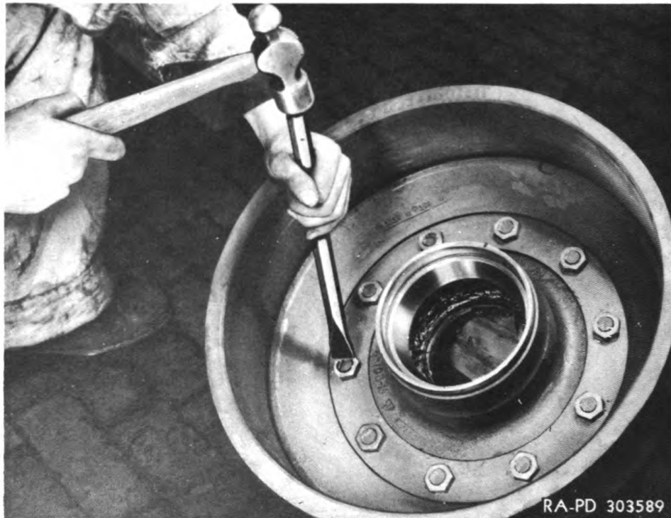
Figure 145—Locking Drum Stud Nuts with Chisel
