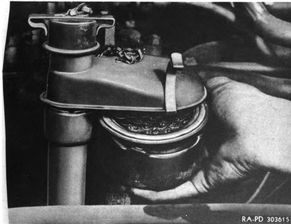
Figure 54—Removing Breather Sump and Mesh
