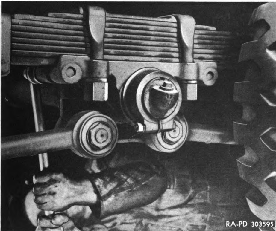
Figure 150—Tightening Spring Seat Clamping Bolts
