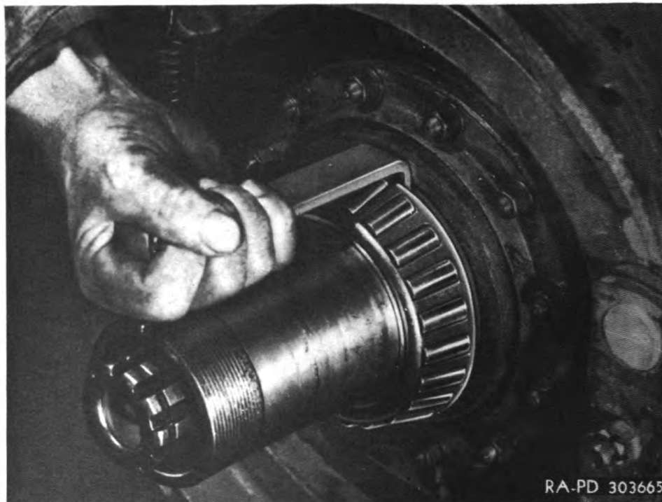
Figure 137—Removing Inner Wheel Bearing Cone
