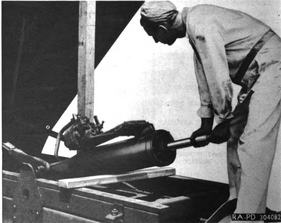
Figure 195—Lifting Hoist Trunnion Out of Frame Sockets
