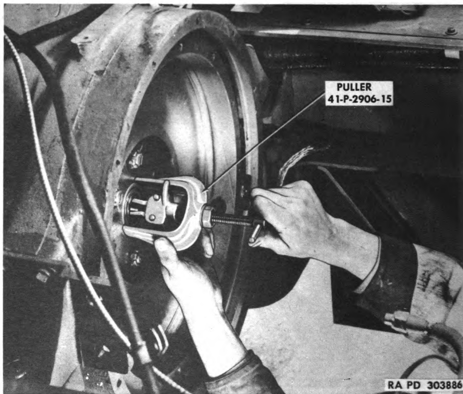
Figure 63—Pulling Clutch Pilot Bearing with Puller 41-P-2906-15
