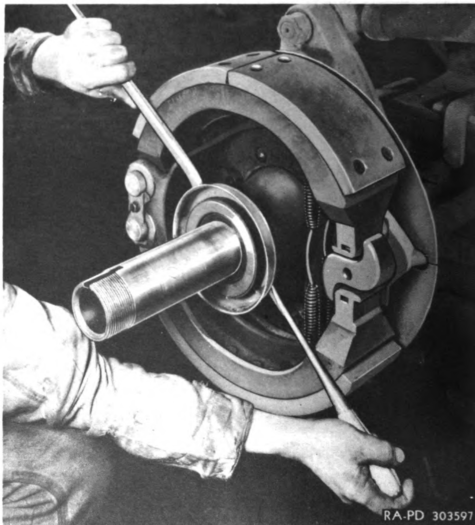
Figure 143—Prying Off Rear Wheel Bearing Grease Retainer
