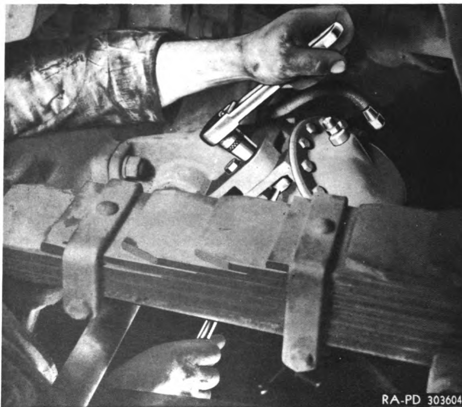
Figure 124—Removing Brake Chamber Mounting Bolts
