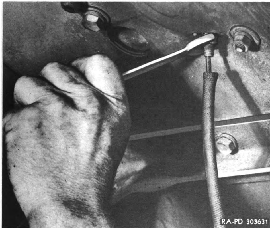
Figure 91—Removing Blackout Marker Light Nut
