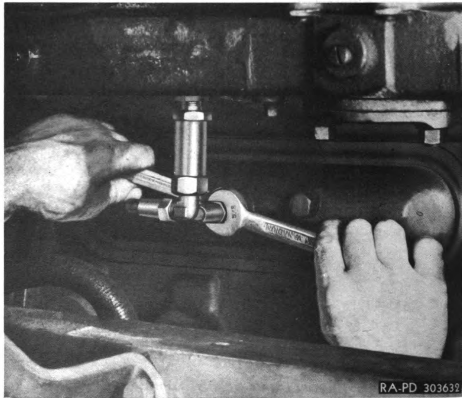
Figure 49—Disconnecting Metering Valve Line
