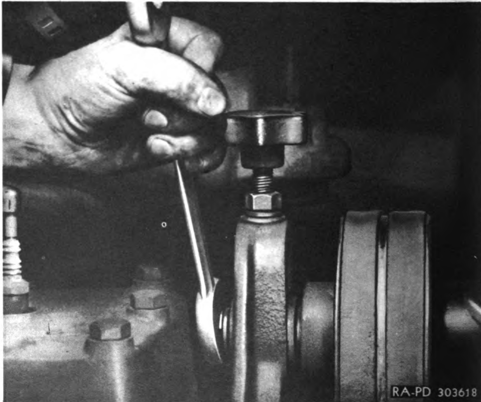
Figure 72—Tightening Fan Spindle Clamp Nut
