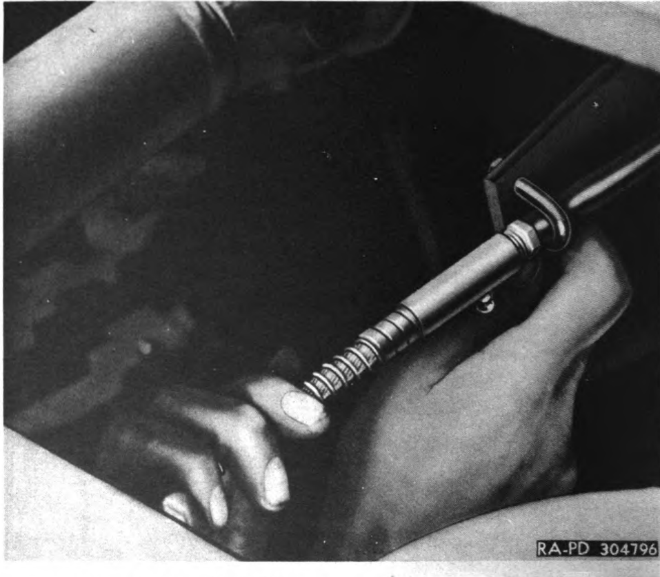
Figure 199—Installing Control Cable Clamp U-Bolt
