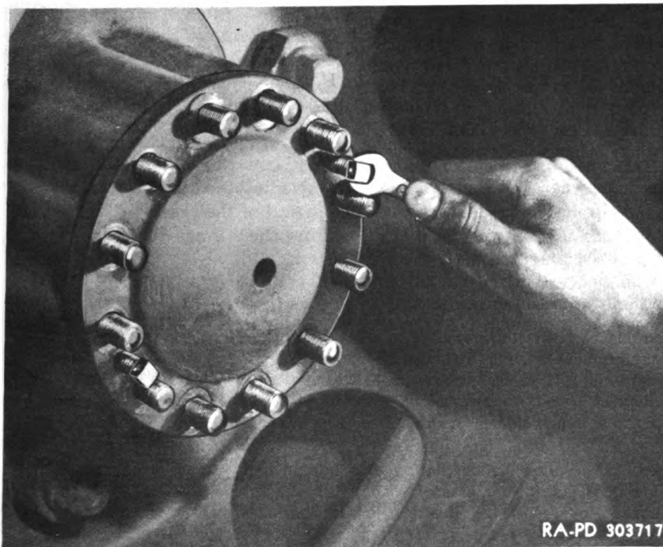
Figure 113—Tightening Rear Axle Flange Puller Screws
