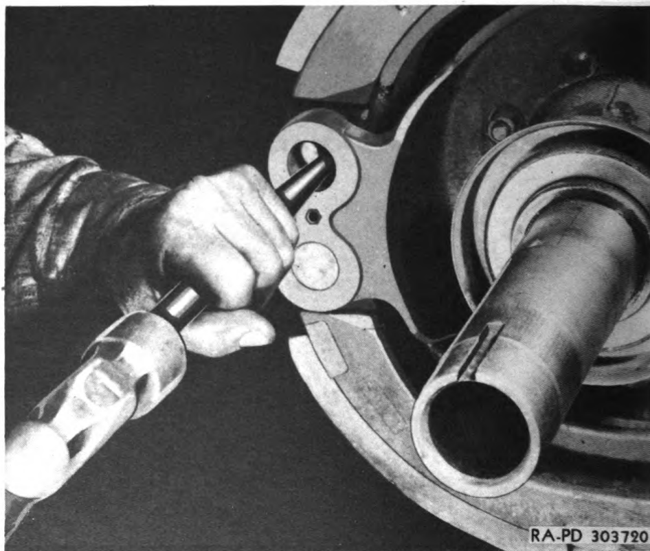
Figure 120—Driving Out Rear Brake Shoe Anchor Pins
