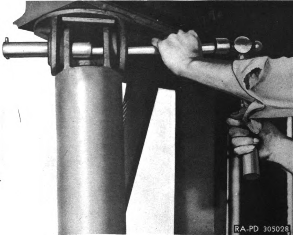
Figure 189—Driving Out Brace Leg Pivot Pin
