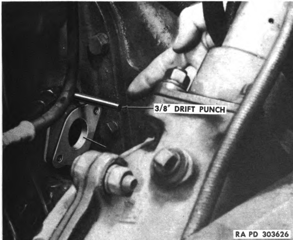
Figure 65—Locating Drive Pin with Drift
