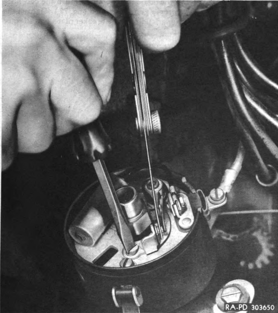
Figure 77—Adjusting Breaker Point Gap to 0.020 inches
