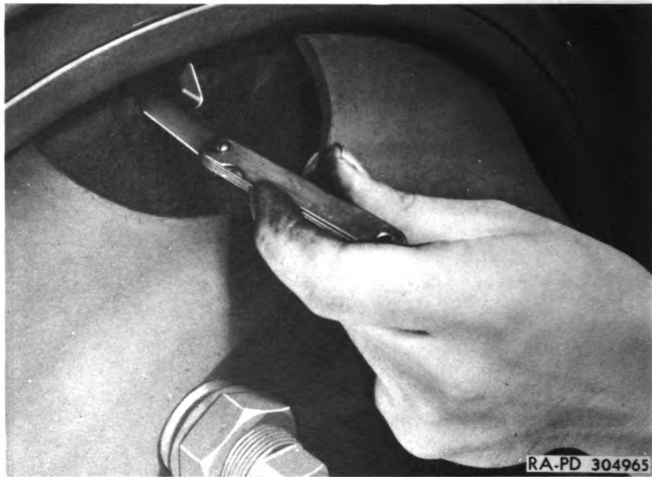
Figure 118—Checking Brake Shoe Clearance (0.010 to 0.015 inch)
