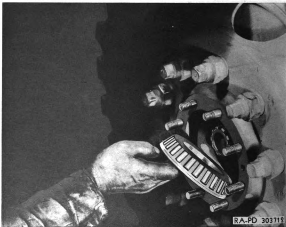
Figure 141—Installing Outer Front Wheel Bearing Cone
