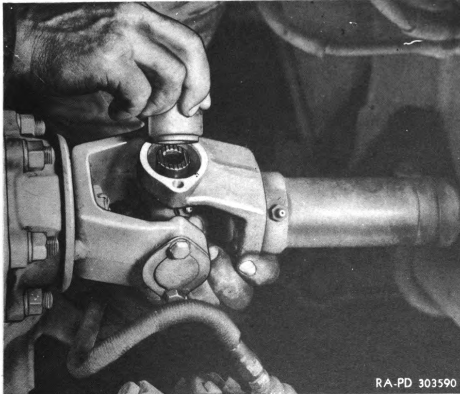
Figure 106—Installing Needle Bearing
