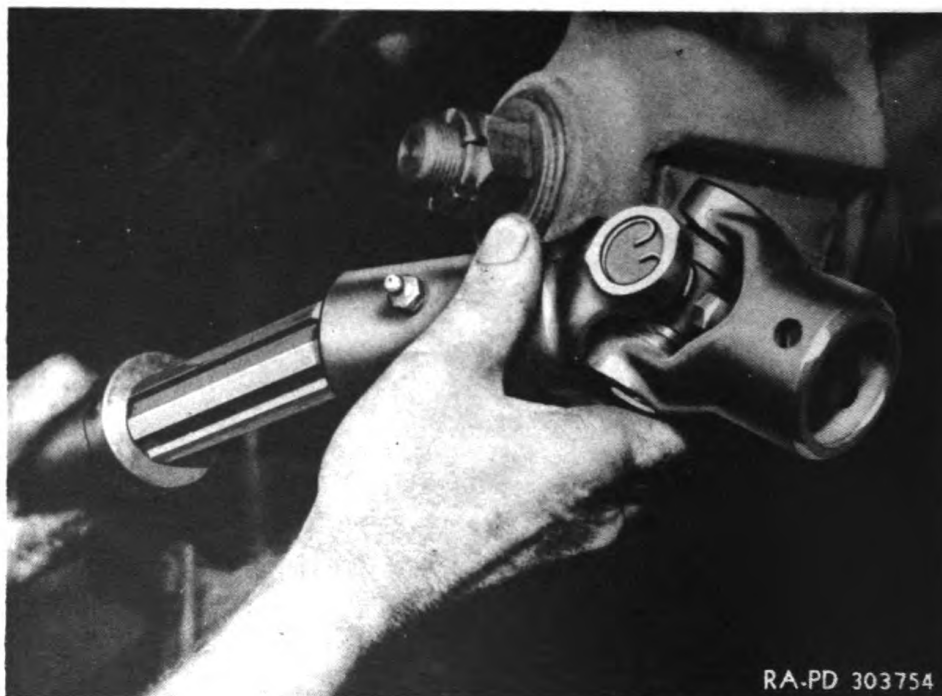
Figure 107—Installing Slip Joint on Winch Propeller Shaft
