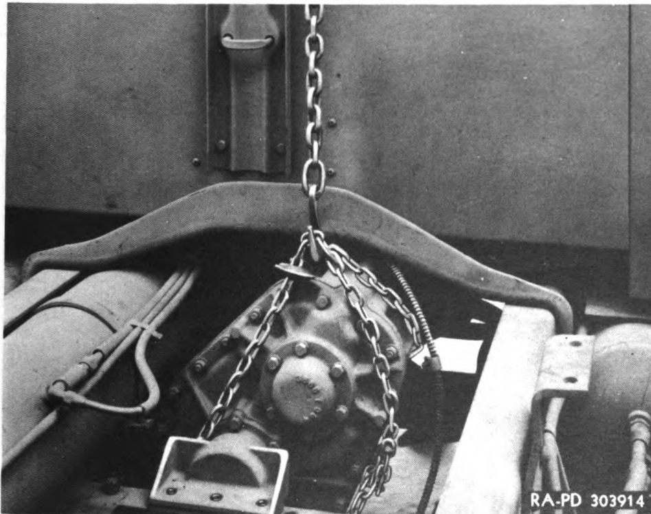
Figure 100—Lifting Transfer on Hoist
