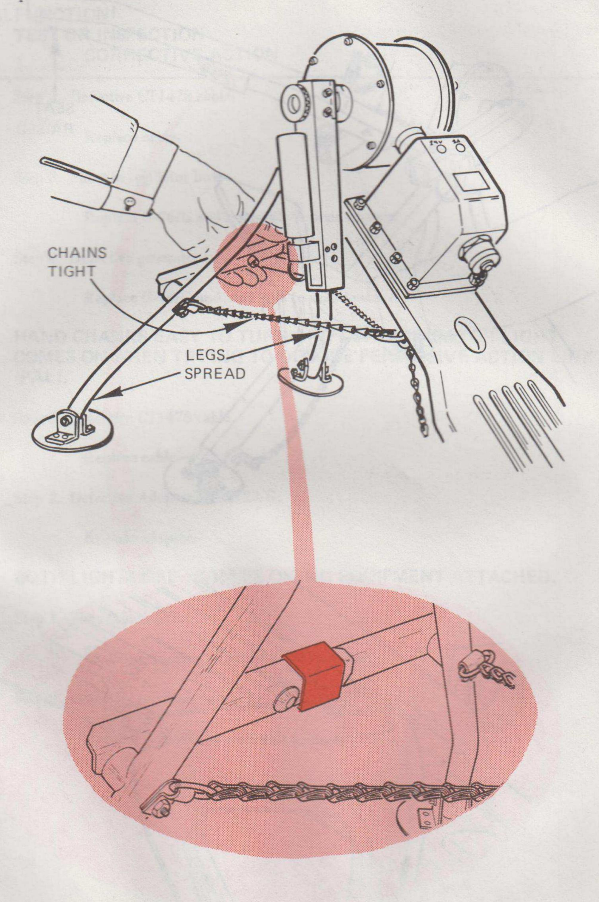
Raise seat away from rear leg and place seat support bracket into the slots under the seat. SEAT RAISED
