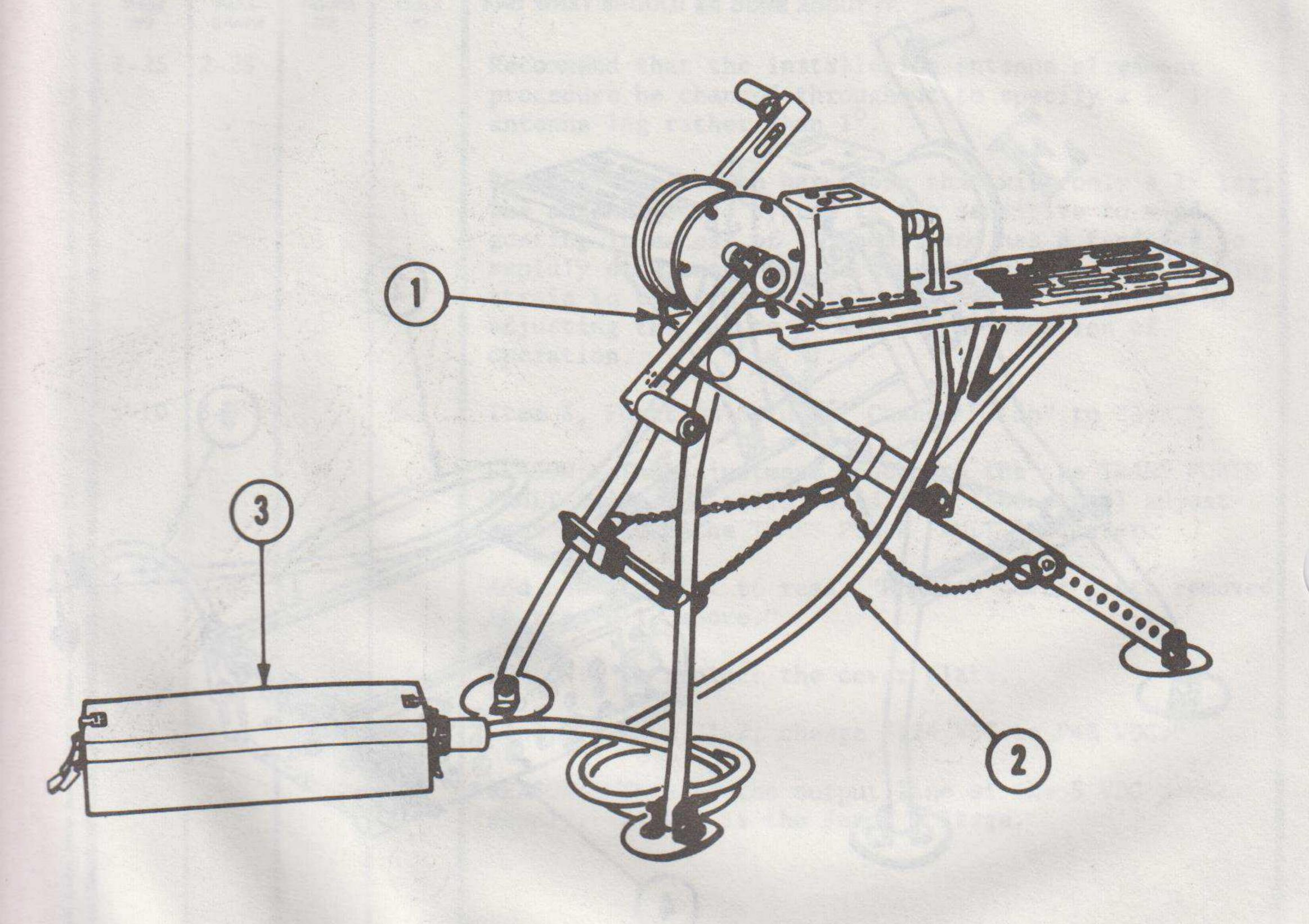
G-76/G (1) Generator Cable CX-13175/G (2) BB-542/U Battery (3)
