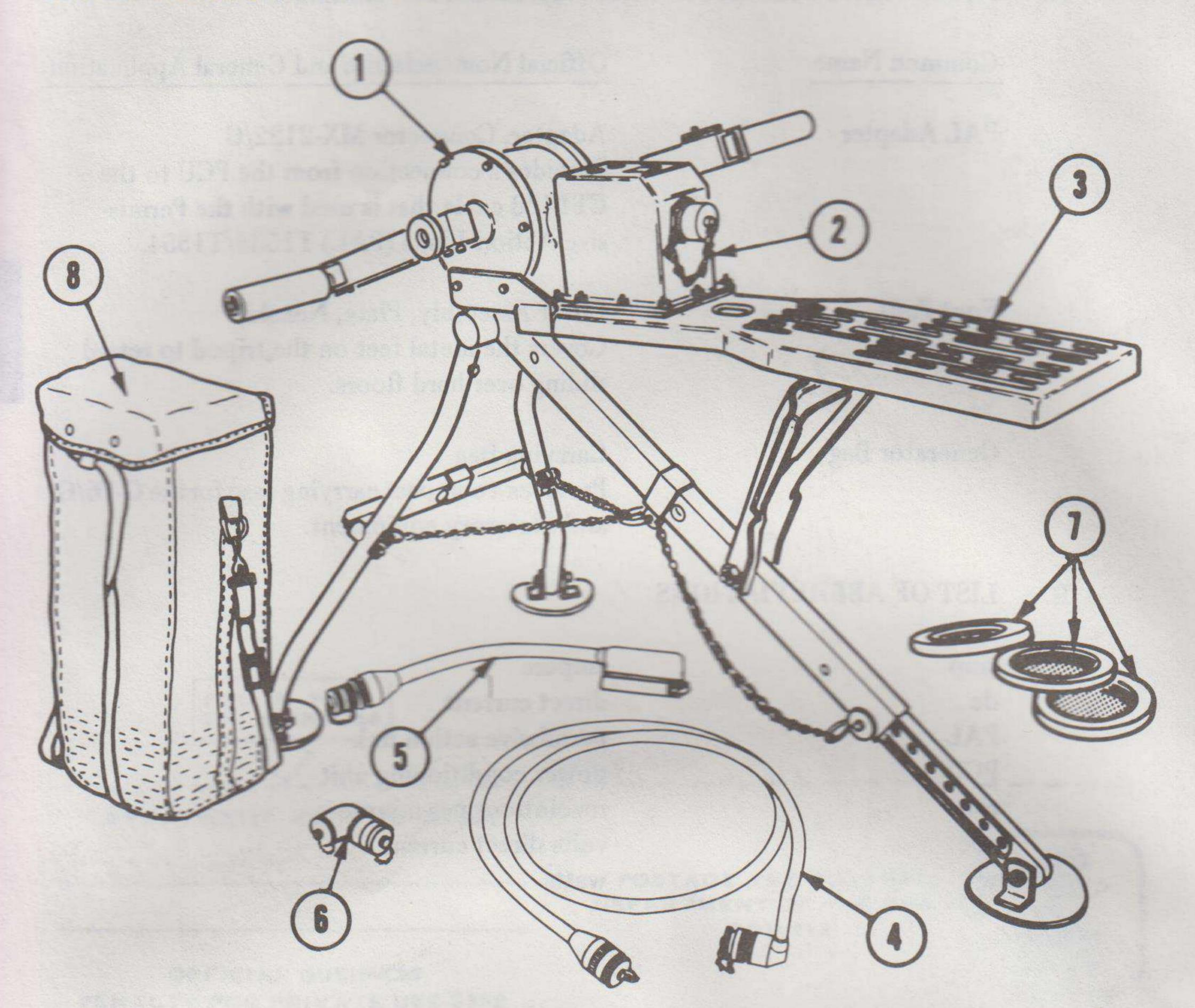
Hand Crank Generator, G-76/G provides power for communications radios, for PAL's and power to charge batteries.
