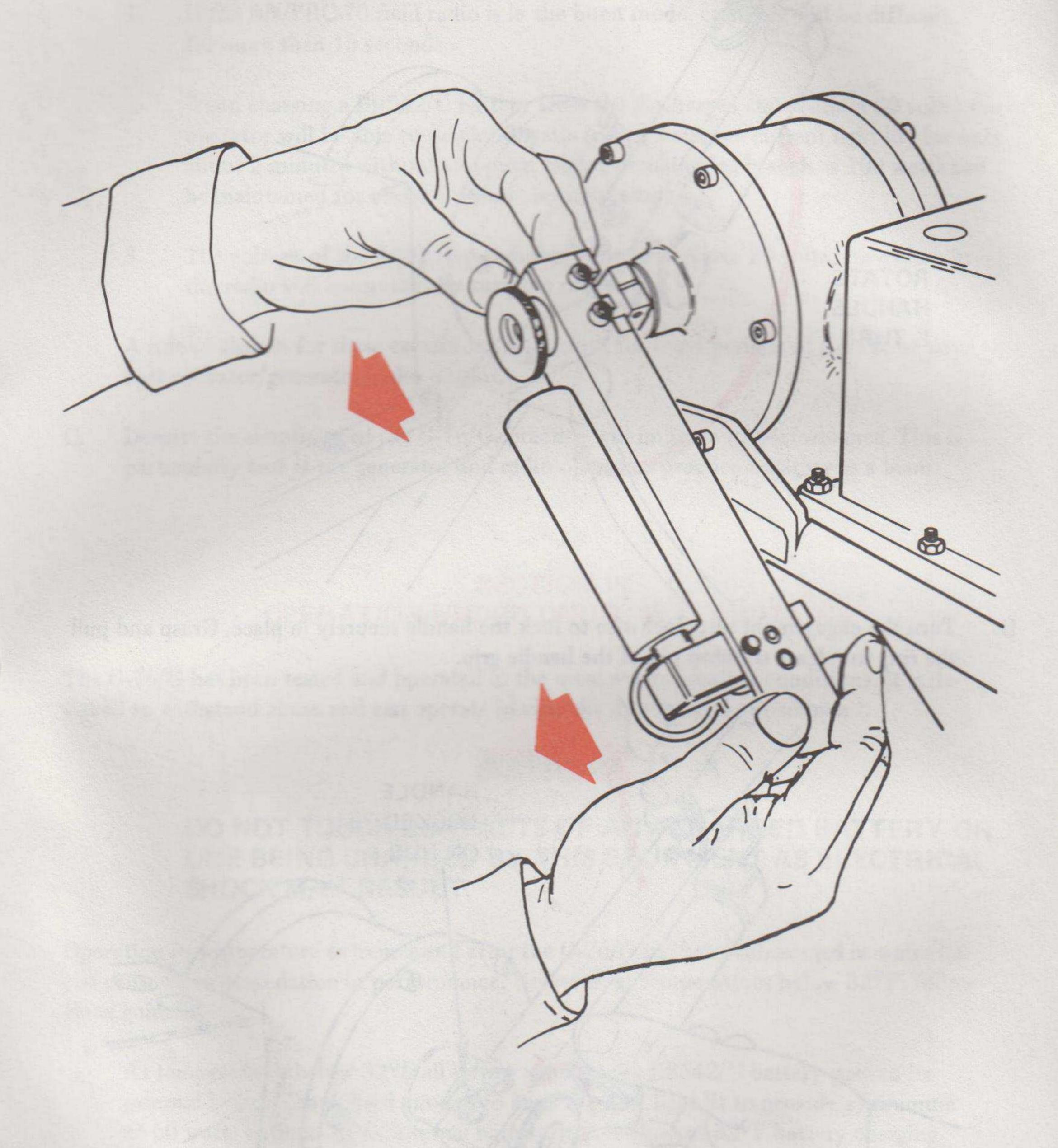
C. Rotate the handle 1/2 turn and push it back into place on the hub.
