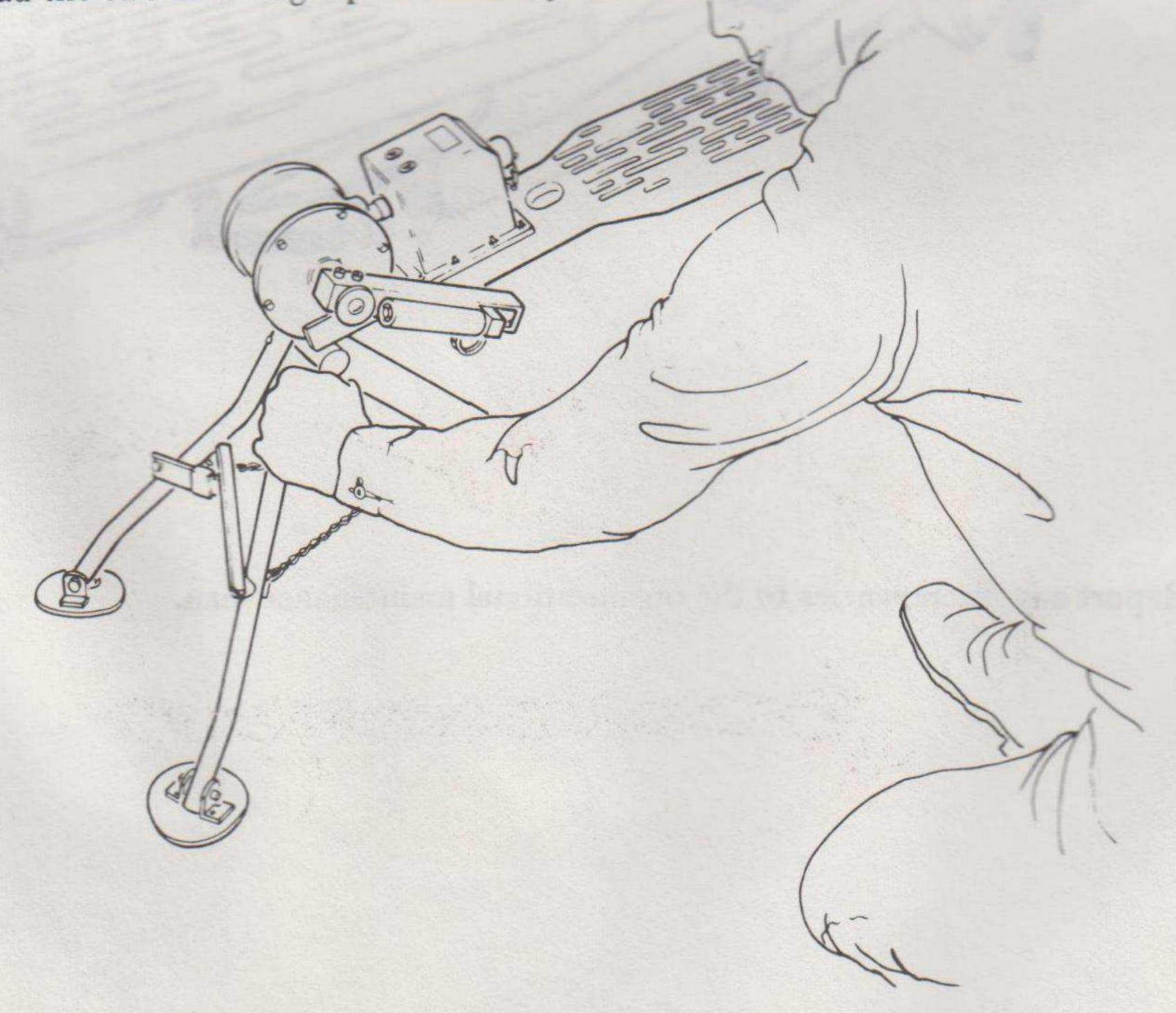
D. Lock the brace for the front legs in the open position by sliding the lock over the pivot point in the brace.
