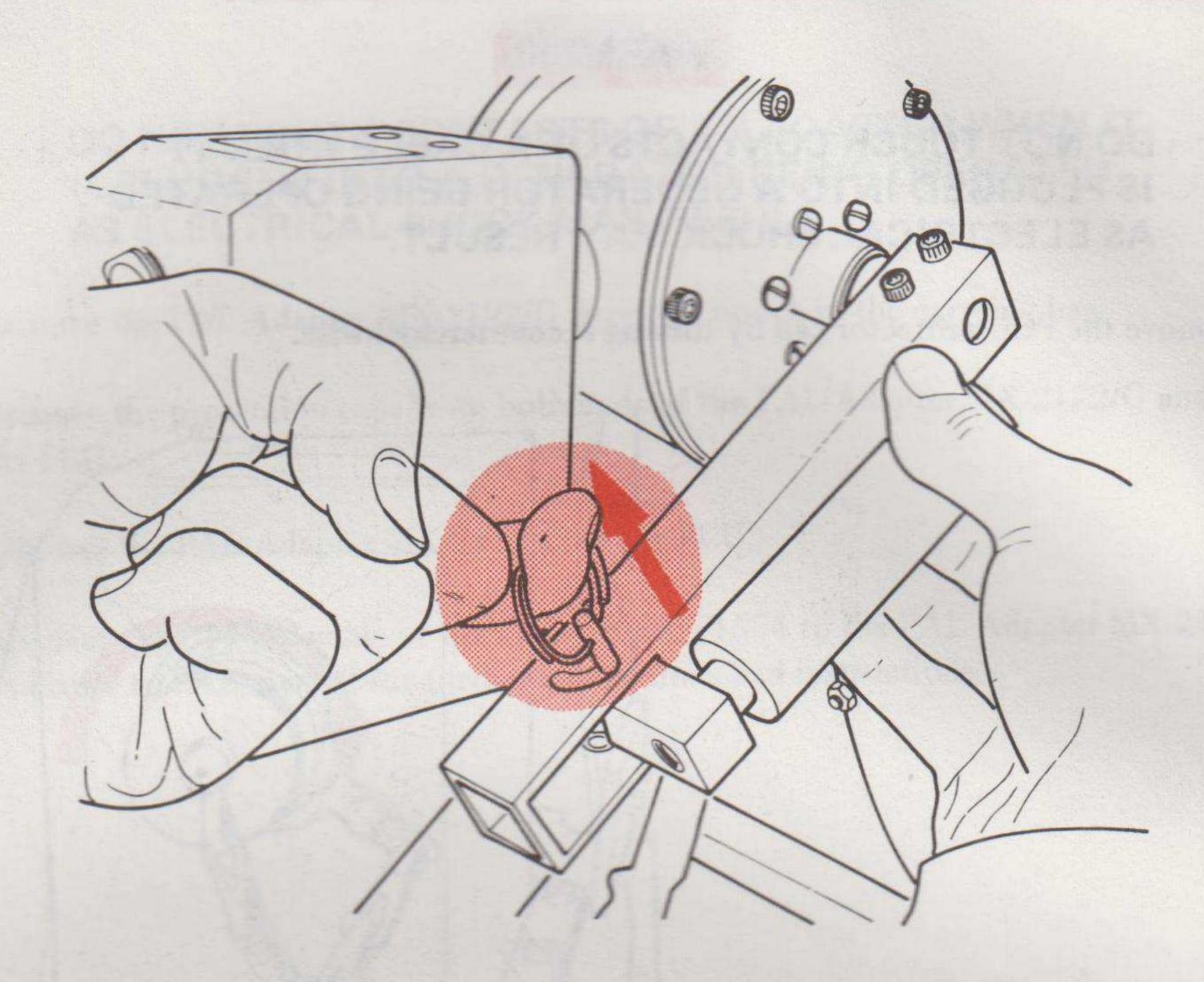
B. Swing the plastic handle grip away from the handle arm to form an L shape. The right and left handles are now in the open and ready position.
