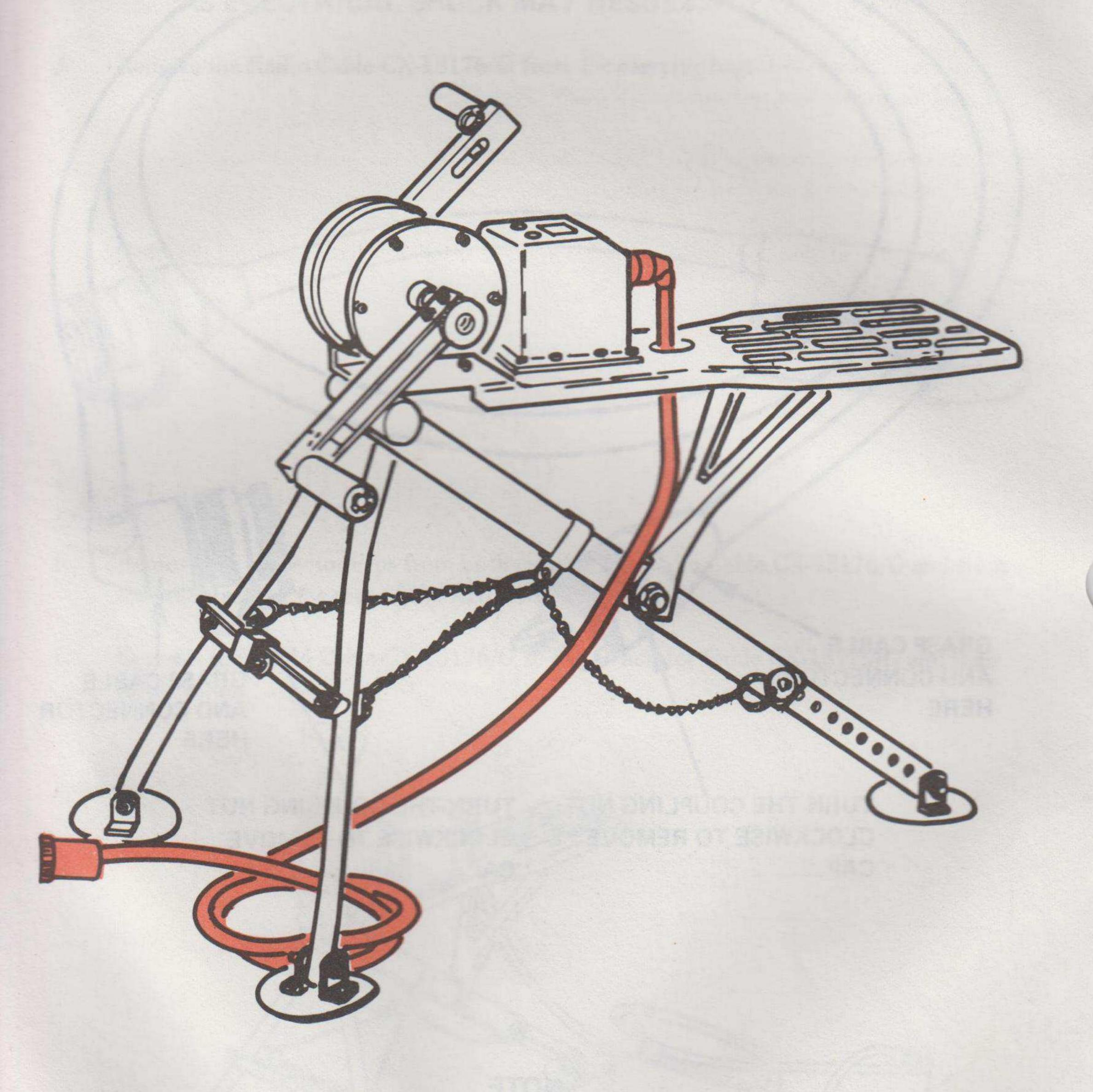
D. Remove the protector cap and connect the cable to the PCU being careful to align the keyways to prevent connector damage.
