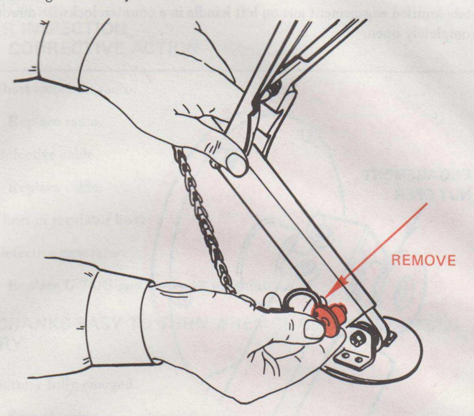
G. When the desired length is reached, lock the leg extension with the stop pin in place.
