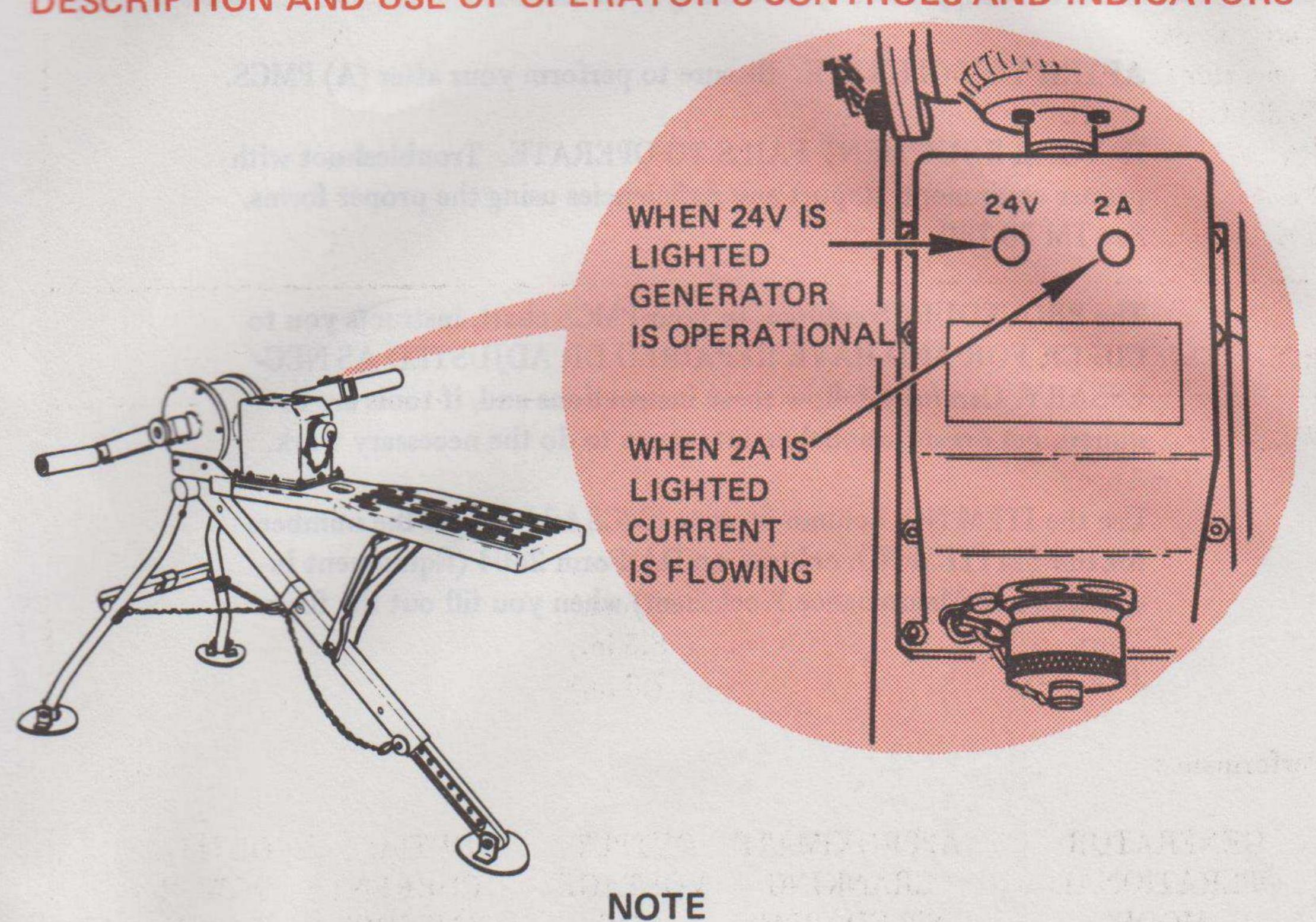
Do not operate the G-76/G until you understand the operation and function of the indicators.
