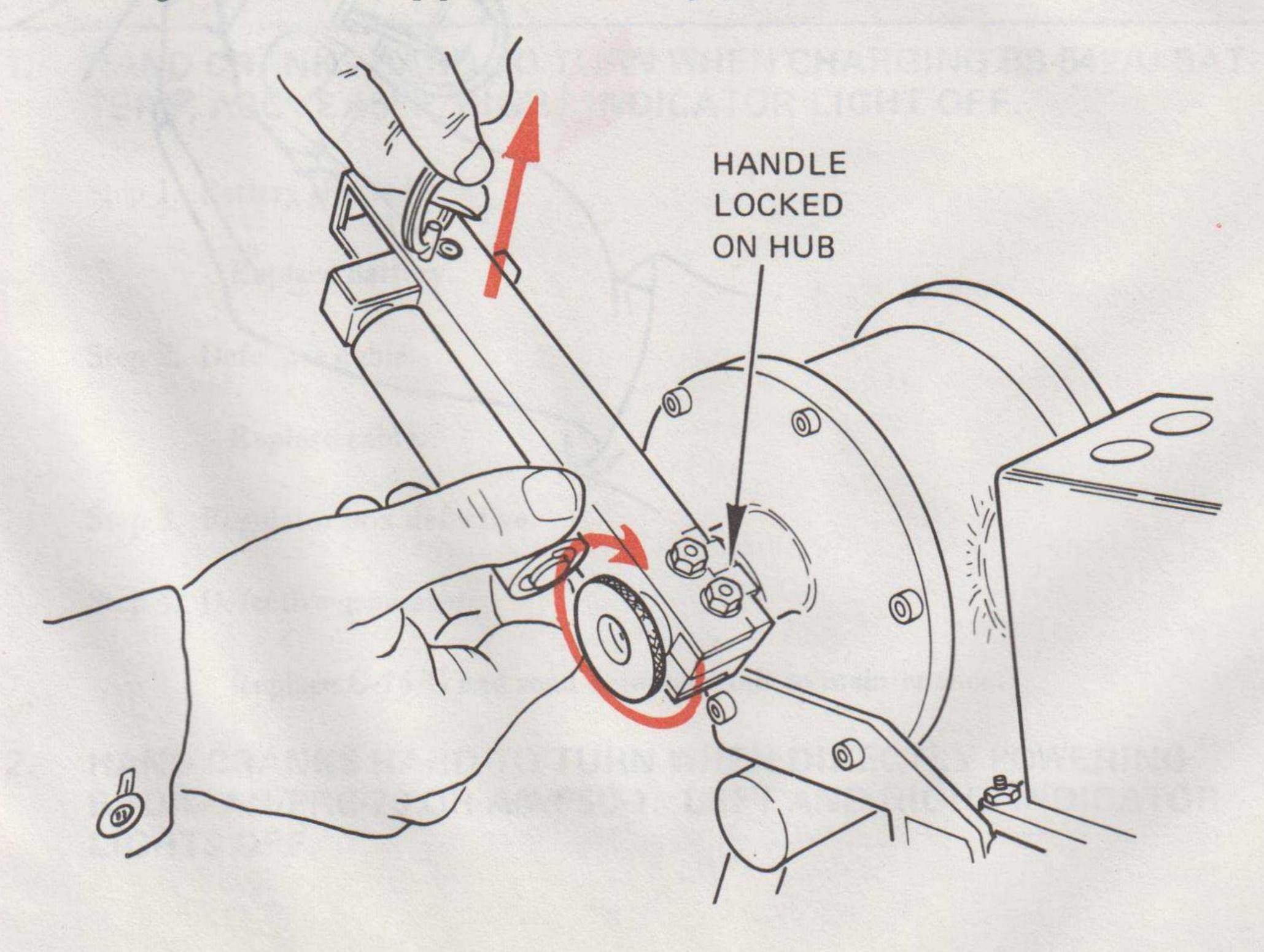
E. Swing the plastic grip away from the handle arm to form an L shape in the open and ready position and release the stop pin.
