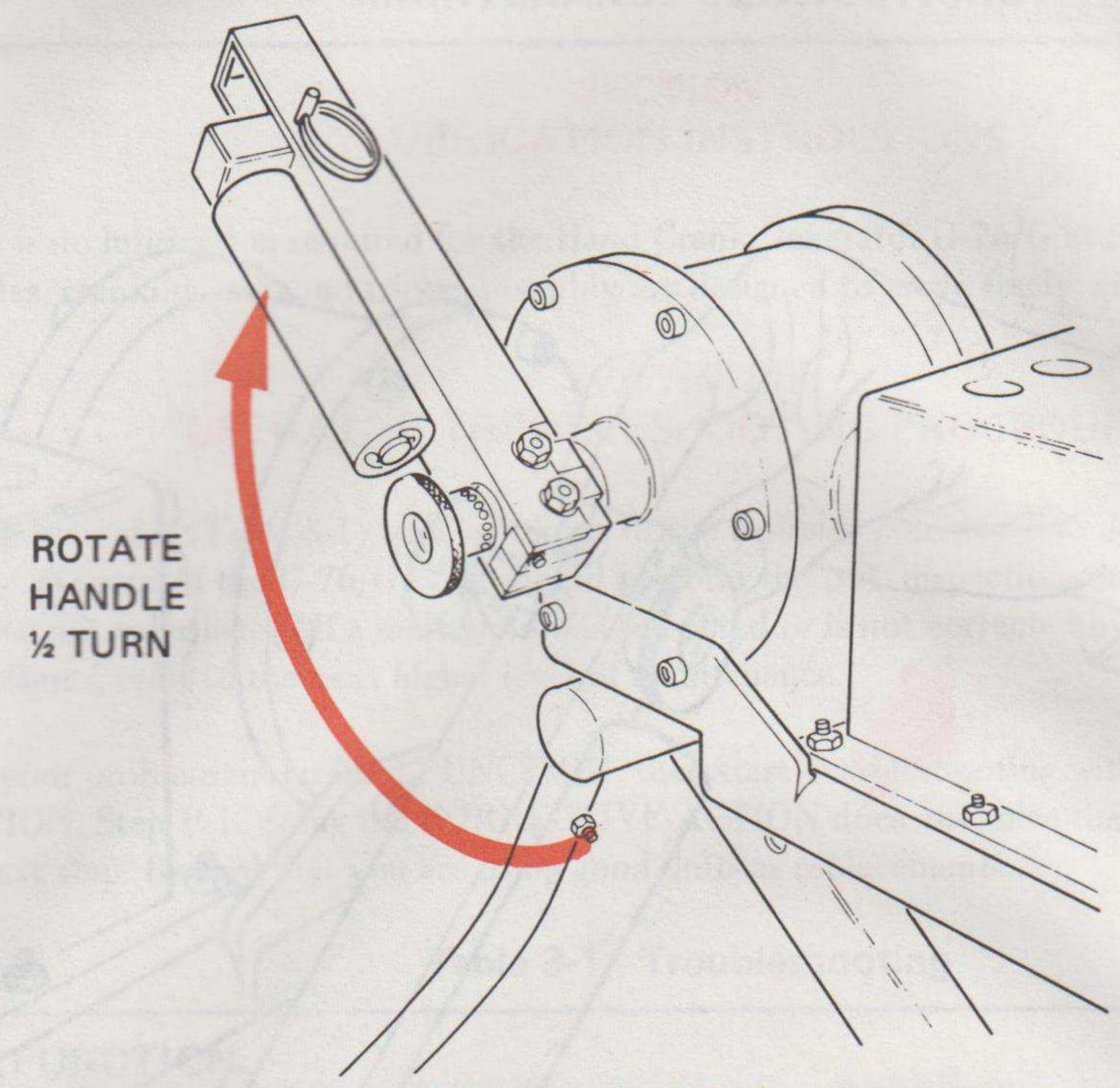
D. Turn the engagement nut clockwise to lock the handle securely in place. Grasp and pull the ring to release the stop pin of the handle grip.
