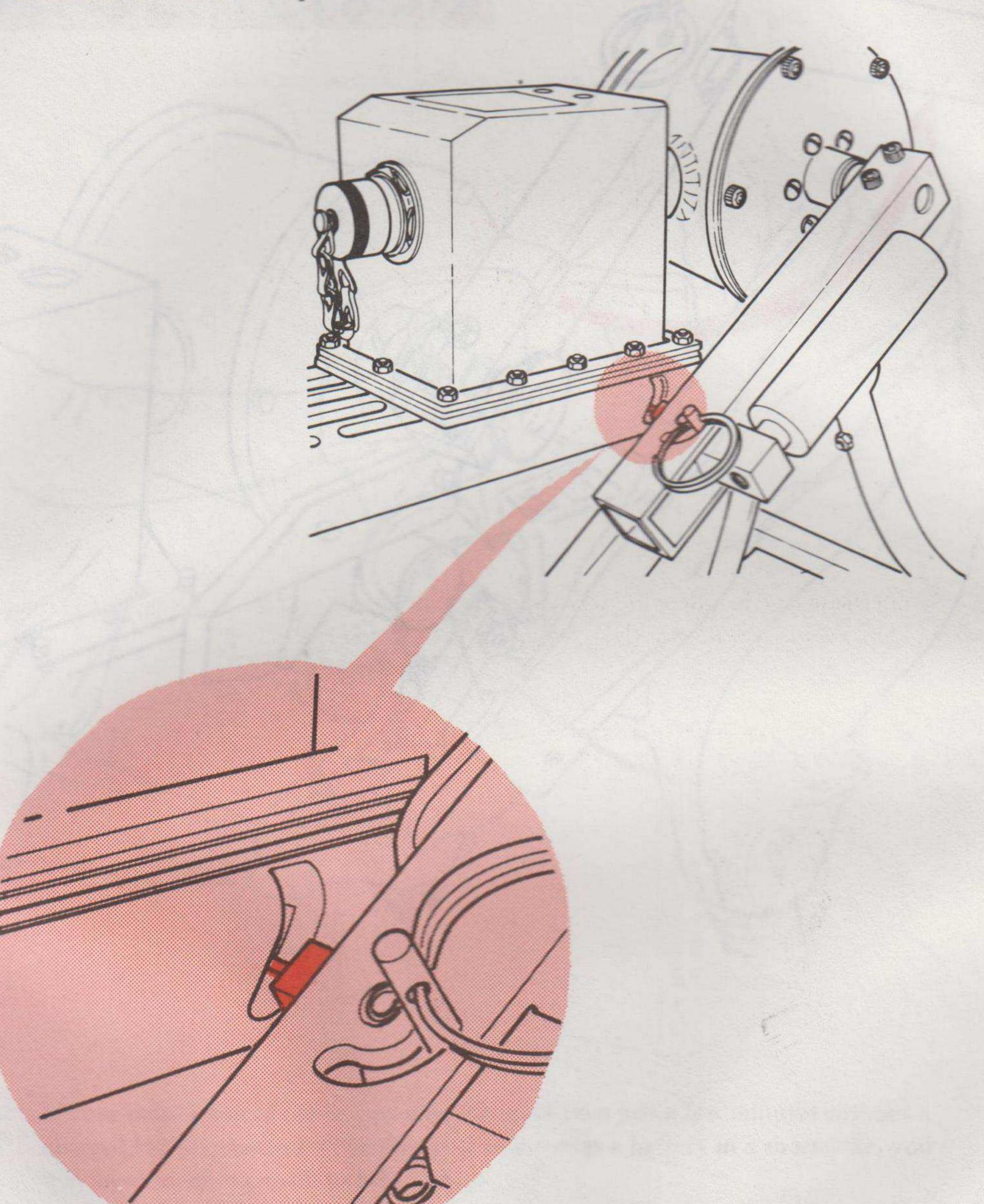
A. Grasp and pull the ring to release the stop pin of the handle grip.
