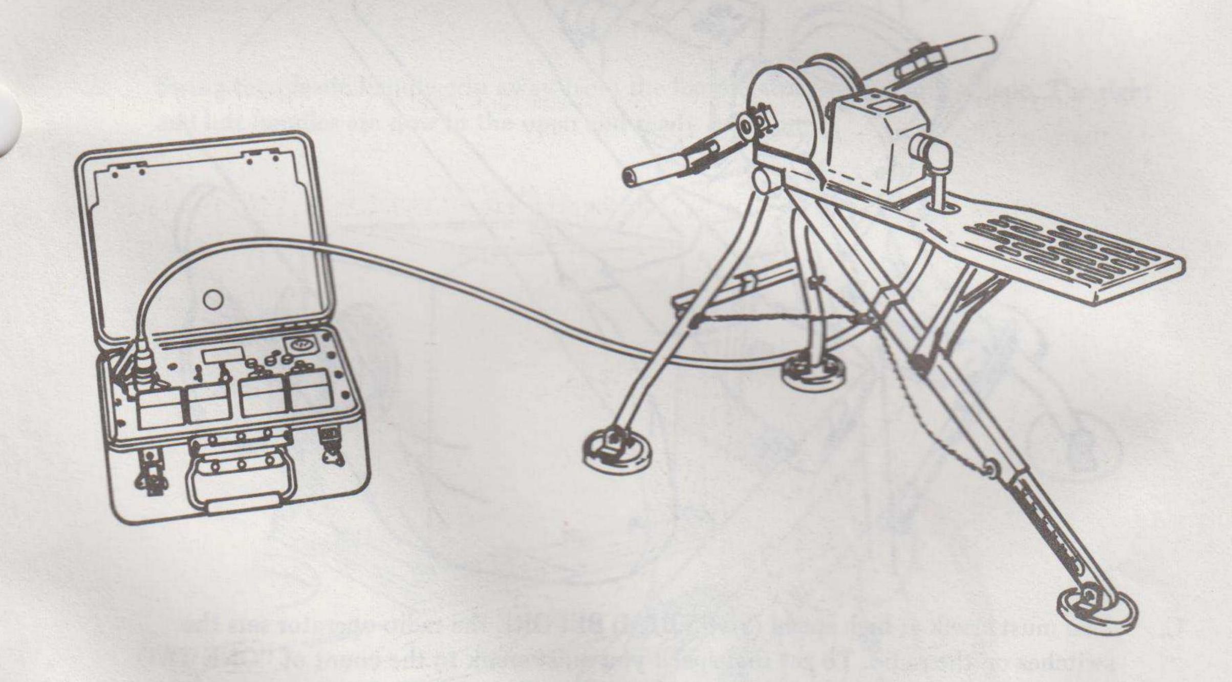
E. Install the three foot pads on the feet of the tripod.
