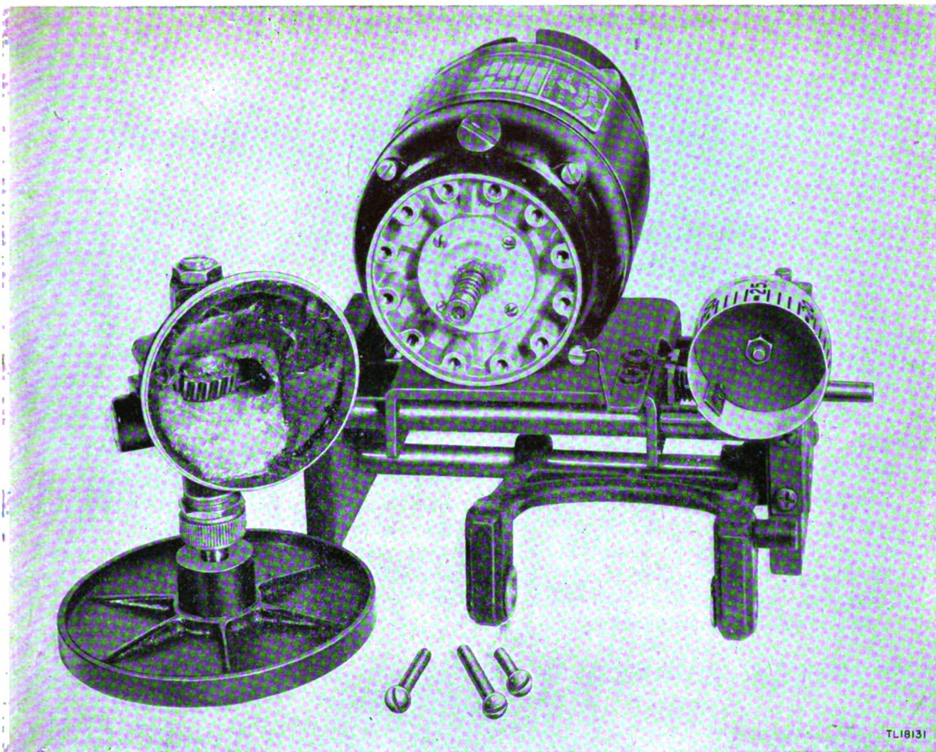
Figure 15. Motor drive assembly with gear housing removed.
