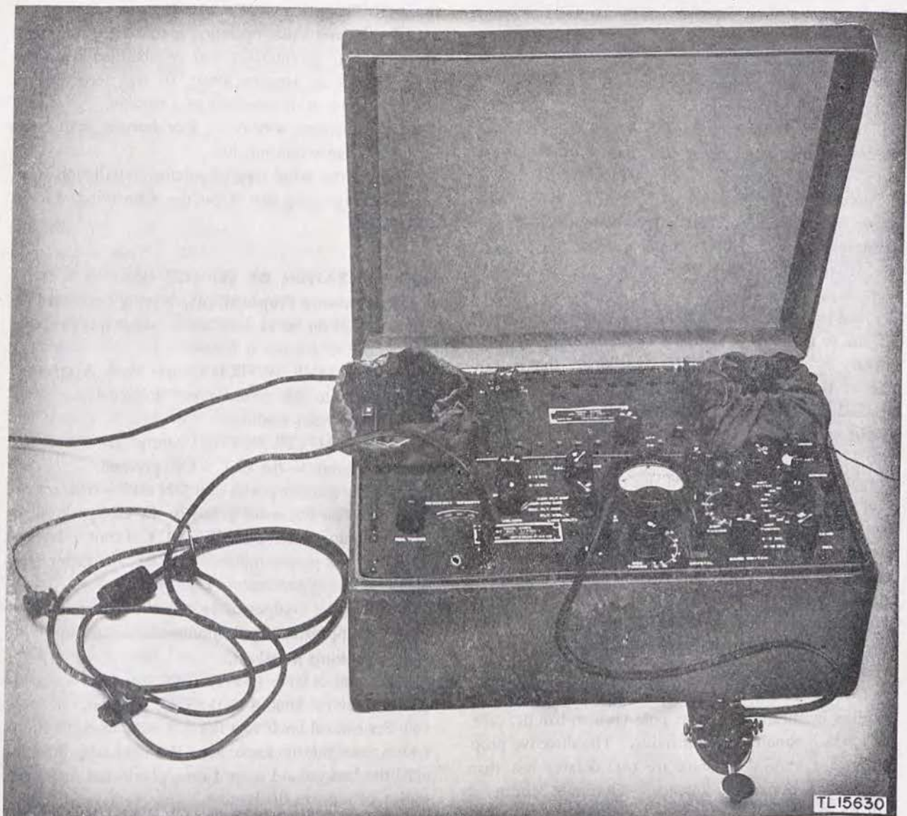
Figure 10. Radio Set AN/PRC-1 ( ) installed for operation.
