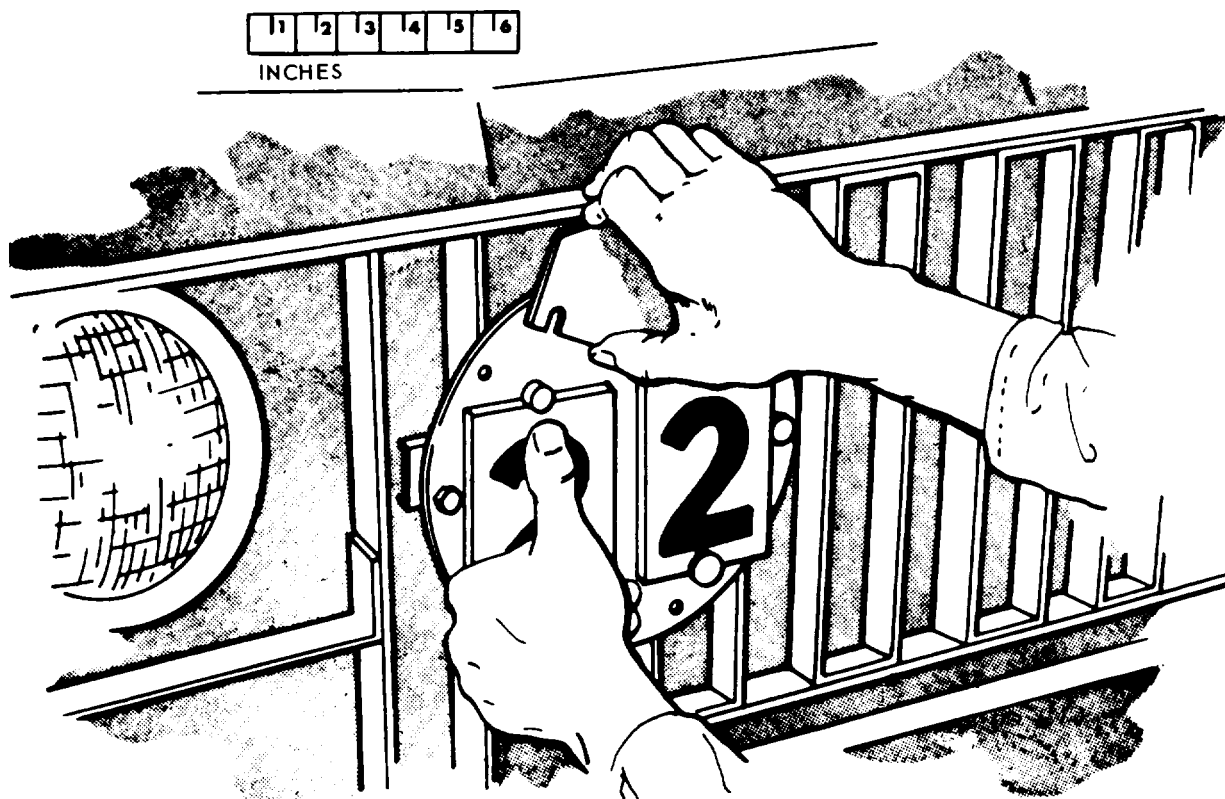
Figure 2-8. Unlocking the retaining plate.
