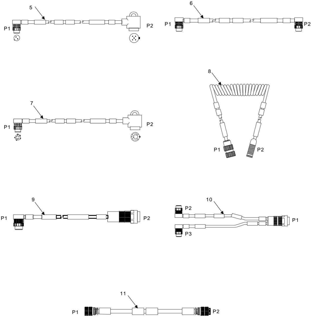
Figure 2-2. Illustrated Parts List - Cables
