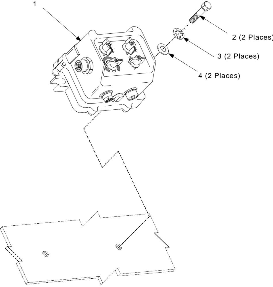
Figure 4-7. Driver's FFCS Installation
