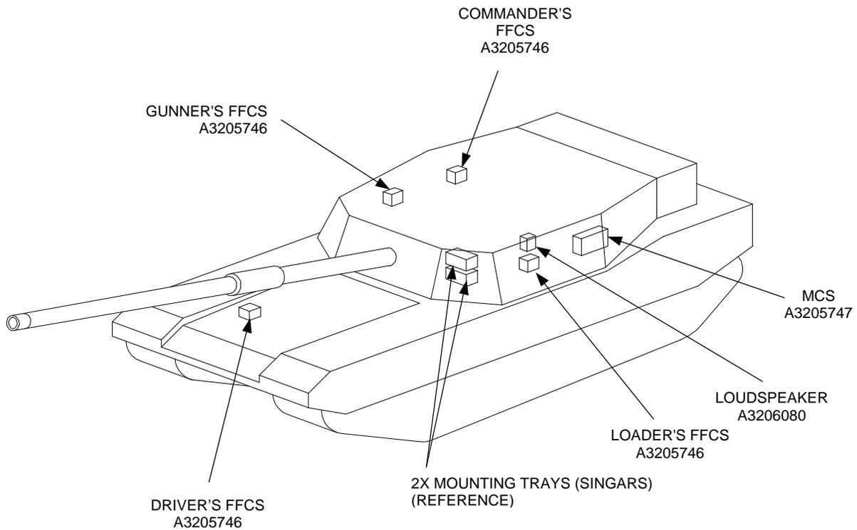
Figure 4-1. Equipment Location Diagram
