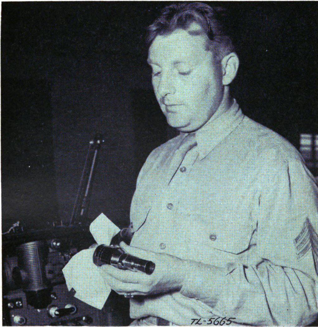
FIGURE 53.—Cleaning lens with tissue.
