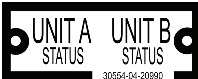
Figure 26. Plate, Status, Switch Box.
