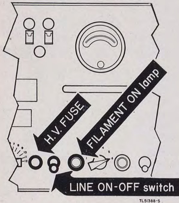
Figure 5. H. V. FUSE, FILAMENT ON lamp, and LINE ON-OFF switch, Radio Transmitter T-14(*)/.
