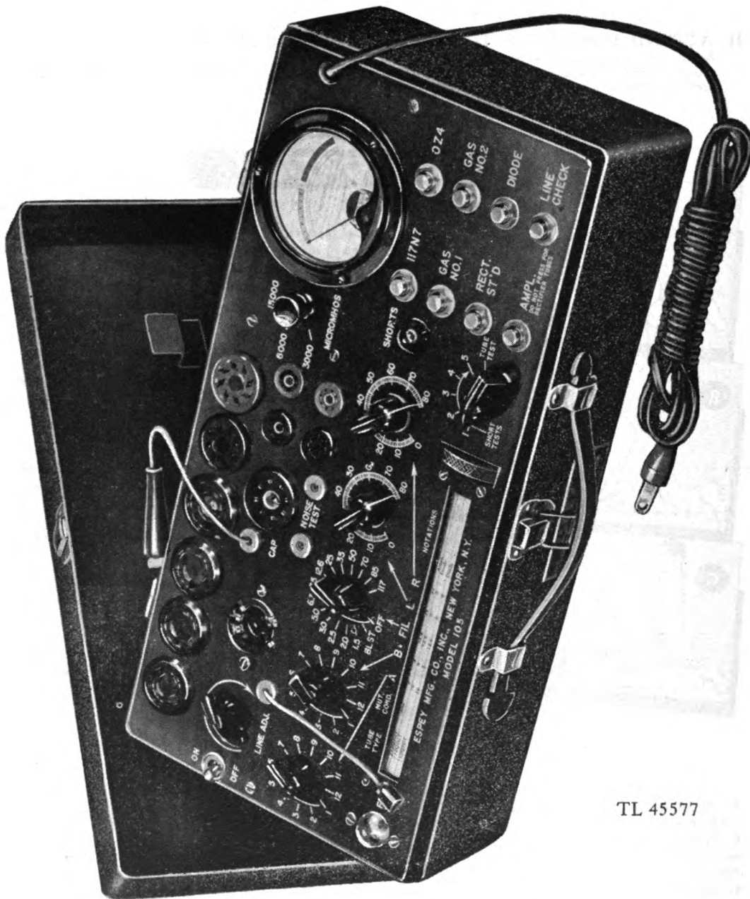
Frontispiece. Tube tester Espey model 105, with cover removed.
