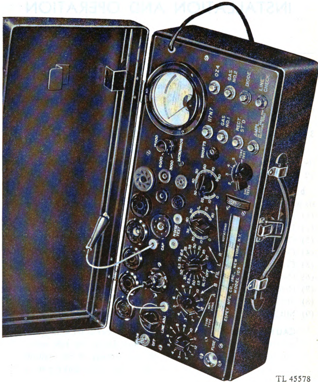
Figure 1. Tube tester showing acorn Tube VT-120 being tested.
