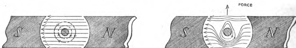
Figure 260. Action of a wire carrying current in a magnetic field. (The current shown is a stream of electrons coming out of the page.)
