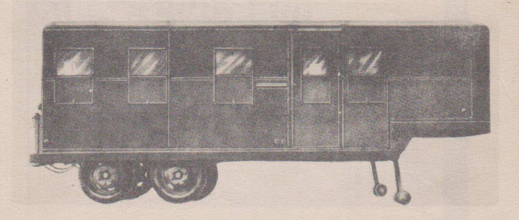
Figure 1—Semitrailer, 2-Ton Payload, 4-Ton Gross, 4-Wheel (4 st), Tandem Axle, Van, 1942-43 (Miller Model K-55)
