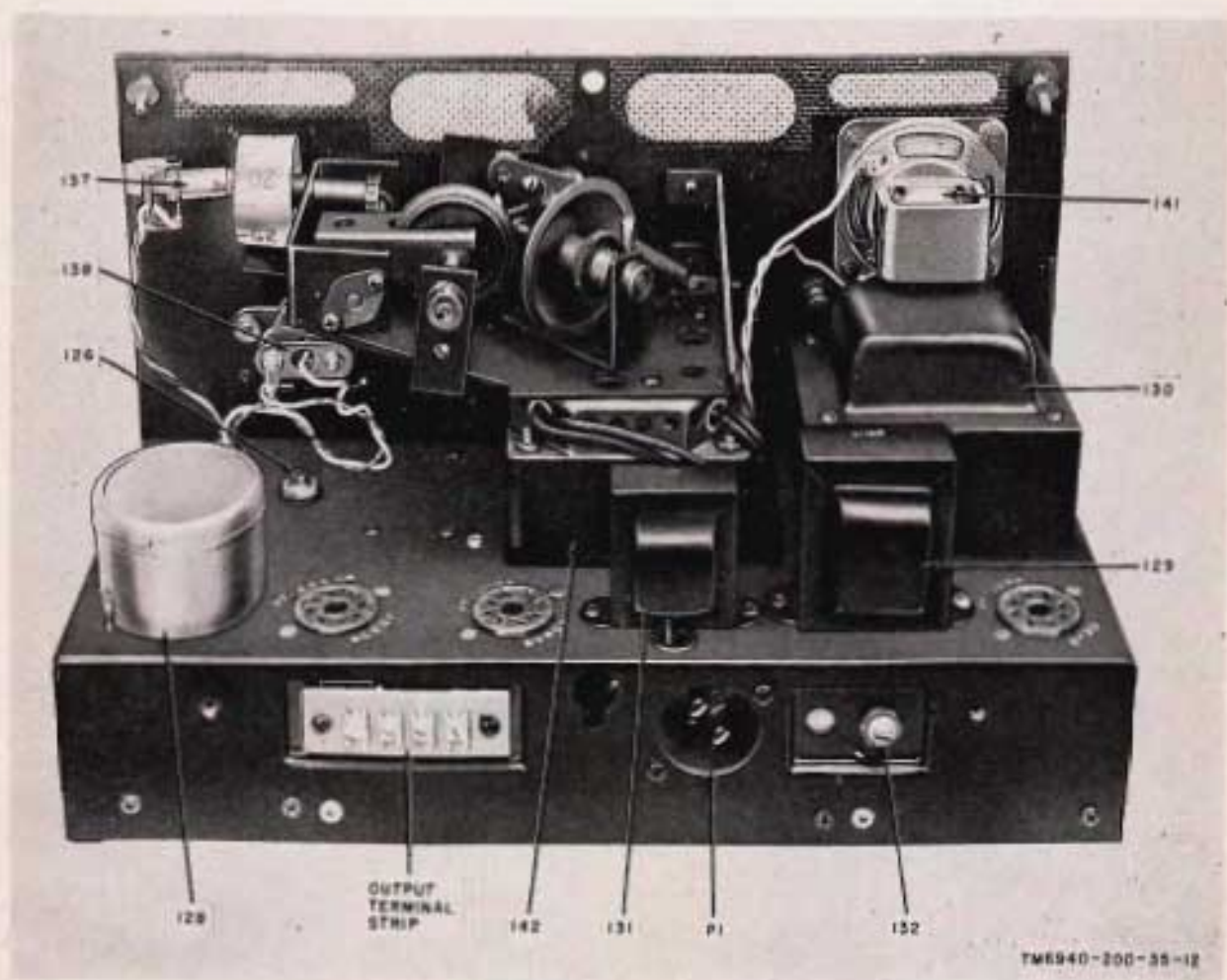
Figure 2. Keyer TG-34-A, location of parts, top view.
