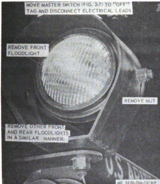
Figure 4-9. Floodlight assembly, removal and installation.
