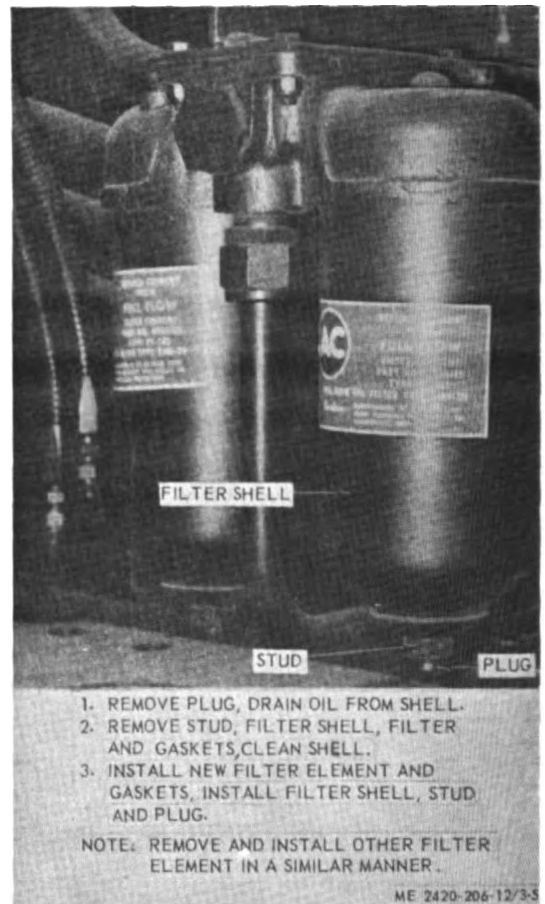
Figure 3-5. Transmission and torque converter, oil filter service.
