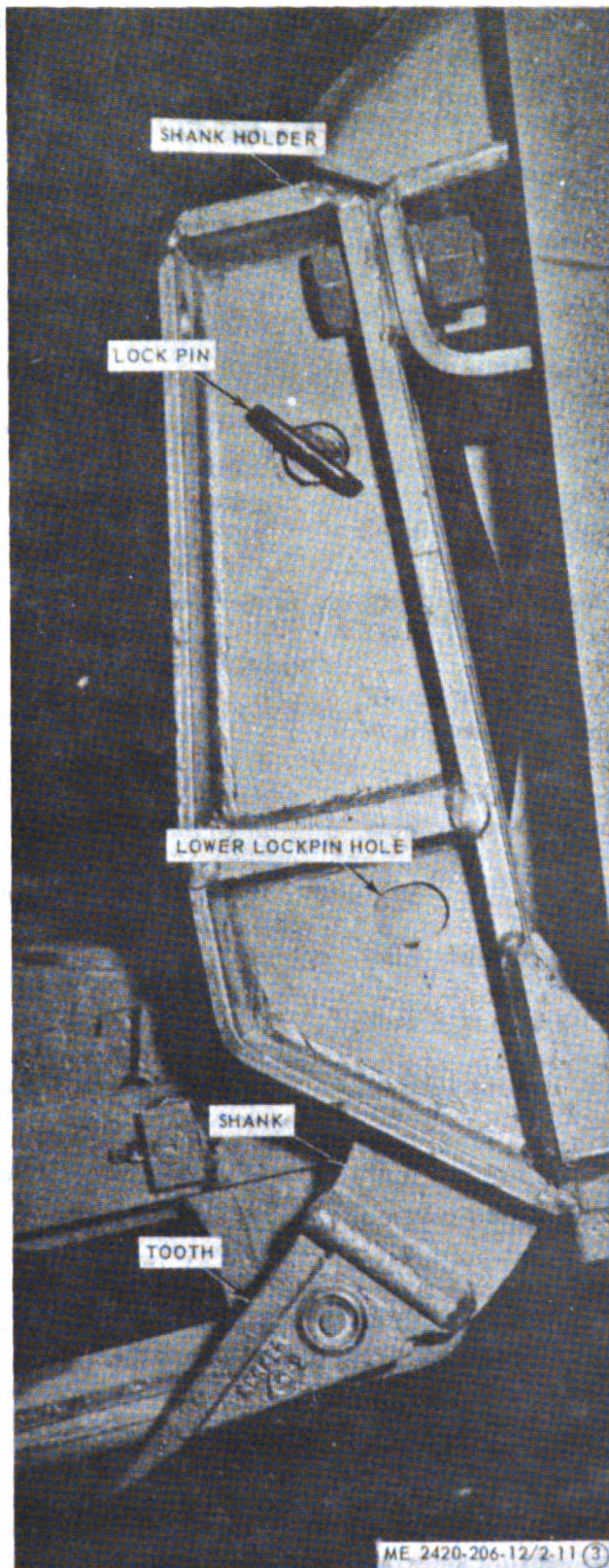
Figure 2-11. Bulldozer and scarifier operating instructions (sheet 3 of 3).
