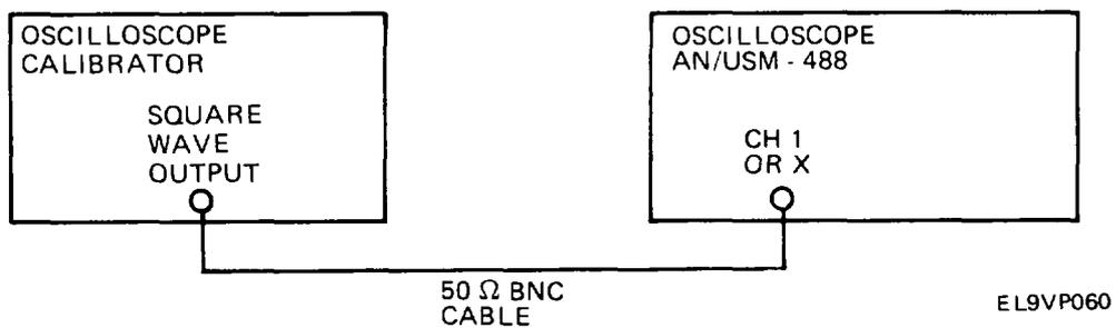
3. Set oscilloscope calibrator for 50 mV output signal.
