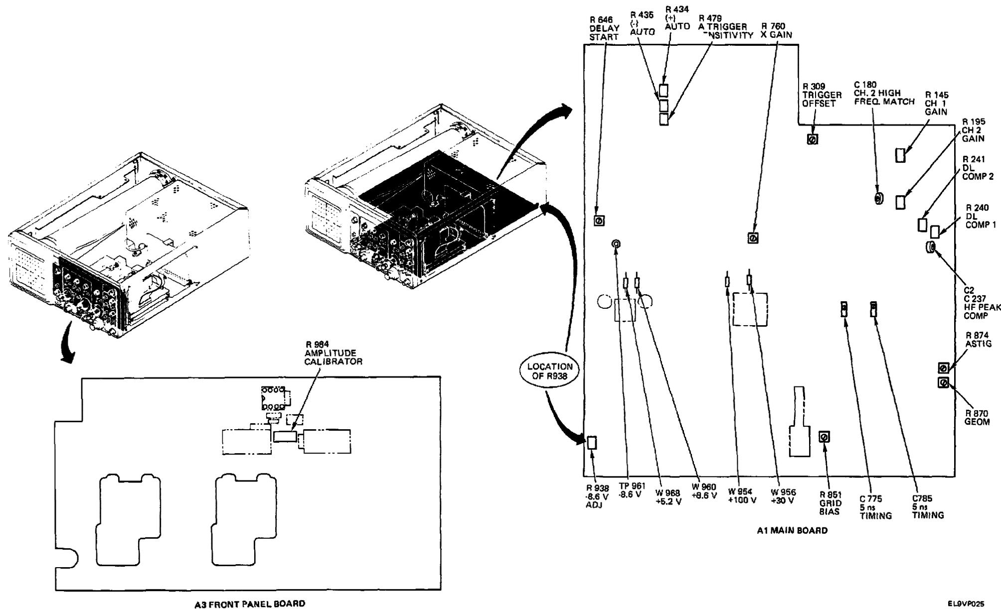
Figure FO-4. Adjustment Points (Sheet 2 of 2)
