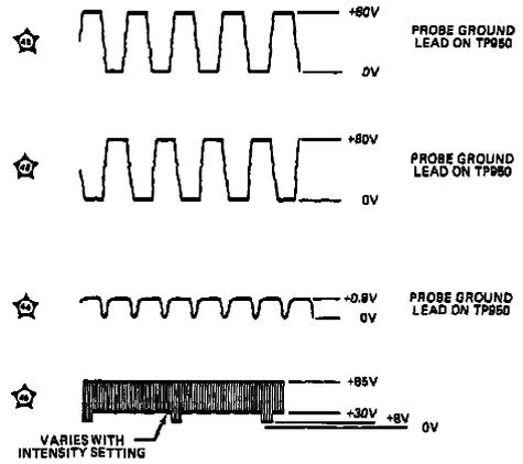
PREREGULATOR AND INVERTER VOLTAGES ARE REFERENCED TO TEST POINT NOTED ADJACENT TO THE VOLTAGE. POWER SUPPLY OUTPUT VOLTAGES ARE REFERENCED TO CHASSIS GROUND.
