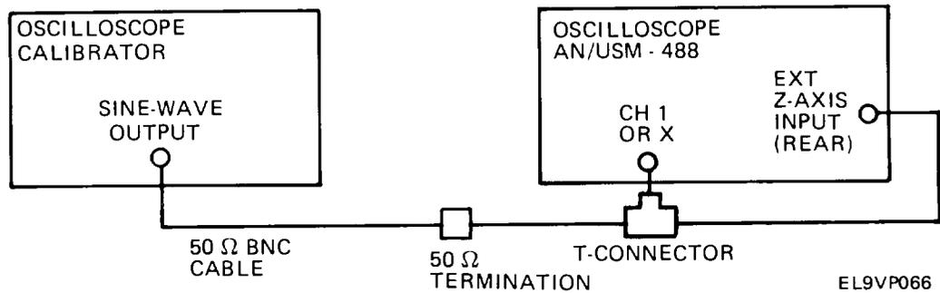
2. Set oscilloscope calibrator for 50 kHz, 5 V output.
