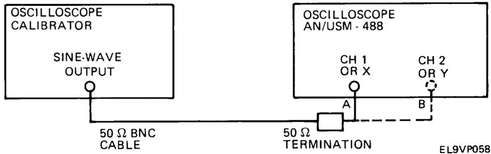
3. Set oscilloscope calibrator for 50 MHz, 5 V p-p output.
