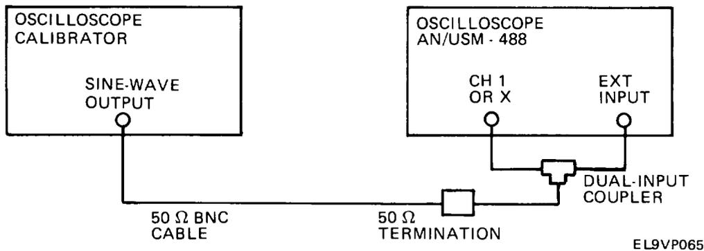
3. Set oscilloscope calibrator for 50 kHz, 6.4-division display.
