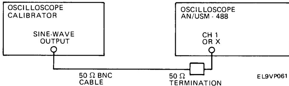
2. Set oscilloscope calibrator for 50 kHz, 5-division horizontal display.
