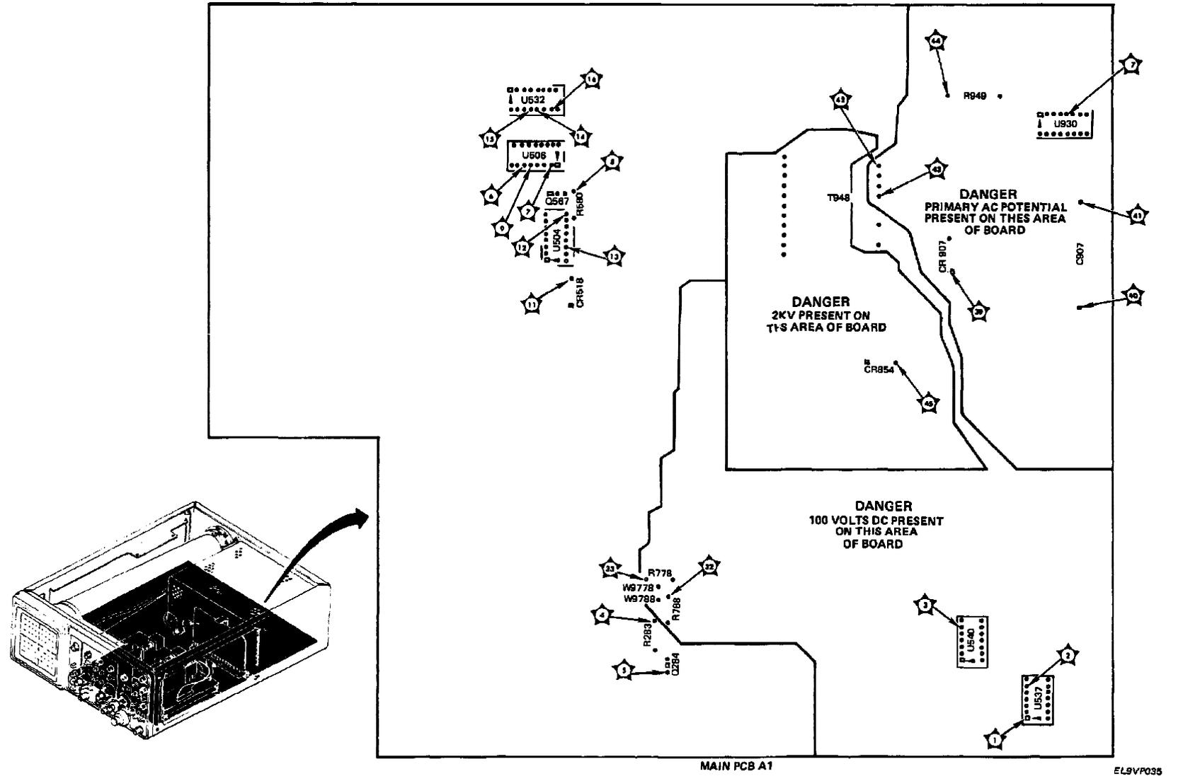
Figure FO-13. Waveform Test Point Locations
