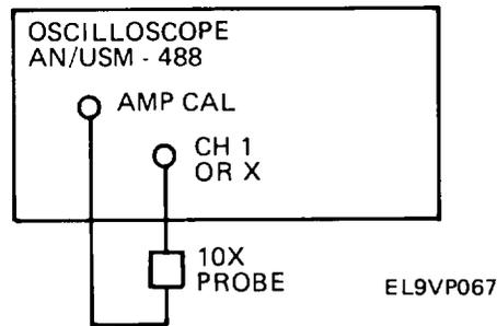
3. Adjust probe compensation for a flat-topped square-wave display.
