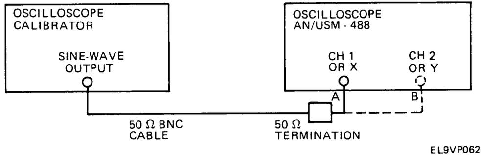
2. Set oscilloscope calibrator for 10 M Hz, 3.5-division amplitude display.
