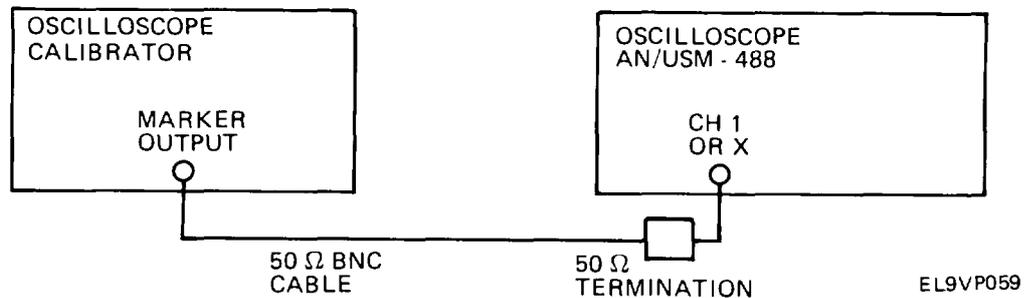
2. Set oscilloscope calibrator for 50 ns time marker output.
