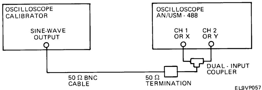
3. Set oscilloscope calibrator for 80 MHz, 6-division display.
