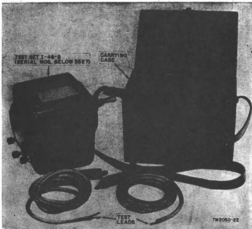
Figure 2. Test set I-48-B (serial numbers lower than 5527), carrying case, and test leads.
