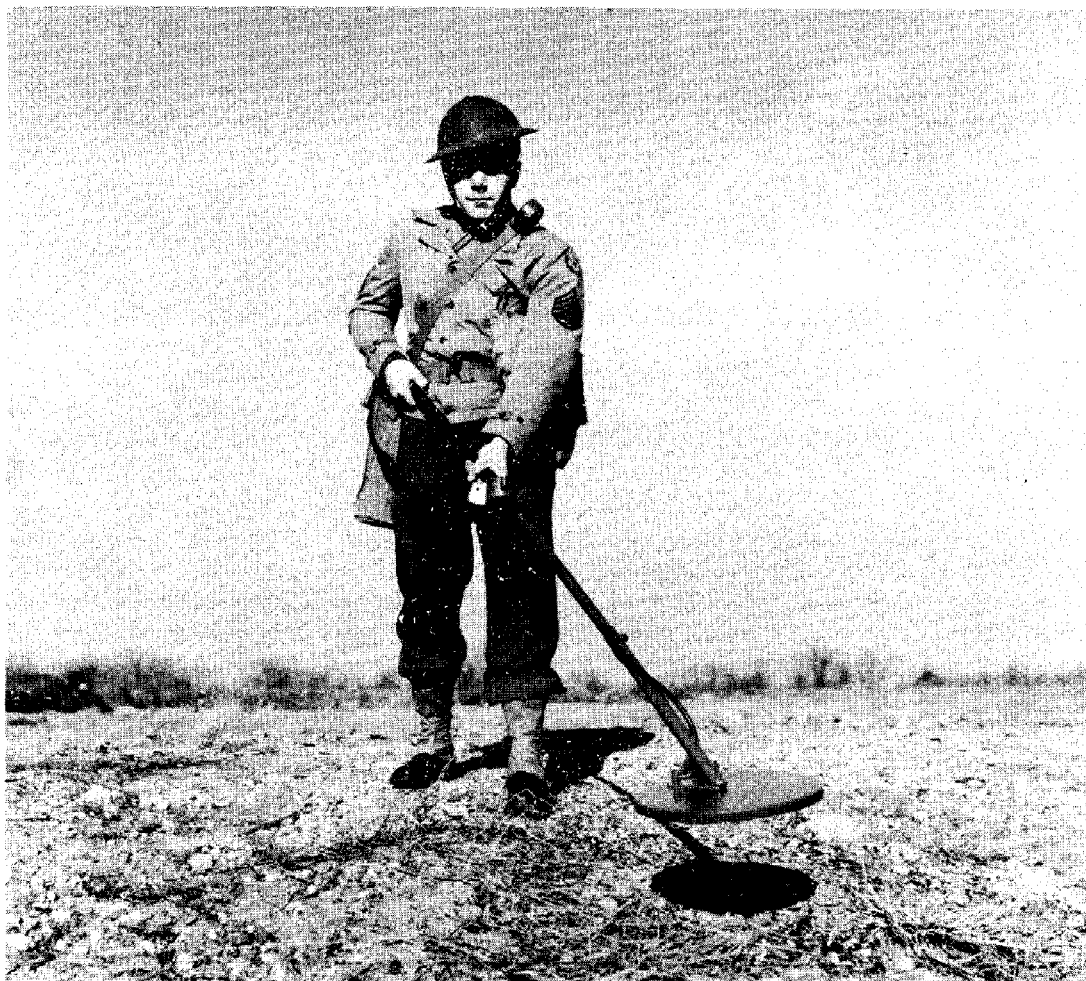
DETECTOR SET SCR-625-D PROVIDES BOTH AUDIBLE AND VISUAL INDICATIONS OF THE PRESENCE OF BURIED METALLIC MINES.
