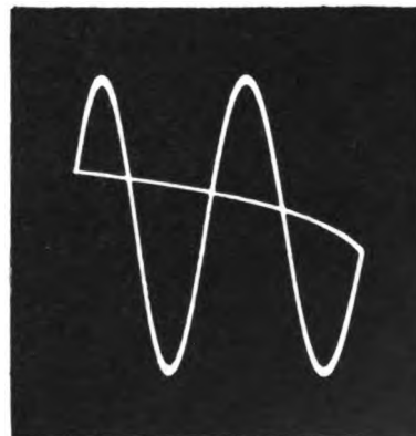
Figure 28. Oscilloscope pattern showing two cycles of a sine wave.
