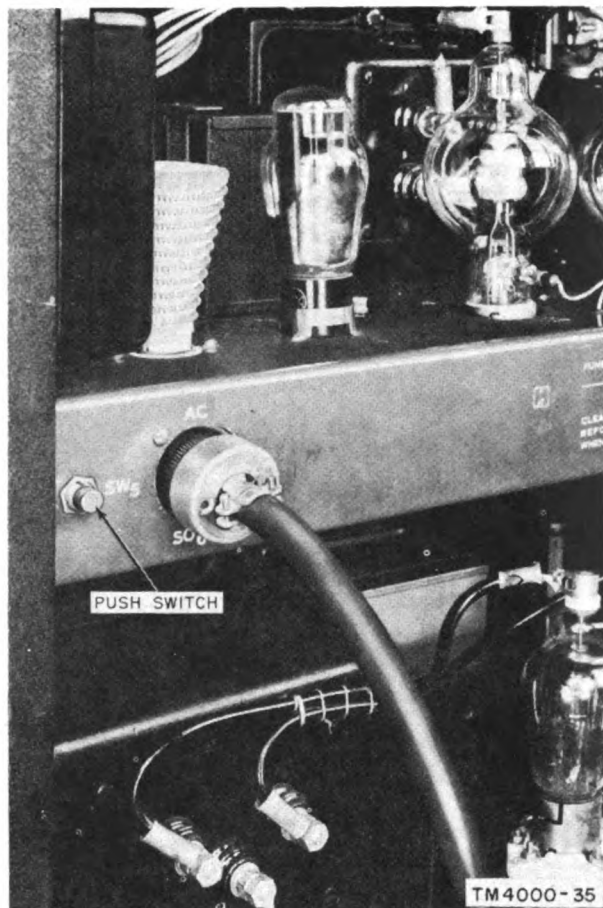
Figure 6. Example of a push-switch interlock.
