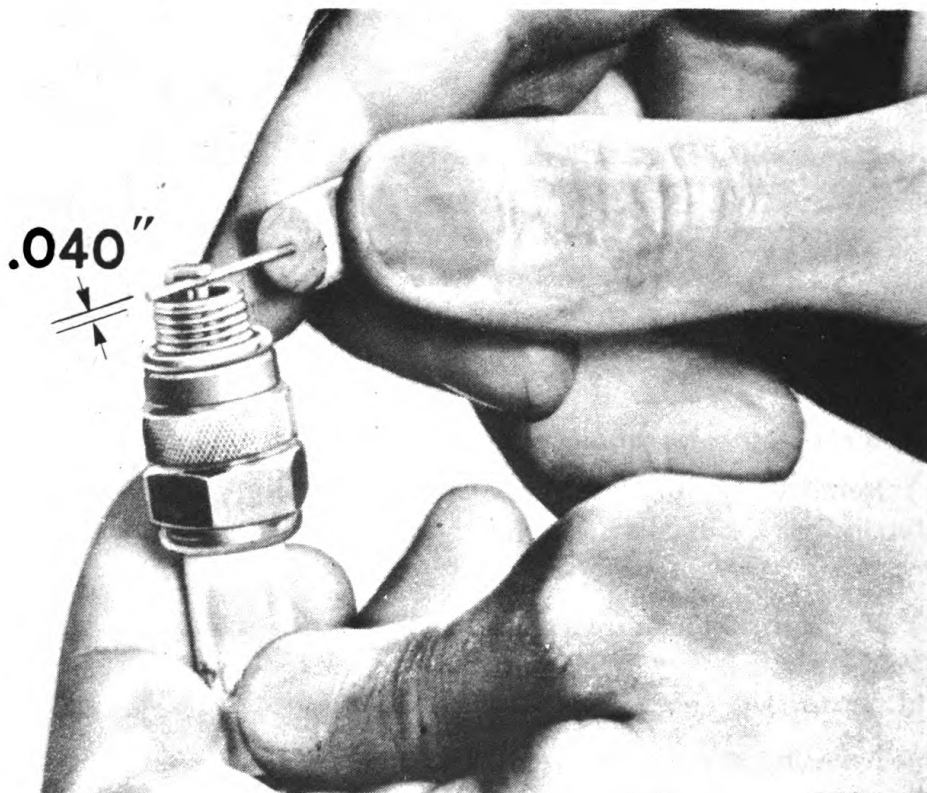
Figure 72—Setting Spark Plug Gap
