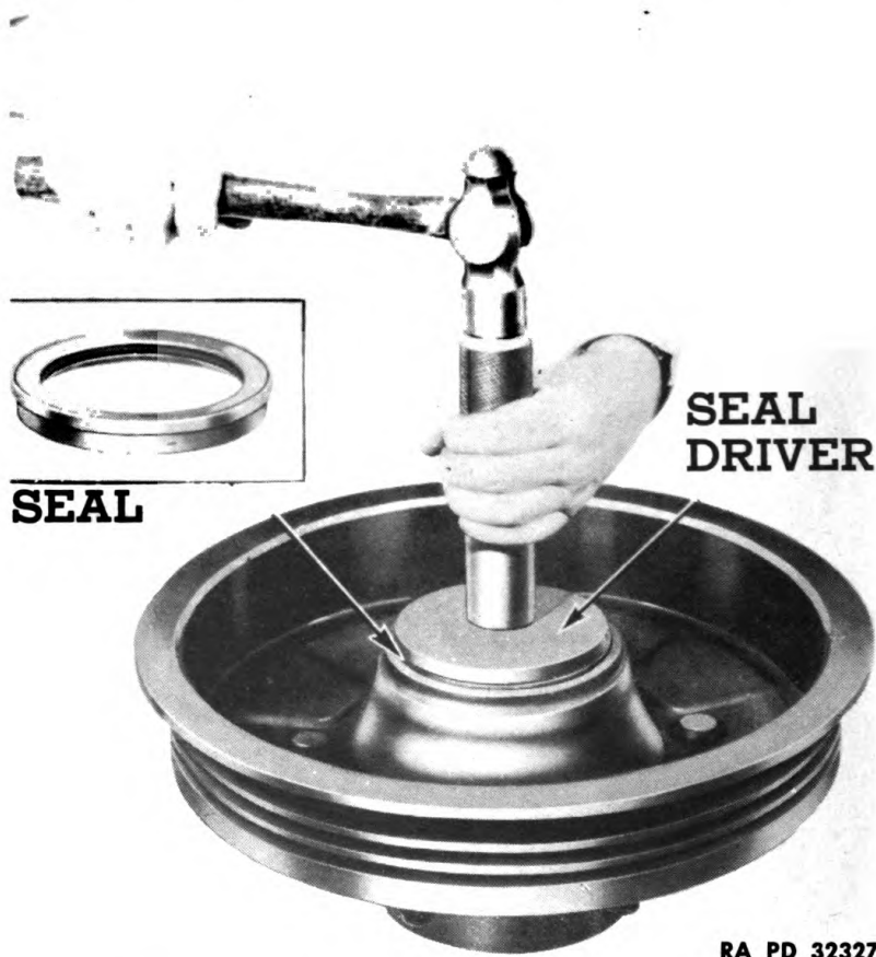
Figure 127—Replacing Inner Bearing Seal
