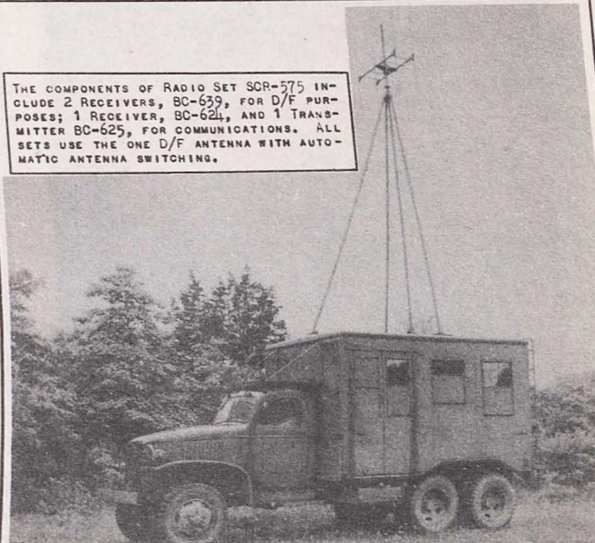
RADIO SET SCR-575 (RADIO DIRECTION FINDING STATION) ANTENNA EQUIPMENT RC-153 RAISED IN POSITION.
