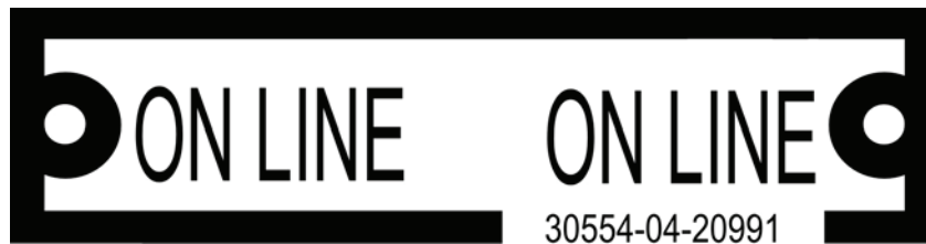
Figure 25. Plate, On Line, Switch Box.
