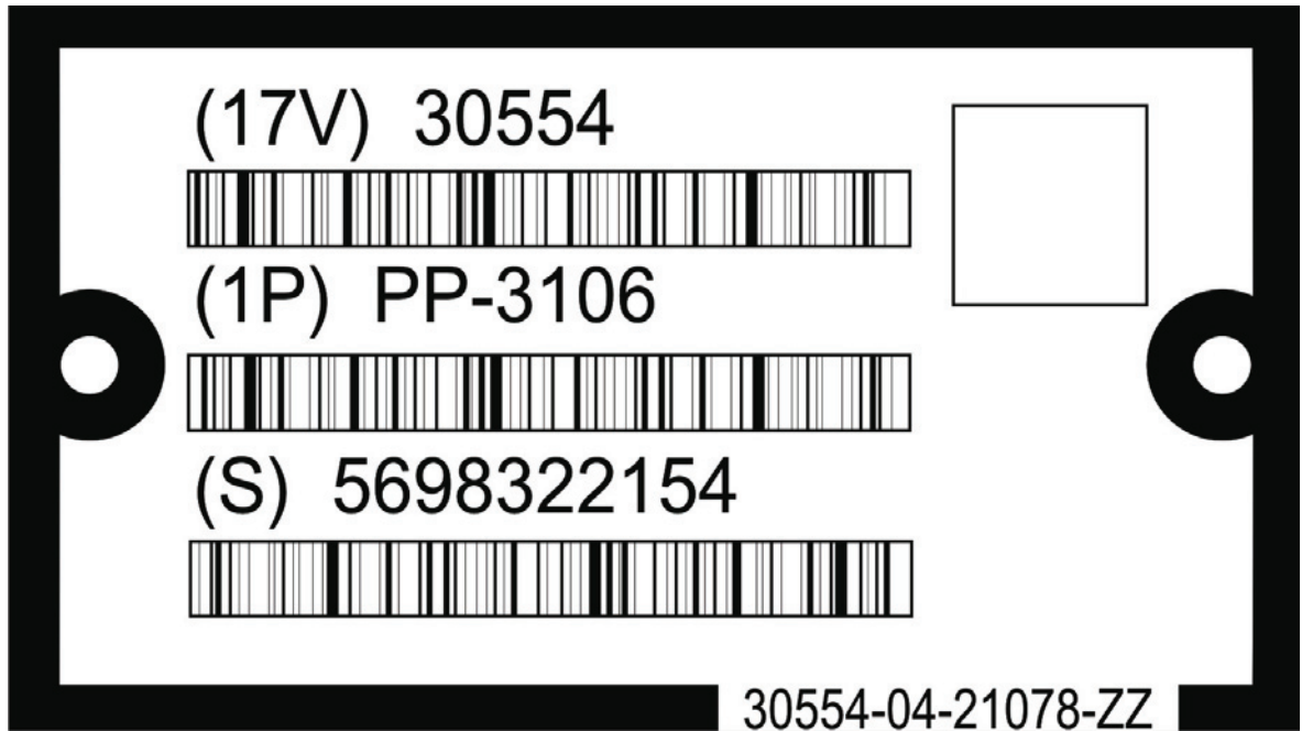
Figure 18. Plate, PP Identification (IUID), PP-3106 Unit A.
