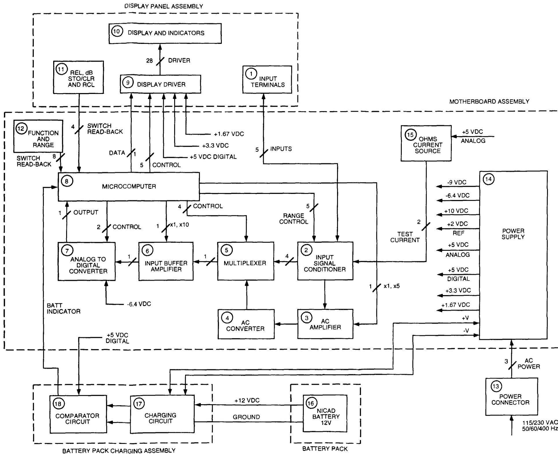
Figure FO-1. Digital Mutimeter AN/USM-486A
