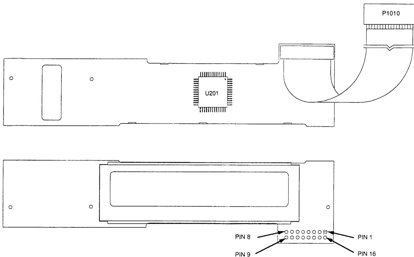
DISPLAY PANEL ASSEMBLY COMPONENT LOCATOR
