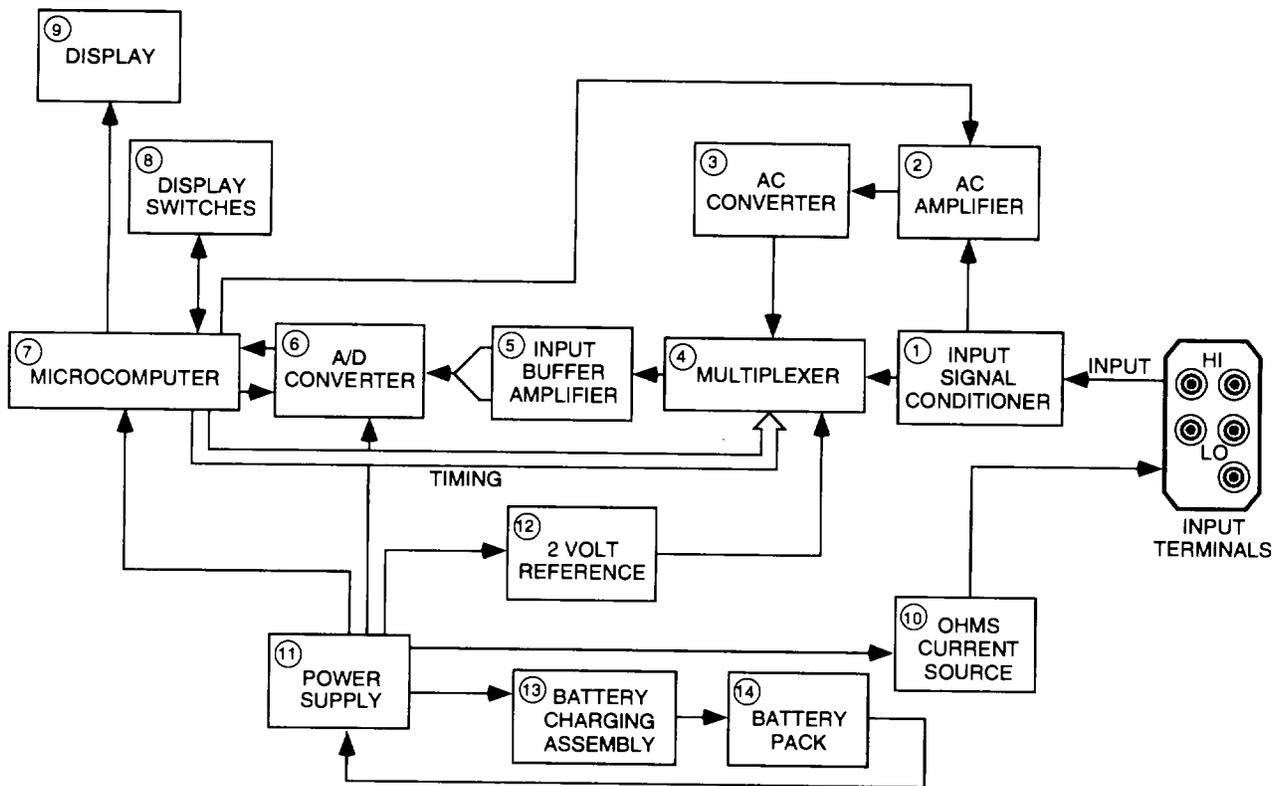
Figure 1-2. Digital Multimeter AN/USM-486A Functional Block Diagram
