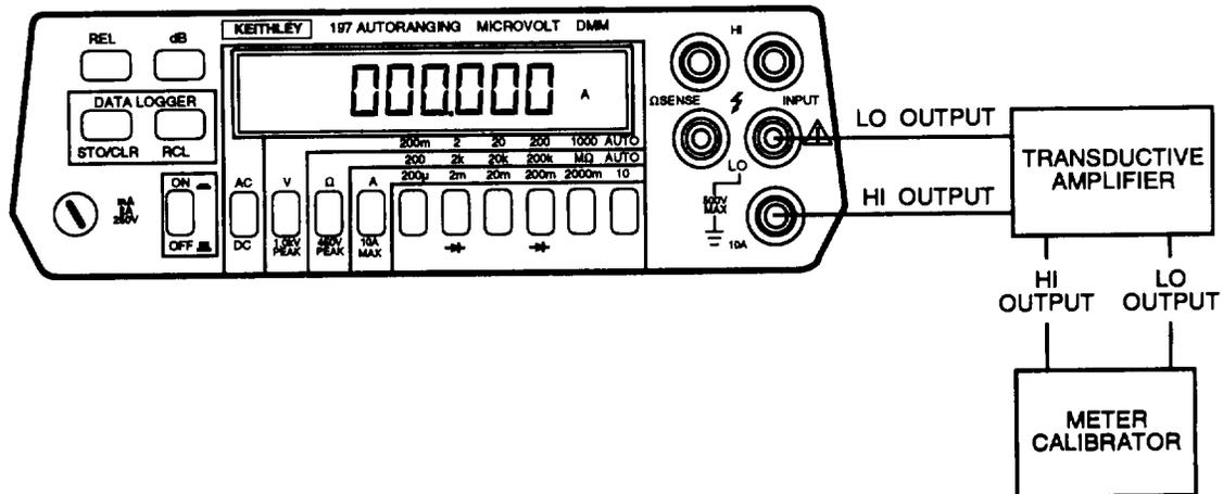
5. Set meter calibrator to the applied ac current (10 A) and frequencies (20 Hz through 10 kHz) as shown below. Verify that the display reads within the specified limits for each current applied. If the display does not read within all specified limits, perform ac voltage adjustment (para 5-25).
