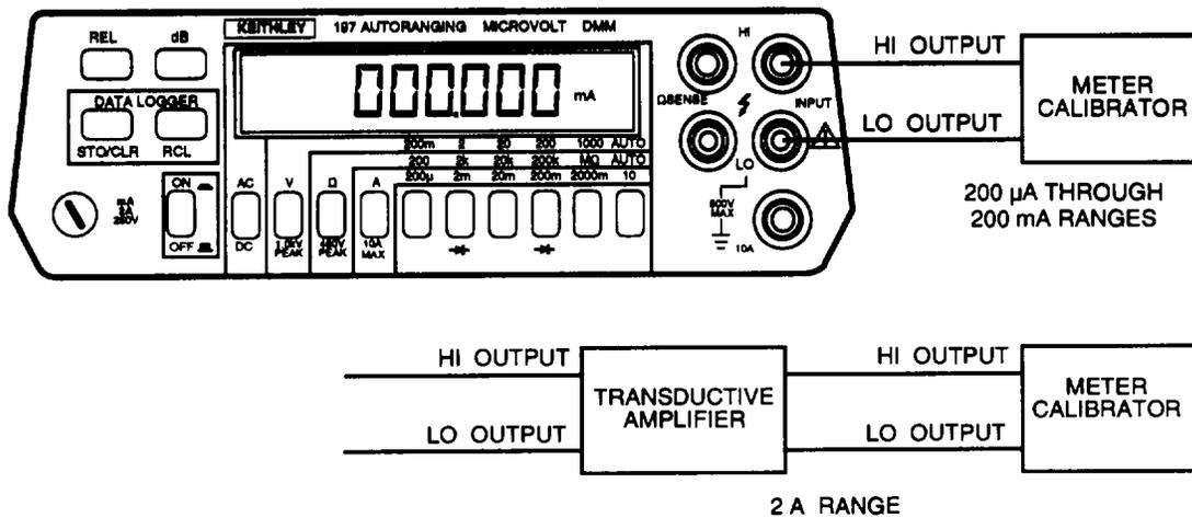
3. Set meter calibrator to each applied ac current (190  $\mu$ A through 1900 mA) and frequencies (20 Hz through 20 kHz) as shown below. Verify that the display reads within the specified limits for each current applied. If the display does not read within all specified limits, refer to Troubleshooting (Chapter 5, Section IV).
