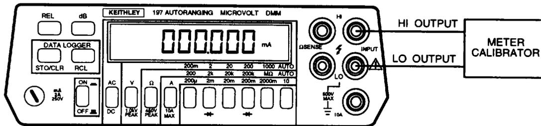
3. Set meter calibrator to 00.000 (short) and zero multimeter [enable REL mode (para 2-22)]. Verify display reads 000.000 $\mu$  A.
