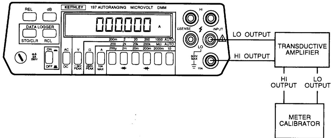
6. Set multimeter for each range and apply dc current as shown below. Verify that the display reads within the specified limits for each current applied. If the display does not read within all specified limits, refer to Troubleshooting (Chapter 5, Section IV).
