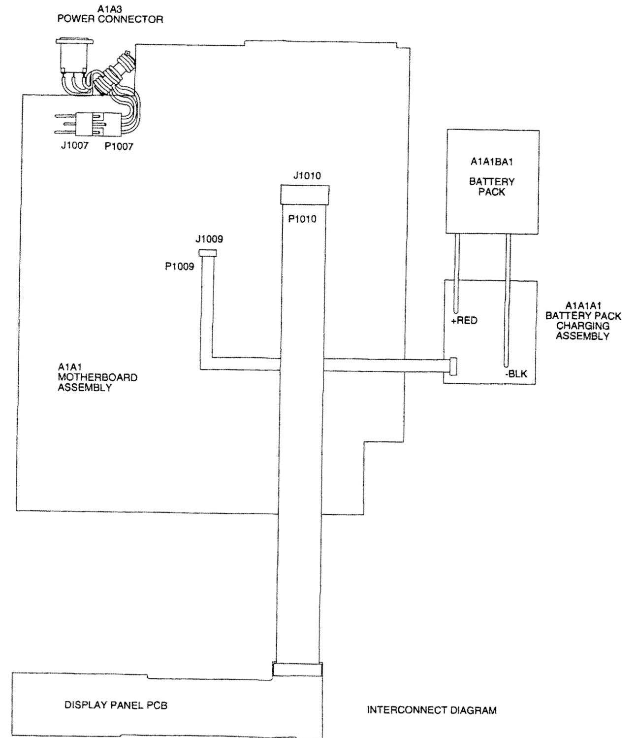
Figure FO-3. Overall Locator and Interconnect Diagrams
