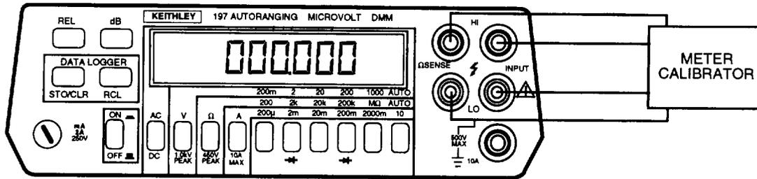
3. Set meter calibrator to 000.000 (short) and zero multimeter [enable REL mode (para 2-22)]. Verify display reads 000.000Ω.
