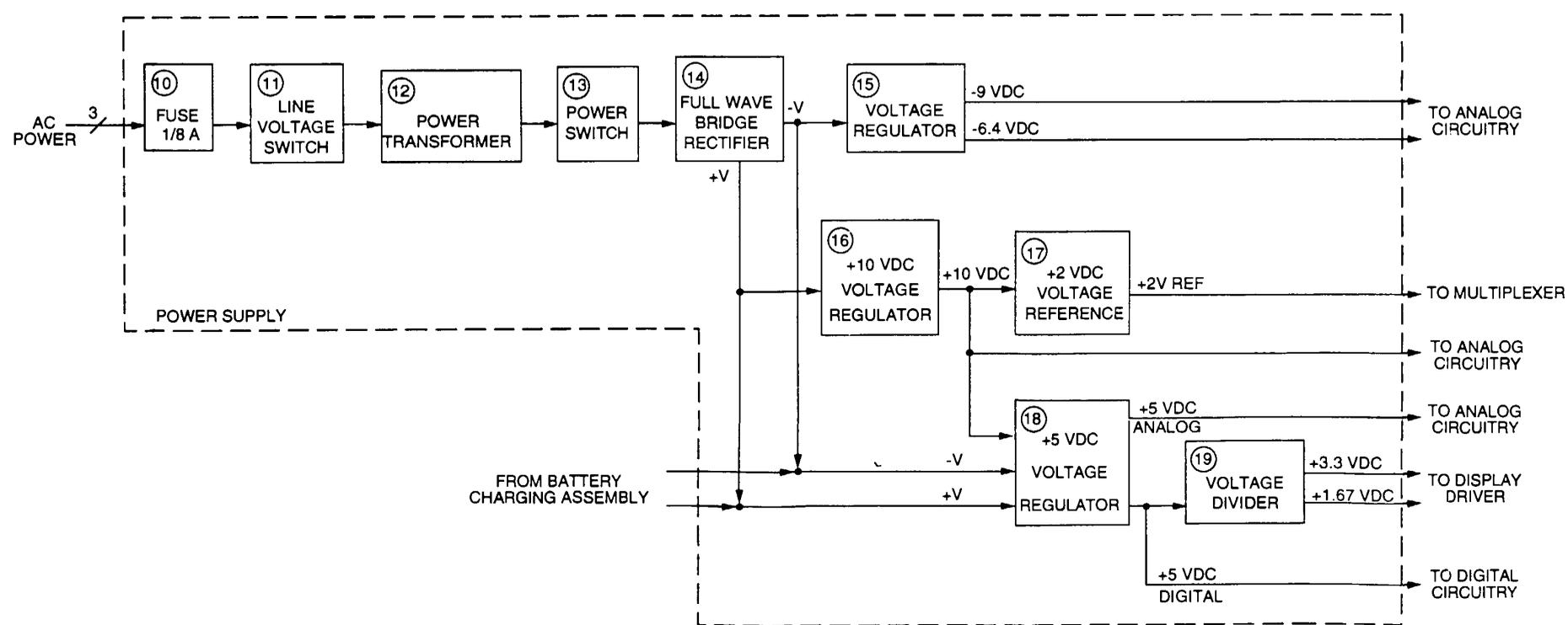
Figure FO-2. Motherboard Functional Block Diagram
