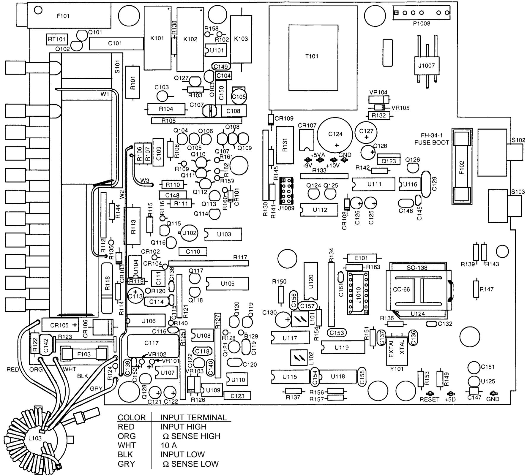
Figure FO-5. Motherboard Assembly Component Locator
