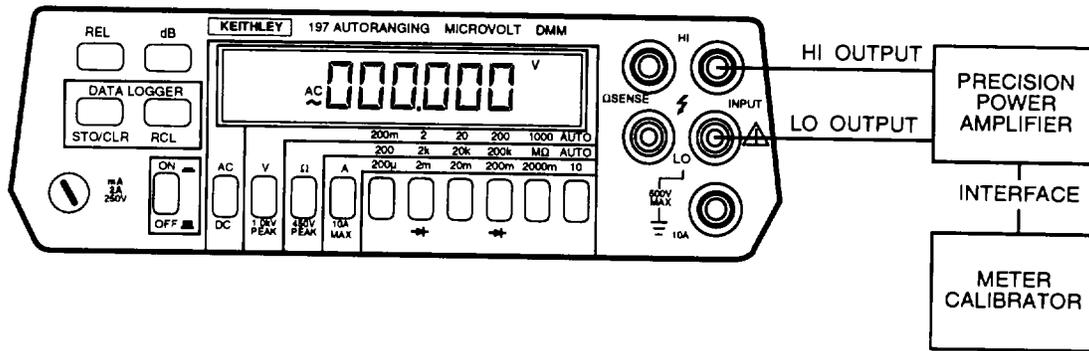
3. Apply voltage of 500.00 Vac at 500 Hz with meter calibrator. Set this as multimeter's zero [enable REL mode (para 2-22)].
