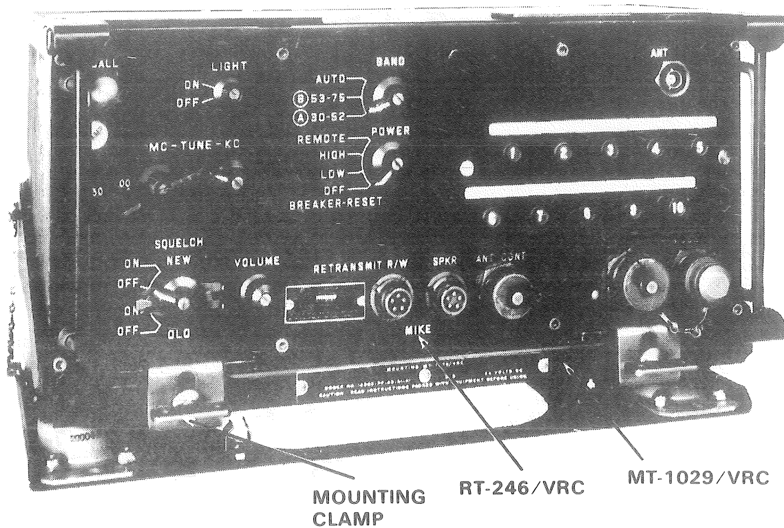
Figure 3. Receiver-Transmitter Radio RT-246/VRC installed on Mounting MT-1029/VRC.
